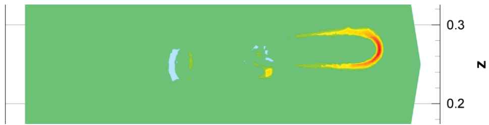
Figure 6.30: Net charge density at times t_1 = 1.89 \cdot 10^{-8} s, isolines in a cut plane y = 0.25
