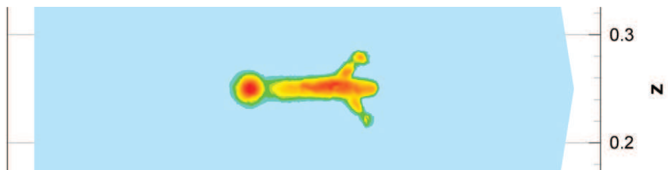
Figure 6.86: Electron density at times t_1 = 1.47 \cdot 10^{-8} s, isolines in a cut plane y = 0.25
