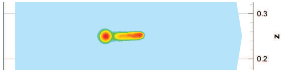
Figure 6.37: Electron density at times t_1 = 1.26 \cdot 10^{-8} s, isolines in a cut plane y = 0.25
