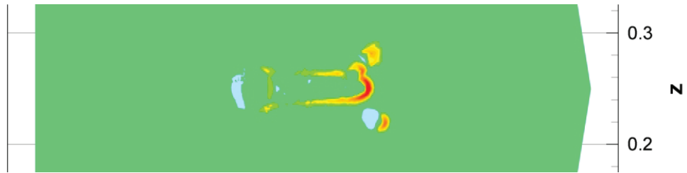
Figure 6.97: Net charge density at times t_1 = 1.36 \cdot 10^{-8} s, isolines in a cut plane y = 0.25
