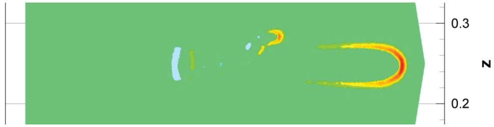
Figure 6.51: Net charge density at times t_1 = 1.89 \cdot 10^{-8} s, isolines in a cut plane y = 0.25
