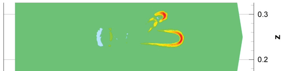
Figure 6.74: Net charge density at times t_1 = 1.68 \cdot 10^{-8} s, isolines in a cut plane y = 0.25
