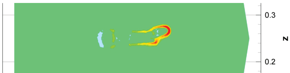
Figure 6.28: Net charge density at times t_1 = 1.47 \cdot 10^{-8} s, isolines in a cut plane y = 0.25
