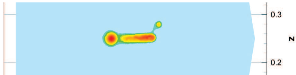
Figure 6.59: Electron density at times t_1 = 1.31 \cdot 10^{-8} s, isolines in a cut plane y = 0.25
