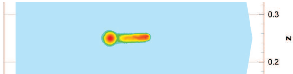
Figure 6.58: Electron density at times t_1 = 1.26 \cdot 10^{-8} s, isolines in a cut plane y = 0.25
