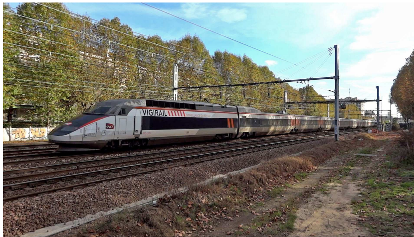
Figure 1.2: High-speed train IRIS 320 for the tracks inspection.
