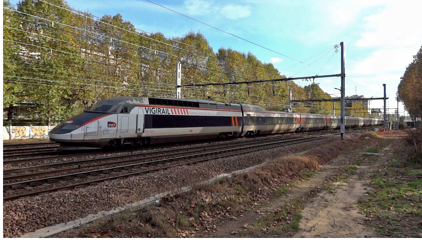
Figure 1.2: High-speed train IRIS 320 for the tracks inspection.
