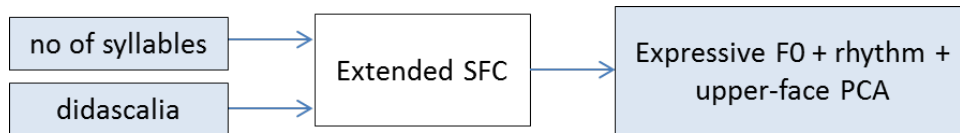
Figure 5.7: Prosody generation with model-based technique. The SFC model uses phonotactic information and didascalia in order to generate prosodic stylized contours.
