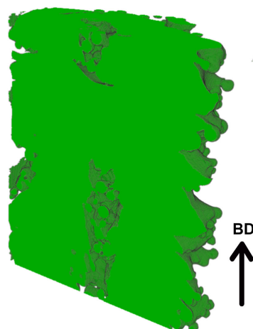
Figure 9.2 longitudinal cut of a vertical 1.5 mm diameter strut manufactured with the "Net" theme. Large porosity is observed in the center of the strut.
