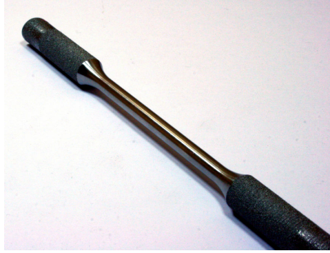
Figure 5.7 5 mm diameter sample machined from an as-built sample with a 6 mm diameter.
