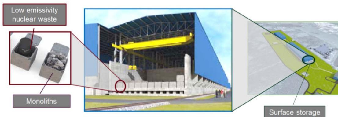
**Figure 1.1 Surface disposal solution for low emissivity nuclear waste: cAt project in Dessel, Belgium (ONDRAF/NIRAS, 2010)**
