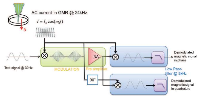
Figure 3.24: Modulation/demodulation frequency principle.
