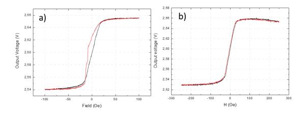
Figure 3.29: a)R(H) response of a yoke with 200 µA feeding current, presenting some jumps due to magnetic domain switching. b) R(H) response of a yoke for a 200 µA feeding current and with a low-pass at 30 Hz.
