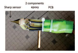
Figure 3.17: Sharp probe for slice recordings. The sensor is fixed on a PCB and the contact pads are wire-bonded and isolated by a 2-components epoxy. The brass rod on the back of the PCB is later fixed to a micromanipulator for precise positioning on the sensor when inserted in the tissues.
