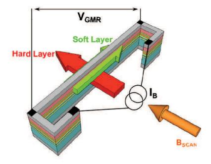
Figure 2.8: Four-points contact measurement of a yoke.  $B_{scan}$  is the external applied field. The current  $I_B$  is sent at the edges of the yoke and the output voltage  $V_{GMR}$  is measured in the linear region of the yoke. Adapted from [64]
