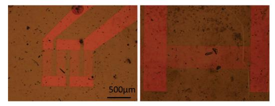
Figure 4.6: Planar probes used for muscle recordings. Meander (left) and a segment (S1) probes.
