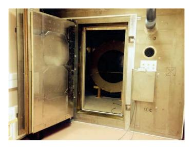
Figure 3.19: Magnetically shielded room at SPEC/CEA Saclay.
