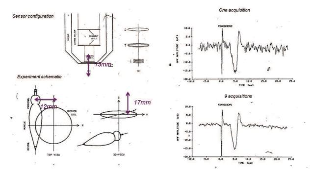
Figure 4.3: Summary of the main result obtained in ref [13]. The signal is measured by a SQUIDs at 4 K placed at 17 mm from a muscle of a Leopard frog.
