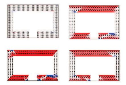
Figure 2.6: Evolution of the magnetization in a yoke for four external applied magnetic fields (-10 mT, -1 mT, 0, 1 mT). Arrows indicate the direction of the planar magnetization while colours indicate the momentum out of plane (typically 1°). This configuration is calculated by a micromagnetic software (*oommf*). Adapted from [63]
