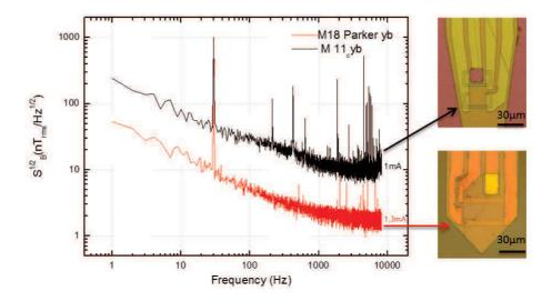
Figure 3.33:  $S_B$  as function of frequency for sharp model 1 (#M11) with 2 yokes (3x30 µm) and sharp model 4 (#M18Parker) with 2 larger yokes (4x40 µm).
