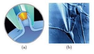
Figure 1.6: Schematic representation of intracellular recordings. (a) Patch-clamp principle (cell-attached technique): a thin pipette (1 µm diameter), isolates an ionic channel to perform intracellular recordings. (b) Microscopy image of patch-clamping. Adapted from [26].
