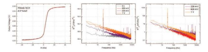
Figure 5.6: Sharp magnetrode characteristics. Left: R(H) response of #M24 Monk probe with a resistance  $R_0 = 440 \Omega$ , a MR ratio of 6 % and a sensitivity near zero field of 4.9 %/mT. One can note the linear response of the GMR. Middle: noise voltage spectrum as function of the frequency. Right: field equivalent noise as function of frequency.
