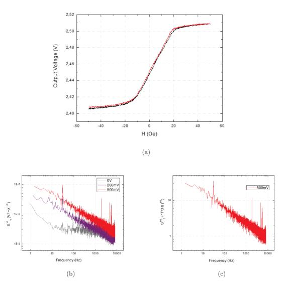
Figure 4.23: Sharp probe calibration (#M11G). a) R(H) on 3x30 µm yoke. The probe exhibits a linear, non-hysteretic response with a MR of 4.48 % and a sensitivity at zero field of 1.2 %/mT. b) Voltage noise as function of frequency. c) Field equivalent noise as function of frequency
