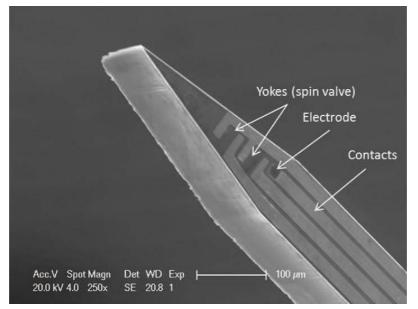
(a) SEM picture of a spin valve deposited on a 150  $\mu m$  silicon substrate and containing two yokes (30x3  $\mu m)$  with a gold pad electrode.
