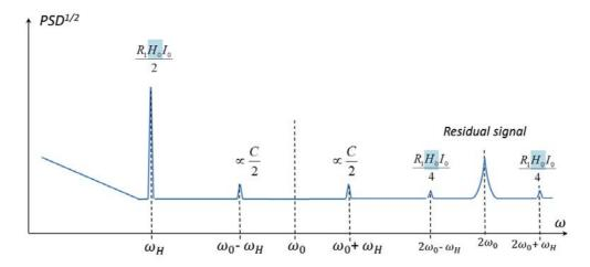
Figure 3.23: PSD after the demodulation step.
