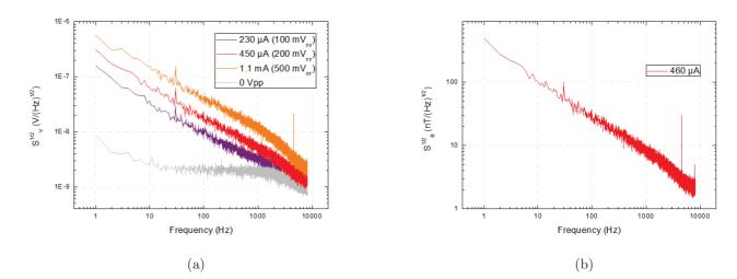
Figure 3.31: DC noise measurements of the sharp magnetrode #M8a (30x3 µm yoke- 440  $\Omega$ ) with DC noise measurement. The frequency bandwidth is 0.3 - 3 k Hz. An AC signal test at 30 Hz produced a magnetic field of 100 nT<sub>rms</sub> that is measured by the sensor (seen in the PSD). Noise measurements were achieved in the shielded room. a) PSD of the voltage noise for several bias currents. b) Field equivalent noise (detectivity).
