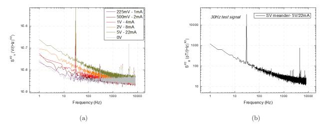
Figure 3.28: Noise measurements on meander planar probe with DC setup. A test signal of 850 nT<sub>RMS</sub> at 30 Hz is sent to calibrate the sensor. a) S<sub>V</sub> corresponds to the PSD of the voltage noise as a function of frequency for various bias voltages. b) Corresponding field equivalent noise S<sub>T</sub> expressed in  $pT/\sqrt{Hz}$  as a function of frequency.
