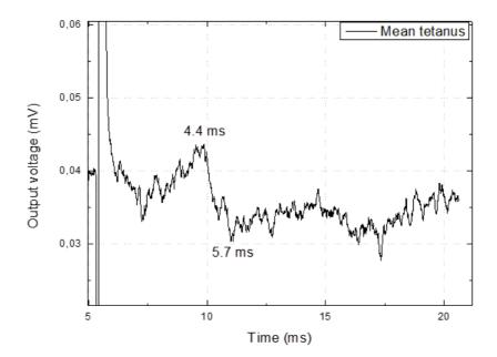
Figure 4.13: Output signal of the probe when the muscle is under tetanus. Very fast electrical stimulations are applied through the nerve, leading to a full contraction of the muscle, but where the AP is still propagating. In these recordings, the noise level recorded is quite high and the magnetic AP is detected because of its specific timing.
