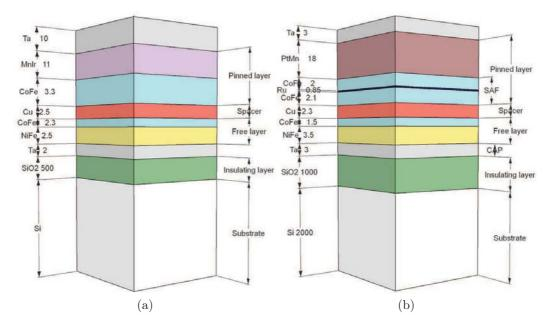
Figure 3.4: Spin valve stacks used for magnetrode process a) SV stack used for the first set of sharp magnetrode process (from INESC-MN) b) SV stack used for the second and third set of both sharp and planar magnetrode process (from AllegroMicrosystems). Thicknesses are given in nm.
