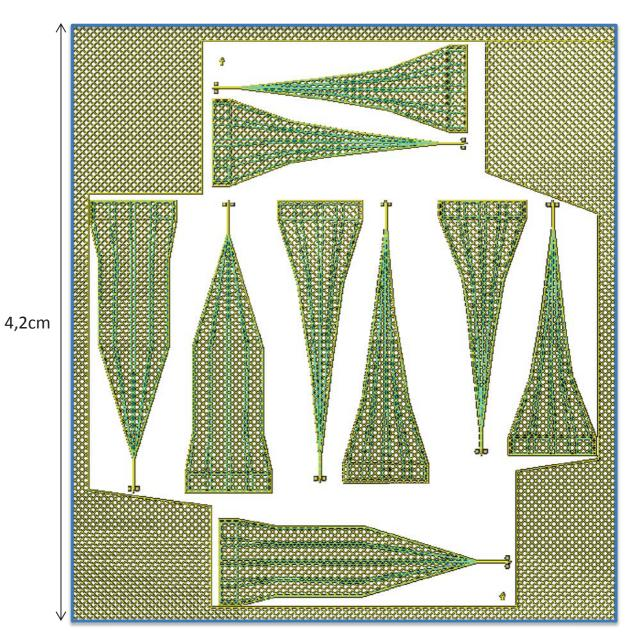
Two yokes 30x3 µm + electrode (*In vivo & in vitro*)
