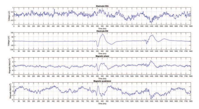
Figure 5.10: Same recordings channels than on Figure 5.8with longer stimulation (500 ms). Note the separation in time between the peaks at the onset (850 ms) and at the offset (1350 ms) because of the longer light exposure. The magnetic phase output is well correlated with the tungsten electrode, and the quadrature exhibits also a small signal (2 nT compared to 10 nT in the phase output).
