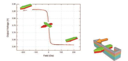
Figure 2.5: A typical R(H) curve of a sharp magnetrode (#M11g). GMR is patterned as a yoke shape contacted by two points. The resistance  $R_0$  is 250  $\Omega$  with a MR ratio of 4.48 % and a sensitivity of 1.2 %/mT. The red arrow does represent the hard layer while green arrow the free layer of the yoke. The external magnetic field applied (orange arrow) coming from a current source is parallel to the hard layer.
