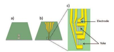
Figure 3.7: Sample after contact deposition. a) sample after GMR etching b) sample after contact deposition, previously lithographied as explained in 3.1.1.3; the resist is spinned and exposed where contact pattern is defined c) a zoom-in of the tip with two yoke sensors and an electrode point contact to measure the electric potential within tissues (in this exemple the electrode is made out of Ti/Au, in the same deposition step as the contacts).
