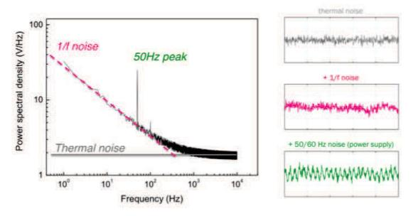
Figure 2.9: Voltage PSD as function of frequency.
