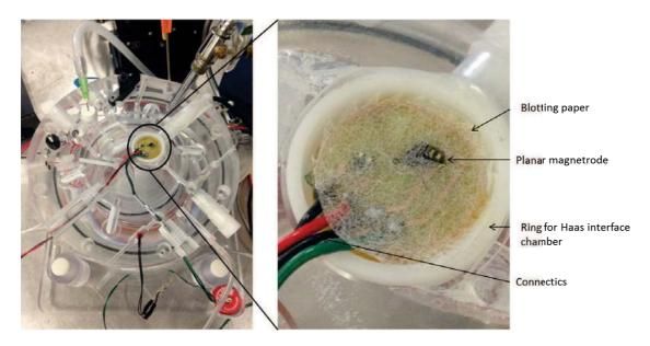
Figure 4.22: Planar sensor for slice setup. Left: full view of the sensor mounted on the interface chamber at UNIC-CNRS. Right: close-up view of the sensor in the chamber.
