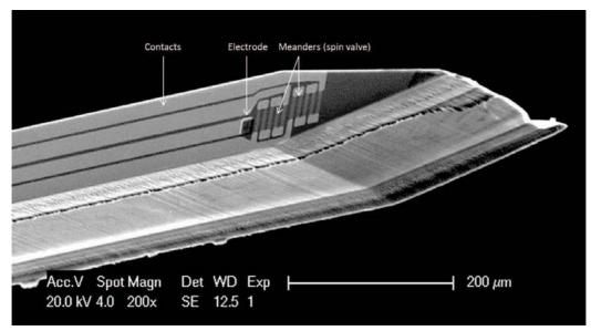
(b) Spin valve deposited on a 200  $\mu m$  silicon substrate
