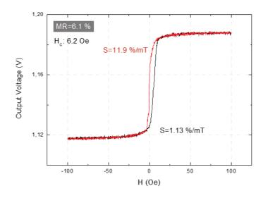
Figure 3.26: R(H) of the sharp probe (#Peterson2 *R15*). The current injected in the GMR is 200 µA with a low-pass at 30 Hz. Note that the sensitivity at zero field is greatly different on the black curve and on the red curve at 0 field, because of the coercive field (6.2 Oe).
