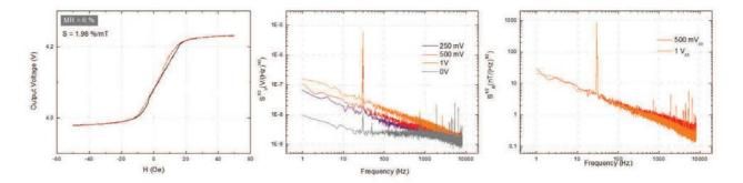
Figure 5.5: Sharp magnetrode characteristics. Left: R(H) response of #M19Evans probe with a resistance  $R_0 = 820 \ \Omega$ , a MR ratio of 6 % and a sensitivity near zero field of 1.9 %/mT. One can note the linear response of the GMR. Middle: Noise voltage spectrum as function of the frequency. Right: Field equivalent noise as function of frequency.
