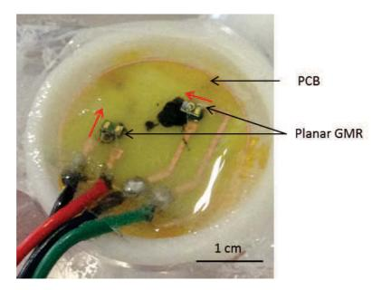
Figure 3.14: Planar magnetrode for slice recordings.
