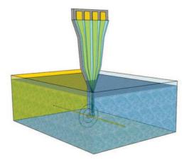
Figure 3.34: Phantom wire setup. A sharp magnetrode is inserted in a box filled with a conductive solution (ACSF). A signal at 30 Hz is sent into a thin wire and produce a small magnetic field detected by the probe.
