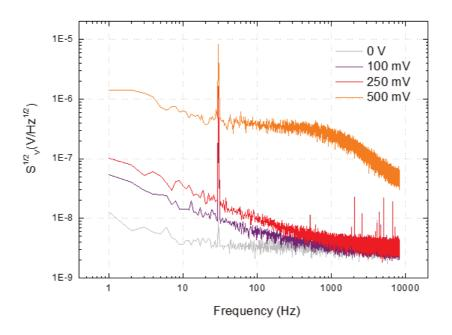
Figure 2.10: Voltage PSD as function of frequency at different voltages for a sharp magnetrode (cf chapter 3) patterned as a yoke shape ( $4x40 \mu m$ ). Note the presence of magnetic RTN at 500 mV bias voltage in the GMR.
