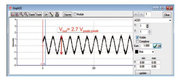
Figure 3.25: Screen shot of acquisition system while applying a test signal of 850 nT<sub>rms</sub> at 30 Hz on the sensor and measuring  $V_{GMR}$  output amplitude as function of time in a DC noise configuration (Probe #Peterson2 R15).
