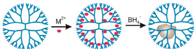
SCHEME 6. Crook's Synthesis of a Nanoparticle inside a PAMAM Dendrimer a
