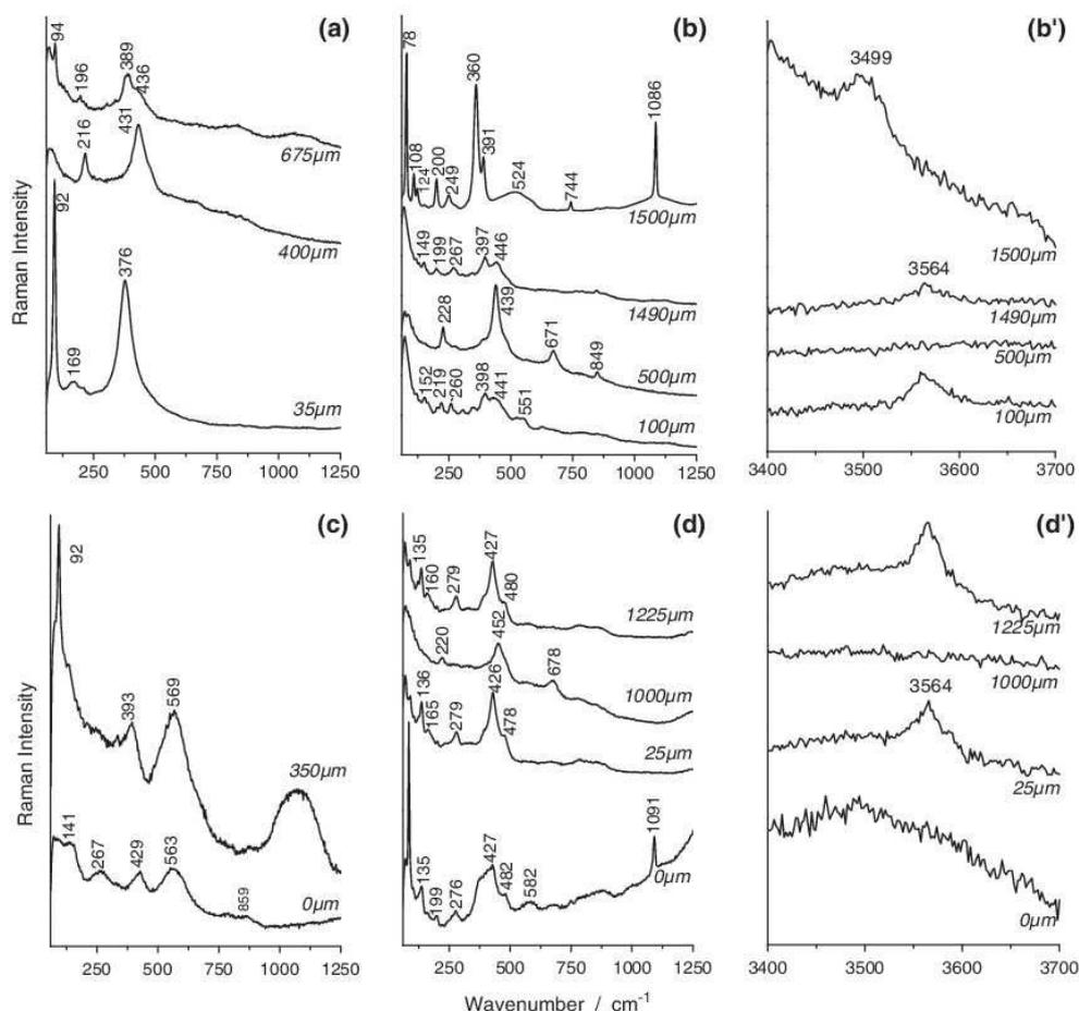
**Fig. 9.** Detail of the Raman profilometry along the fresh section fracture of LNO (a, b and b') and PNO (c, d and d') ceramic pellets protonated using lean- $\text{CO}_2$  (a and c) and rich- $\text{CO}_2$  (b and b'; d and d') water.
