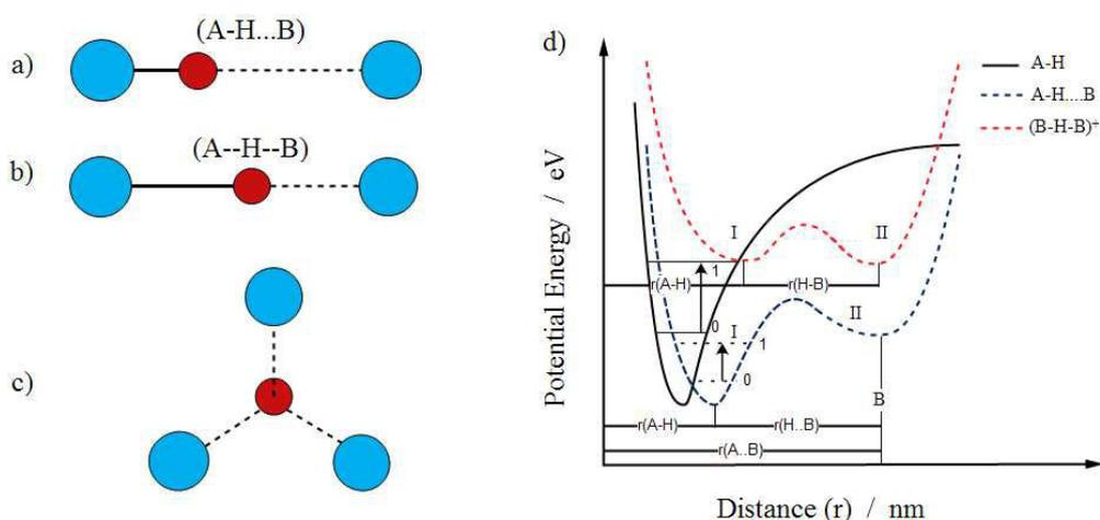
**Figure 1.2:** Schematic of a single donor acceptor of hydrogen interaction (a-b), of an ionic proton (c); and d the potential energy well of proton involved in the A-H..B hydrogen bond [12,15], Note: the red ball represents proton.
