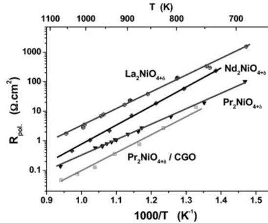
**Figure 2.8:** Arrhenius plots of the polarization resistance ( $R_{pol}$ ) of  $Ln_2NiO_{4+\delta}$  ( $Ln = La, Nd, Pr$ ) [126].
