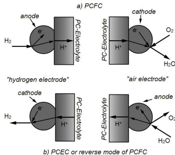
**Figure 2.7:** Working diagram of anode and cathode of PCFC (a) and PCEC – reverse mode of PCFC (b) Note: a part involve with fuel may call 'hydrogen electrode' and one involve with oxygen/air call 'air electrode'.
