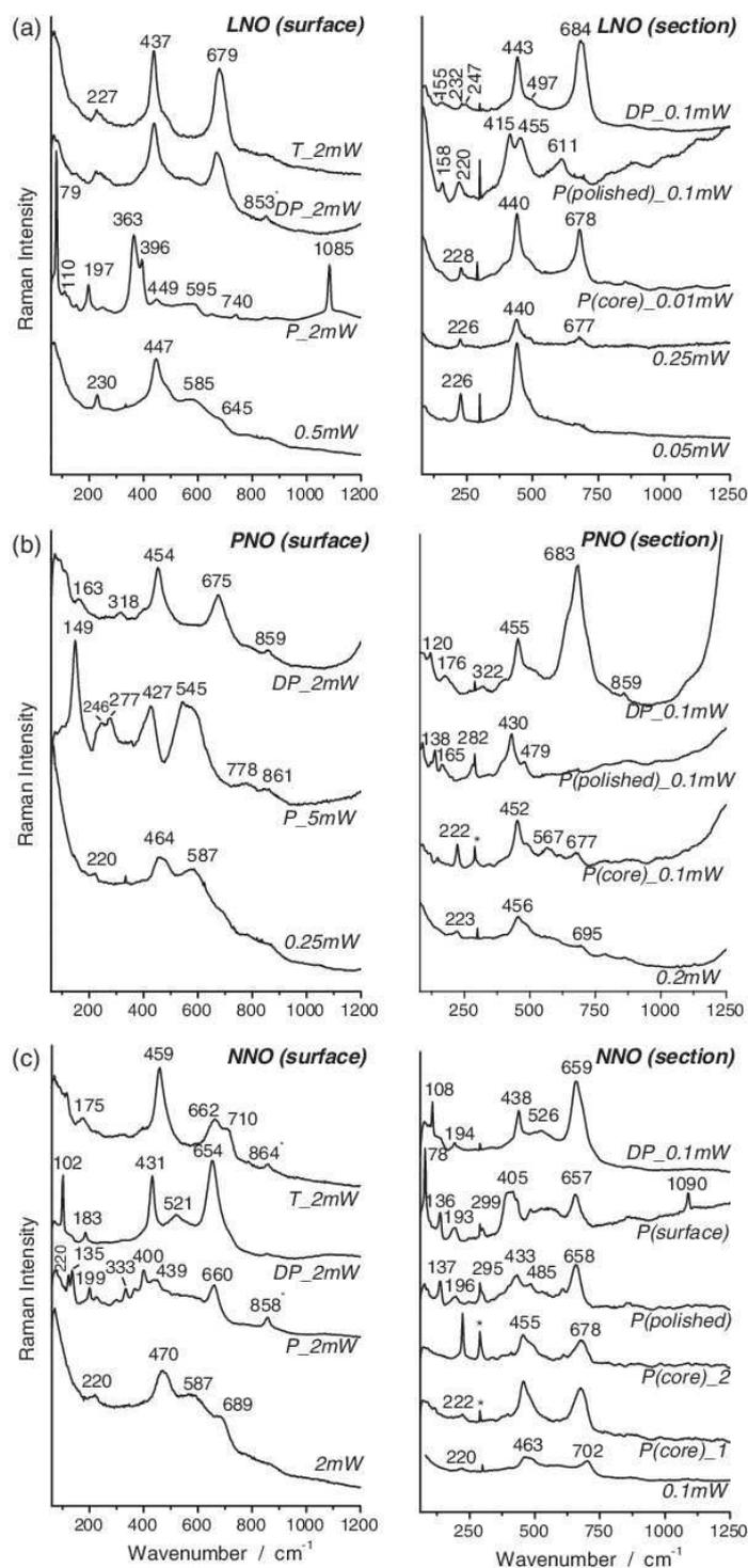
**Fig. 4.** Representative Raman spectra (a) recorded with blue (458 nm) laser line of pristine, protonated (P: 40 bar, 7 days and 55 bar, 8 days), de-protonated (DP) and thermally treated (T) of LNO (a), PNO (b) and NNO (c). The laser power at sample is given; 50× microscope objective is used. In (b) spectra recorded at low and very low laser power are given. The pellet is polished (P) in order to record representative spectra of the different layers.
