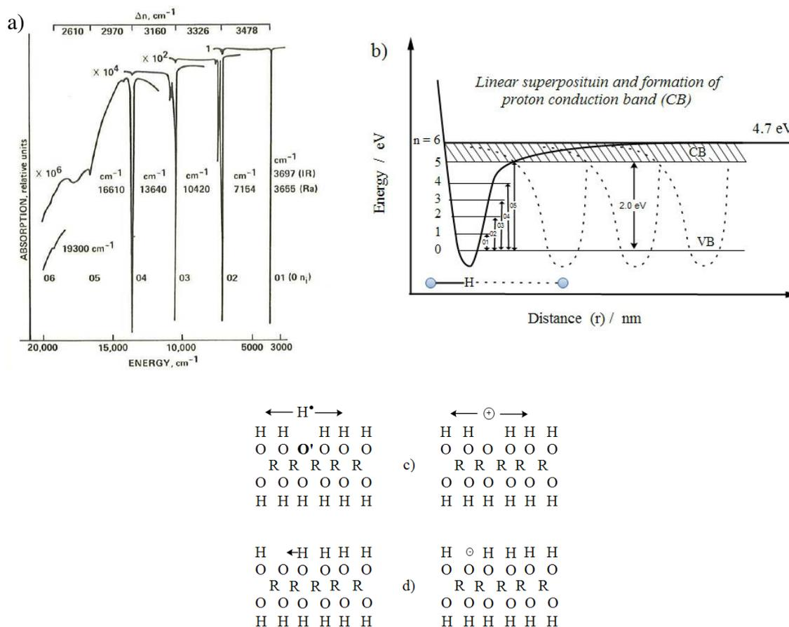
**Figure 1.3:** a) overtone series of the stretching mode in  $Mg(OH)_2$  b) Morse potential well of  $Mg(OH)_2$  and its linear superposition schematically presented the formation of proton conduction band (CB) above the fifth excited level, c) delocalization of proton in CB, d) diffusion of a proton vacancy [18].
