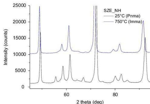
**Fig. 5.** Neutron diffraction patterns in limited 2 theta range characteristic of non-protonated SZE ceramics recorded at 25 °C and 750 °C. The disappearance of some Bragg peaks reveals the presence of long range order structural phase transition from the Pnma orthorhombic to the Imma pseudo tetragonal symmetry. Results of neutron diffraction refinements at RT, 500 °C and 800 °C can be found in Fig. S3.
