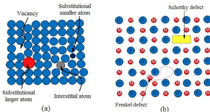
**Figure 1.1:** Scheme of (a) Point defects (b) Schottky and Frenkel defect forms in metal oxides solids (MO).
