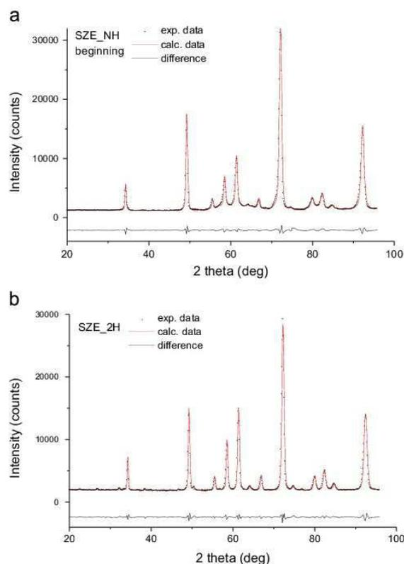
Fig. 2. Examples of neutron diffraction pattern refinement characteristic of (a) non-protonated, pristine (b) 2<sup>nd</sup> time protonated SZE proton conductor. Other examples can be found in Fig. S1.
