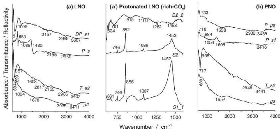
**Fig. 8.** ATR and microATR-FTIR ( $\mu$ ) spectra recorded at the surface of protonated (P), de-protonated (DP) and thermally treated (T) LNO and PNO ceramics. Comparison is made with protonated LNO ceramic using  $\text{CO}_2$  saturated water. The in-depth probed surface layer varies when Germanium ( $\mu$  ATR FTIR) or Diamond (ATR FTIR) are used.
