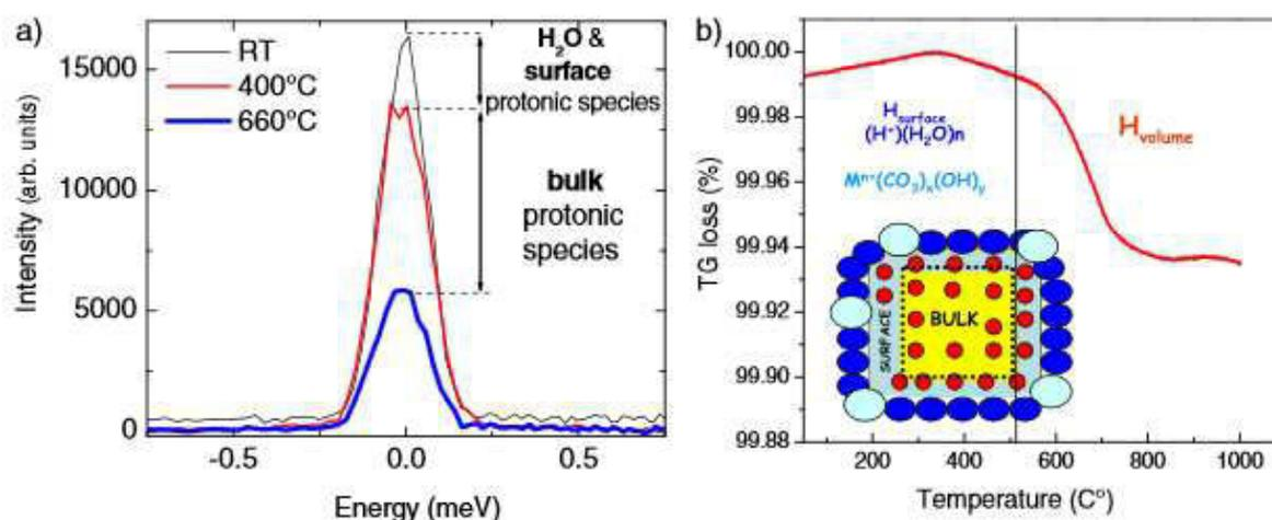
**Figure 1.6:** Determination of protonic species content : (a) elastic peak intensity variation as a function of temperature and (b) mass loss detected by TG analysis in the case of  $\text{SrZrLnO}_{3-\delta}$  [14,37], Note: schema draw in (b) illustrates the distinction of bulk and surface protons.
