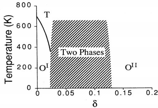
**Figure 2.4:** Approximate structural phase diagram for  $\text{La}_2\text{NiO}_{4+\delta}$  [55].
