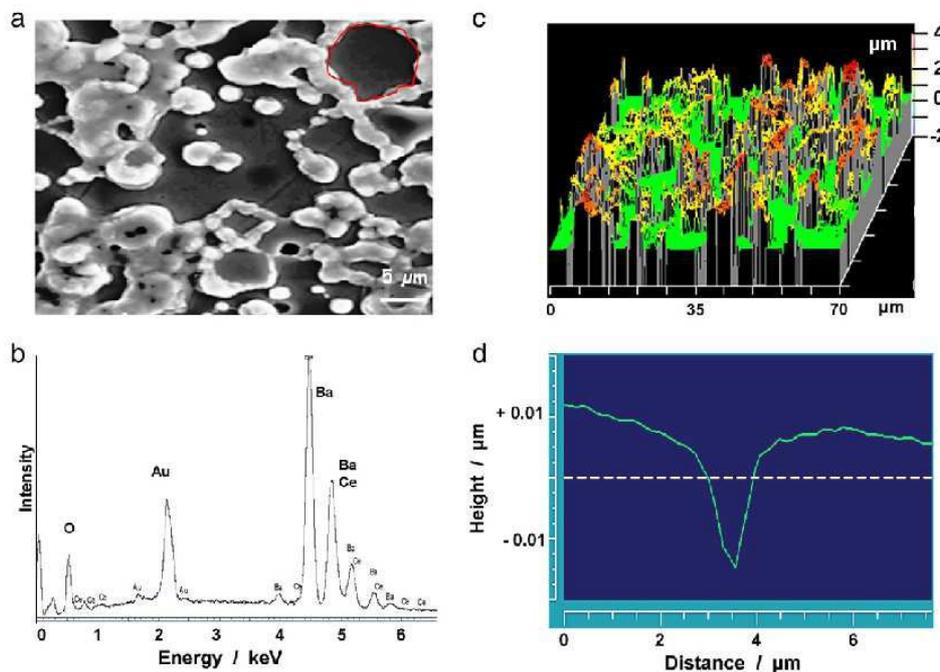
Fig. 2. Polished BCZYZ, annealed in 60 mbar  $\text{H}_2\text{O}$  for 12 h at 400 °C SEM micrograph (a) and EDX (b) analysis showing Ba-rich surface features. c) A white light interferometry measurement showing the surface topography. d) The grain, boundary is especially sensitive to the formation of Ba-rich formation.
