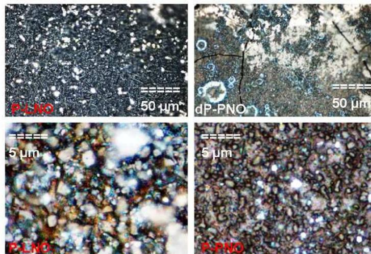
Fig. 1. Optical microphotographs of the surface of protonated LNO (P-LNO) and PNO (P-PNO) ceramics at different magnification. Comparison is given with de-protonated PNO sample (dP-PNO).
