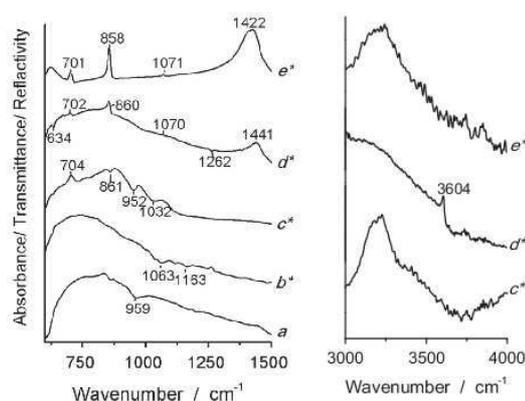
Fig. 8. ATR and micro ATR-FTIR spectra recorded at the surface of as-prepared (a, b), protonated under 20 bar free- $\text{CO}_2$  (c), under 40 bar free- $\text{CO}_2$  (d), 40 bar absorbed- $\text{CO}_2$  (e) and thermal treatment (f). (Note: \* indicates the spectra collected with the  $\mu$ -ATR Ge crystal).
