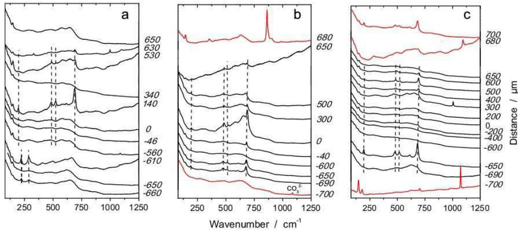
Fig. 9. Raman mapping along the fresh cross-section fracture of LSCF6428 ceramic pellets protonated under (a) 20 bar of  $\text{CO}_2$ -free water, (b) 40 bar of  $\text{CO}_2$ -free water, and (c) 40 bar of  $\text{CO}_2$  saturated water.
