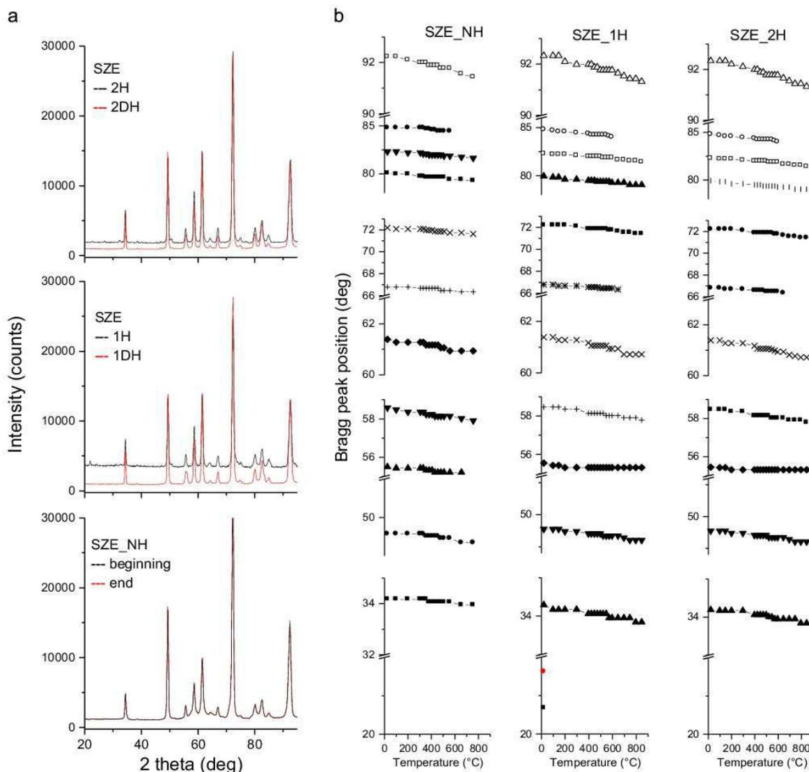
**Fig. 3.** Neutron diffraction patterns recorded at the beginning and the end of each measurement cycle (a) and temperature dependences of Bragg peak positions (b) characteristic of non-protonated, first time protonated and second time protonated SZE proton conductor. Zoom of neutron diffraction patterns presented in Fig. 3 can be found in Fig. S2.
