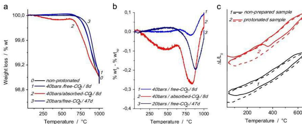
Fig. 6. (a) Thermal analysis of as-prepared and protonated LSCF6428 (b) corresponding TG weight loss difference,  $\%wt_p - \%wt_{np}$ . (c) Two consecutive thermal expansion (length variation/initial length) curves of as-prepared and protonated LSCF6428 under free- $\text{CO}_2$  water pressure.
