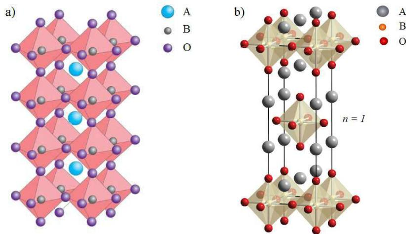
**Figure 2.1:** a) *Ideal perovskite structure (ABO<sub>3</sub>)* b) *a perovskite-related structure in Ruddelsden-Popper phase, (A<sub>2</sub>BO<sub>4</sub>)* [3].
