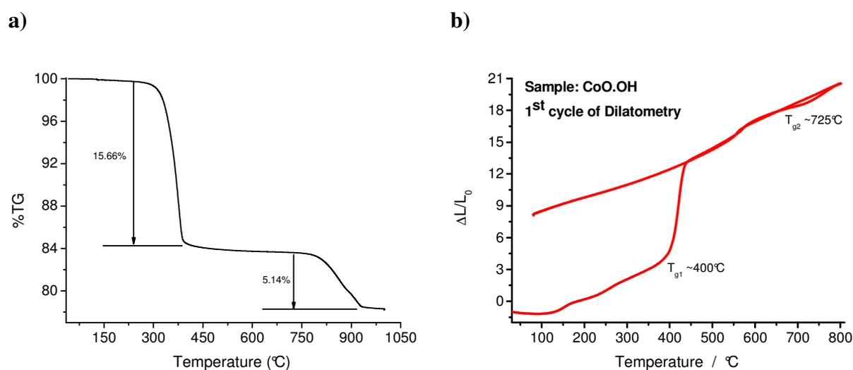
**Figure 3.3:** Thermal analysis of CoOOH (black mining) a) TGA curve under He-atmosphere, 10°C.min<sup>-1</sup> and b) Thermal expansion curve under Ar-atmosphere, 10°C.min<sup>-1</sup>.
