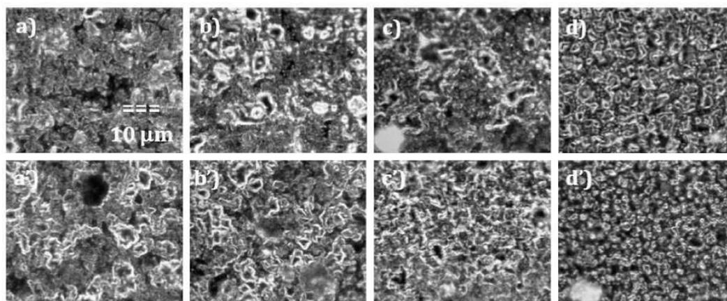
Fig. 5. Micro-features ( $10\ \mu\text{m}$ ) of LSCF6428's surface sample in different states (a) as-prepare sample (b) 40 bar of  $\text{CO}_2$ -free water pressure for 8 days (c) 20 bar of  $\text{CO}_2$ -free water pressure for 47 days (d) 40 bar of  $\text{CO}_2$ -saturated water pressure for 8 days.
