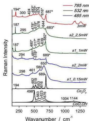
Fig. 3. Raman signatures of as-prepared LSCF6428 ceramic at different surface area/laser power/wavelengths and of  $\text{Co}_3\text{O}_4$  obtained by thermal treatment of  $\text{CoOOH}$  [44]. (\*corresponds to  $\text{Co}_3\text{O}_4$  traces).
