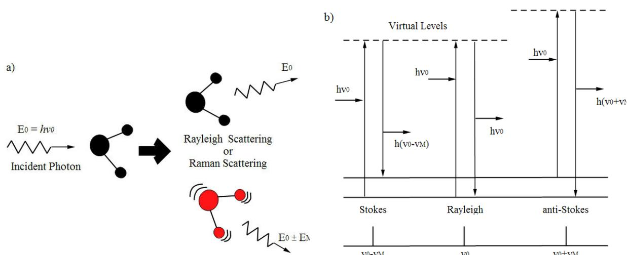
**Figure D.3:** a) Schematic Rayleigh and Raman scattering processes (an incident photon can either scatter elastically or inelastically from a molecule) and b) Stokes scattering and anti-Stokes scattering.
