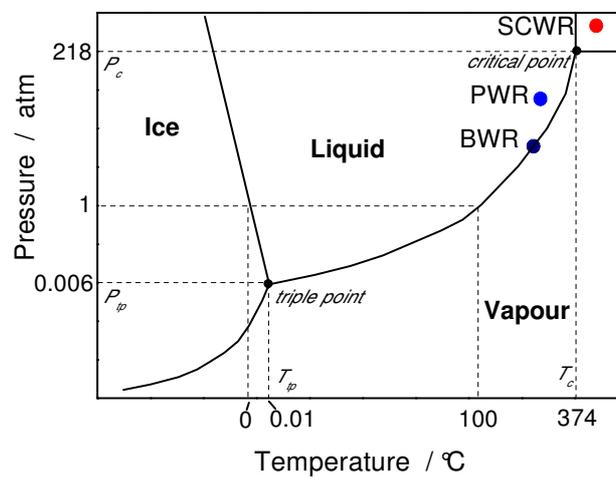
**Figure 4:** Phase diagram of the one component  $\text{H}_2\text{O}$  and indication of the working conditions of different reactor types in nuclear power plant detailed in the text (note: the diagram is not to scale and three data points of reactor's working condition in hydrogen production nuclear plant were collected from literature [46]).
