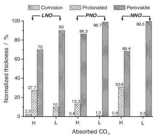
**Fig. 7.** Comparison of the thickness of the different layers formed after autoclave treatment in  $\text{CO}_2$ -lean (L) and -rich (H) water for 5 day at  $40\text{ bar H}_2\text{O}$ .
