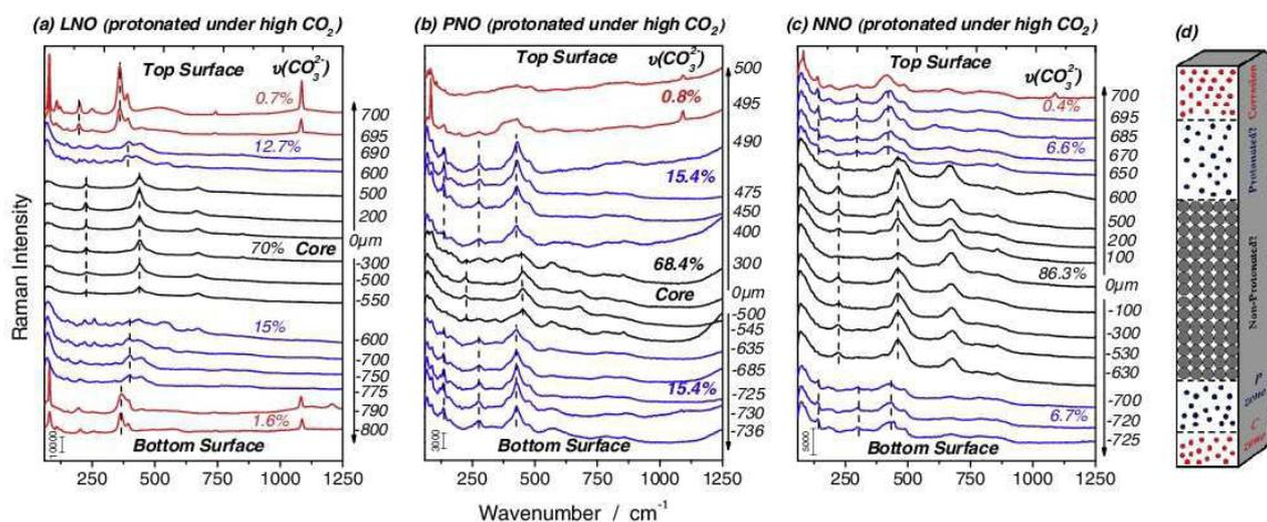
**Fig. 6.** Raman profilometry along the fresh section fracture of LNO, NNO and PNO ceramic pellets protonated using lean- $\text{CO}_2$  and rich- $\text{CO}_2$  water. The use of low magnification microscope objective (e.g.  $10\times$ ) lowers the illumination power/surface unit and avoids phase modification under the laser spot. Scheme of different layers detected in LnNO ceramics (d).
