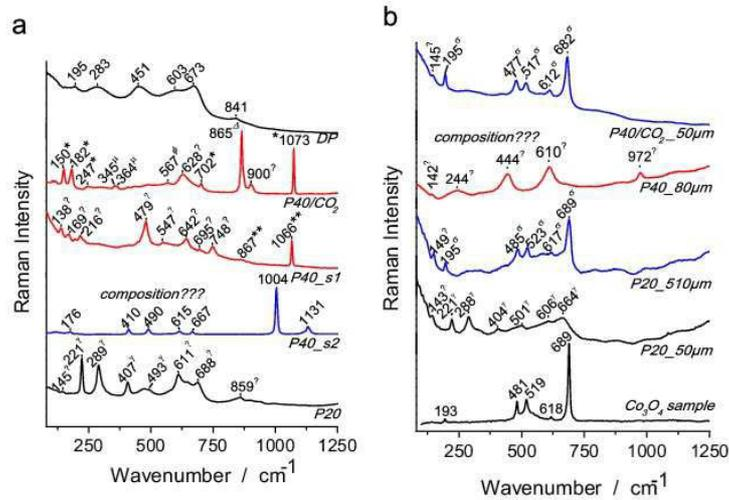
Fig. 7. Raman spectra of LSCF6428 ceramic in different states, protonated and deprotonated, recorded (a) on surface (b) in bulk. (Note: the used symbols are described in Table 2 and sample labels are indicated in the text).
