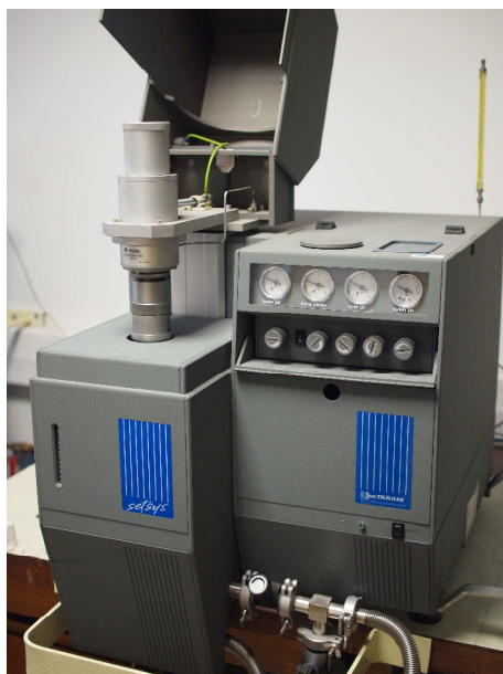
Figure C.4: The thermal expansion (TE) Setaram Setsys 1650 dilatometer instrument equipped with amorphous silica rod and support.
