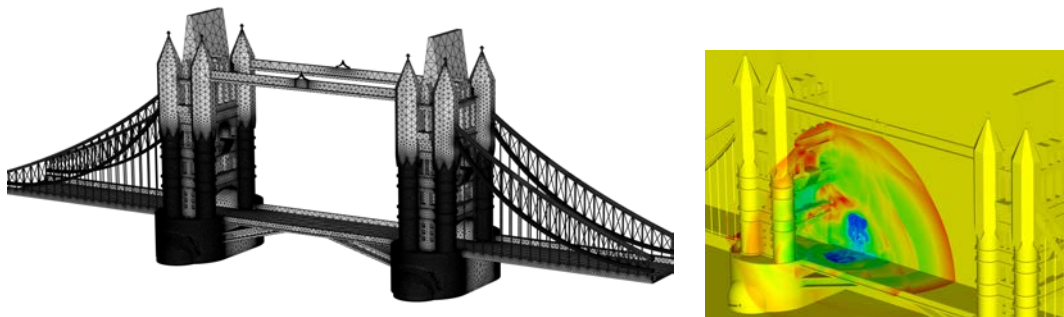
Figure 2.10: Tower-bridge test case. Initial mesh and geometry (left) and density iso-values of the the blast on an adapted mesh (right).
