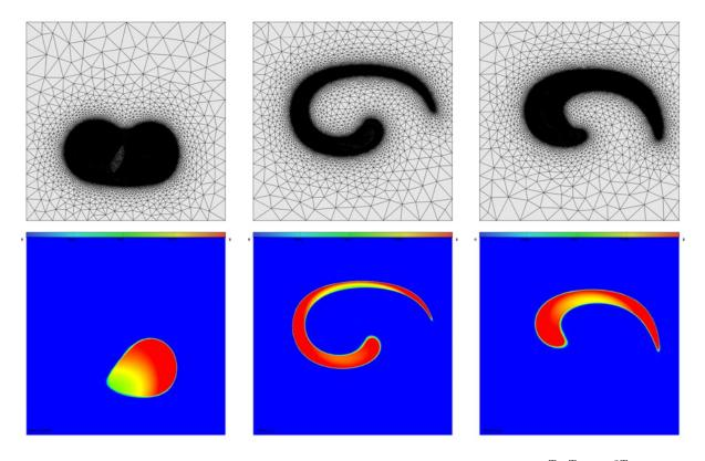
Figure A.9: Adapted meshes and the corresponding densities at times  $t = \frac{T}{16}, \frac{T}{4}$  and  $\frac{3T}{8}$ .
