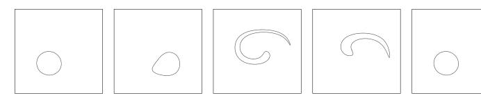
Figure A.7: The 2D bubble's interface at several times from t = 0 to  $t = \frac{T}{2}$  (from left to right:  $t = 0, \frac{T}{16}, \frac{T}{4}, \frac{3T}{8}, \frac{T}{2}$ ). A spatial error is computed at each  $t \in \frac{T}{2}\mathbb{N}$  to evaluate the diffusion due to the numerical model.
