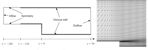
Figure 4.10: 2D step: Test case description.
