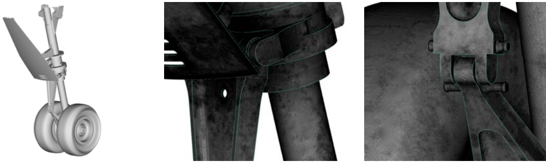
Figure 2.12: Landing gear test case. Geometry of the landing gear (left) and closer view of the surface mesh around some geometrical details (middle and right).
