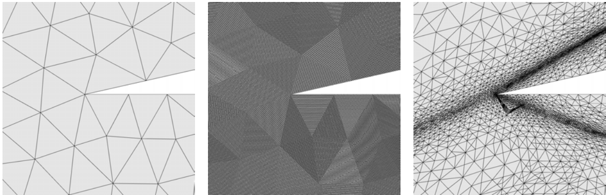
Figure 5.6: Close-up views of three nested meshes of a 2D scramjet. Left: the initial coarse mesh. Middle: all the edges of the mesh were refined. Right: only some edges were refined. Both nested meshes (middle and right) contain elements of bad quality due to the constraints from the initial discretization.
