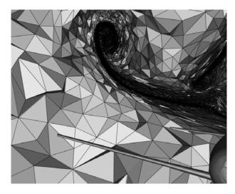
Figure 6.15: Transonic WBT configuration: cut in the trailing vortices region of the final adapted mesh.
