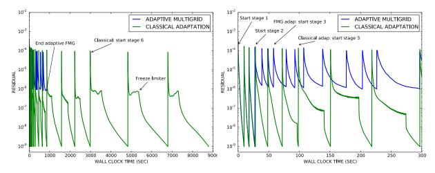
Figure 6.9: 3D subsonic NACA 0012: comparison of the residual convergence in terms of wall clock time. Left: whole simulation. Right: close-up view of the first stages. Note that each stage corresponds to a mesh complexity, and that three sub-iterations were performed for each one of them.
