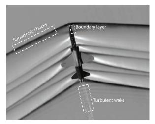
(a) A recent schlieren photograph of a T-38C flying at Mach 1.09 (Credit: NASA).
