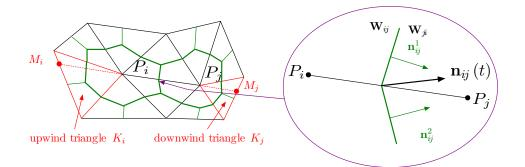
Figure 3.5: Illustration of finite volume cell construction in 2D: two neighbouring cells  $C_i$  and  $C_j$  and the upwind triangles  $K_i$  and  $K_j$  associated to edge  $P_i P_j$ .
