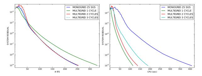
Figure 5.21: 3D subsonic NACA 0012 : Convergence of the residual of the whole simulation. Left: number of time steprations. Right: wall clock time (sec).
