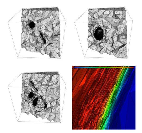
Figure A.18: Adapted meshes for the 3d bubble motion. Top: cuts in the volume at times  $t = \frac{T}{8}$  and  $\frac{T}{2}$ . Bottom: cuts in the volume at time  $t = \frac{3T}{4}$  (right: close-up view of the bubble's interface).
