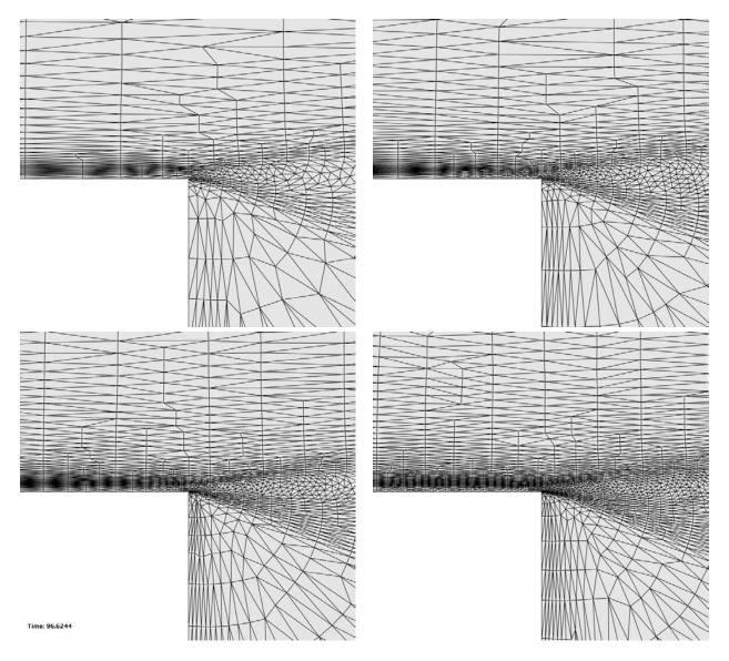
Figure 7.5: Backward facing step: mesh resolution around the corner for the complexity  $24 \,\mathrm{K}$ , to  $36 \,\mathrm{K}$  for the multi-field multi-scale metric from left to right, top to bottom.
