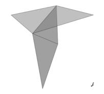
Figure 2.6: Example of a non-manifold configuration (here three faces share an edge).
