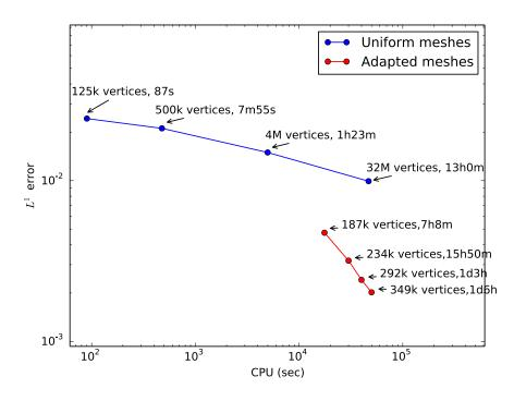
Figure A.17: Spatial  $L^1$  error in 3D at time t = T vs the total CPU time of each simulation.
