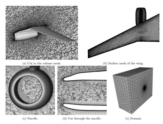
Figure 4.19: DPW2: Coarse mesh of the Wing/Body/Nacelle configuration.
