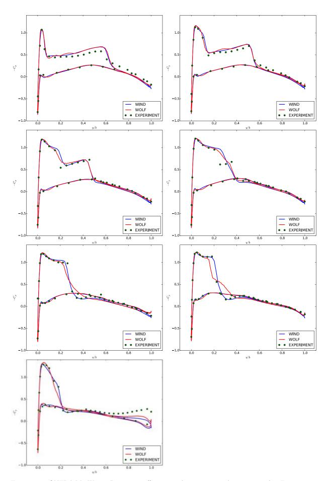
Figure 4.17: ONERA M6 Wing : Pressure coefficients at the 6 extraction lines presented in Figure 4.16.
