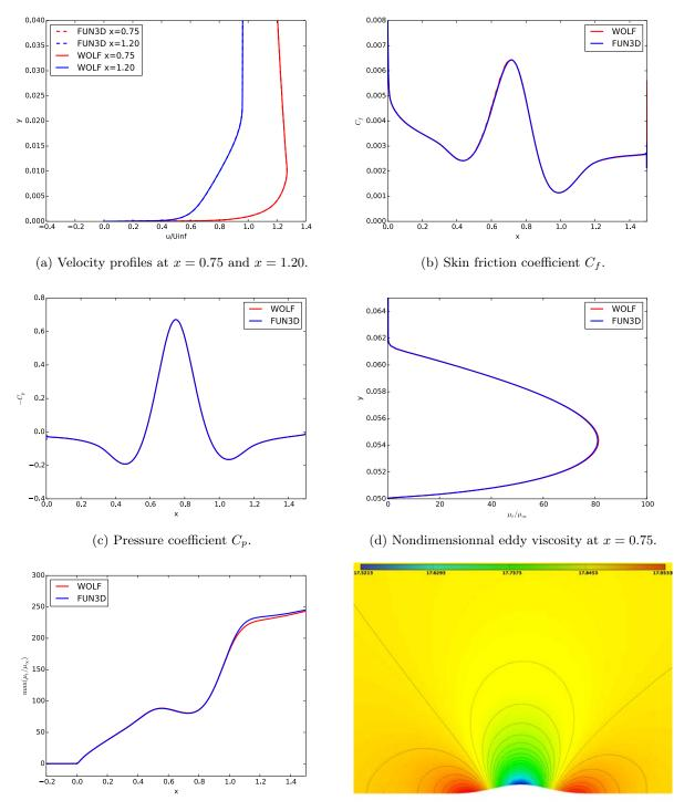
(e) Maximal nondimensionnal eddy viscosity as a function of x.
