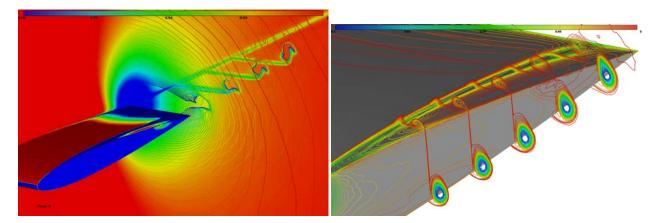
Figure 6.12: 3D subsonic NACA 0012 : velocity isovalues.
