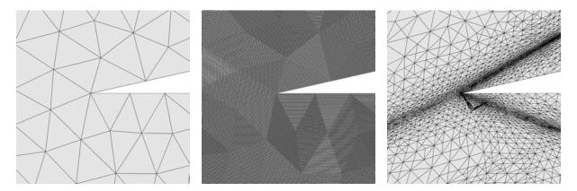
Figure 5.6: Close-up views of three nested meshes of a 2D scramjet. Left: the initial coarse mesh. Middle: all the edges of the mesh were refined. Right: only some edges were refined. Both nested meshes (middle and right) contain elements of bad quality due to the constraints from the initial discretization.
