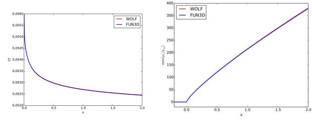
(c) Turbulent flat plate: Surface skin friction coefficient (d) Turbulent flat plate: Maximum nondimensional eddy on finest mesh  $(545 \times 385)$ . viscosity as a function of x.
