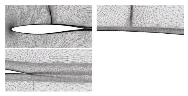
Figure 7.8: RAE 2822: Views of the final adapted mesh using the  $\mathcal{M}_G$  metric and the metric-aligned meshing method.
