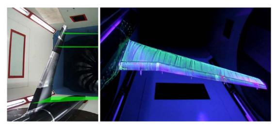
Figure 1: Wind tunnels are tube-shaped facilities, which use powerful fans to move air over a model of aircraft. It teaches a lot about the aircraft aerodynamics, and is extensively used during the design process. (Image credit: NASA).
