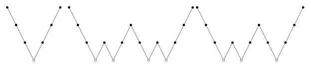
Figure 5.2: Four-grid methods : V-cycle, W-cycle and F-cycle ( $\bullet$  : 1 smoothing SGS iteration,  $\circ$  : Several SGS iterations)
