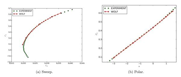
Figure 4.21: DPW2: Results of the drag polar study for the Wing/Body condiguration.
