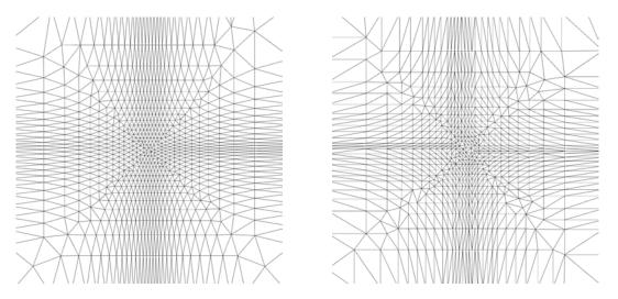
Figure 7.1: Illustration of alignement strategies on a simple analytic function. Left, metric-aligned anisotropic mesh adaptation. Right, metric-orthogonal anisotropic mesh adaptation.
