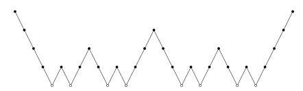
Figure 5.3: A five-grid method: W-cycle ( $\bullet$ : 1 smoothing SGS iteration,  $\circ$ : Several SGS iterations)
