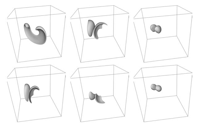
Figure A.14: Result of the computation on the uniform mesh containing 32 Million vertices. The bubble's interface (iso-surface  $\rho = 0.95$ ) at times  $t = \frac{T}{8}, \frac{T}{4}, \frac{T}{2}, \frac{3T}{4}, \frac{7T}{8}$  and T.
