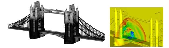
Figure 2.10: Tower-bridge test case. Initial mesh and geometry (left) and density iso-values of the the blast on an adapted mesh (right).
