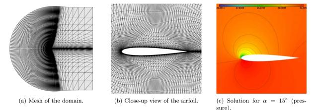
Figure 4.7: Mesh of the NACA 0012 airfoil.
