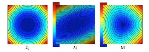
Figure 1.6: Iso-values of the function  $f(\mathbf{x}) = \ell_{\mathcal{M}}(\mathbf{ox})$  where **o** is the origin for different Riemannian metric spaces. Left, canonical Euclidean space  $(\Omega, \mathcal{I}_2)$ , middle, Euclidean metric space  $(\Omega, \mathcal{M})$  with  $\mathcal{M}$  constant and, right, Riemannian metric space  $(\mathcal{M}(\mathbf{x}))_{\mathbf{x}\in\Omega}$  with a varying metric tensor field.
