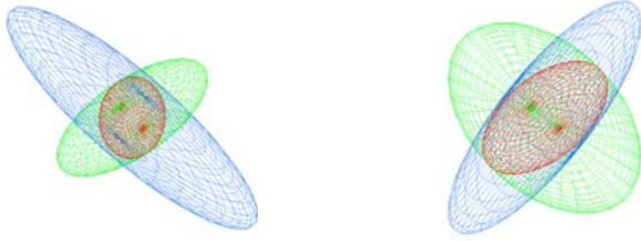
Figure A.6: Two illustrations of the metric intersection procedure. \mathcal{M}_1 (in blue) is intersected with \mathcal{M}_2 (in blue). The resulting metric \mathcal{M}_1 \cap \mathcal{M}_2 is in red.
