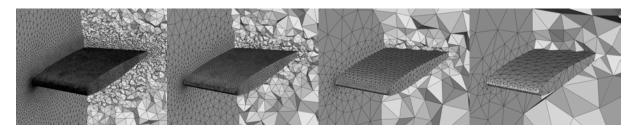
Figure 5.14: 3D subsonic NACA 0012 : Cuts in the volumes of the four meshes used during the multigrid computations. Number of vertices, from left to right: 271 311, 34 452, 4 940, 1 007.
