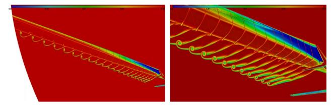
Figure 6.17: Transonic WBT configuration: views of the wing-tip vortices in the wake.
