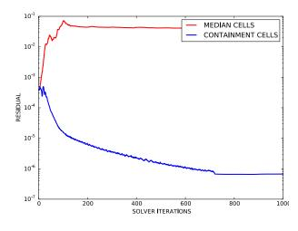
Figure 3.2: 2D turbulent bump: comparison of the residual convergence using the median and the containment cells. For this case, we were unable to converge the computation on median cells (different sets of input parameters have been tried).
