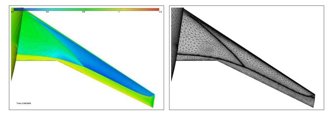
Figure 6.16: Transonic WBT configuration: pressure on the wing and corresponding adapted surface mesh.
