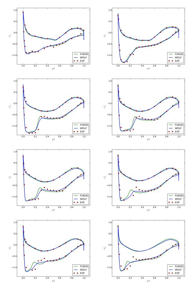
Figure 4.24: DPW2 validation : Wing Body Configuration (sections from 1 to 8).
