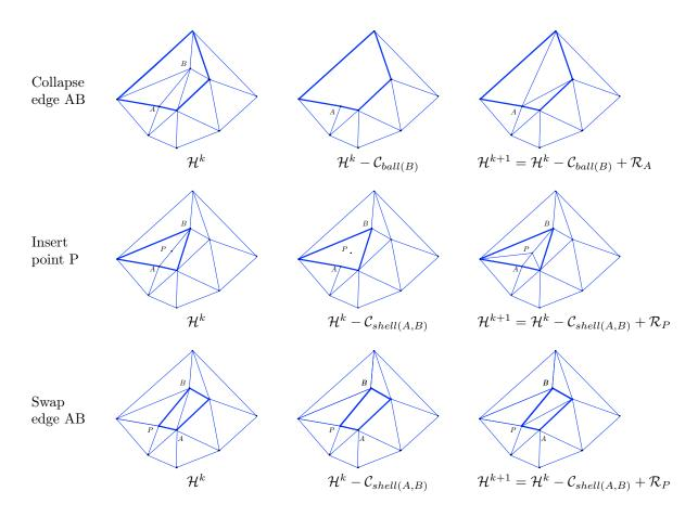
Figure 1.8: Some 2D meshing operators reinterpreted as a cavity-based operator with an appropriate choice of the point to (re)insert and cavity to remesh. From top to bottom, the collapse, insertion and swap operators.
