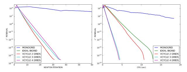
Figure 5.16: Transonic NACA: Comparison of the V-cycles for the convergence of the Newton method after 120 time steps.
