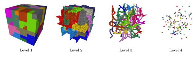
Figure 2.3: Recursive partitioning into 32 sub-domains of a cubic domain for a constant work per element. From left to right, level 1, 2, 3 and 4 of partitioning. We observe that the domain topology varies drastically with the level.
