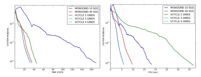
Figure 5.18: 2D transonic NACA: Convergence of the residual of the whole simulation. Left: number of time steps. Right: wall clock time (sec).
