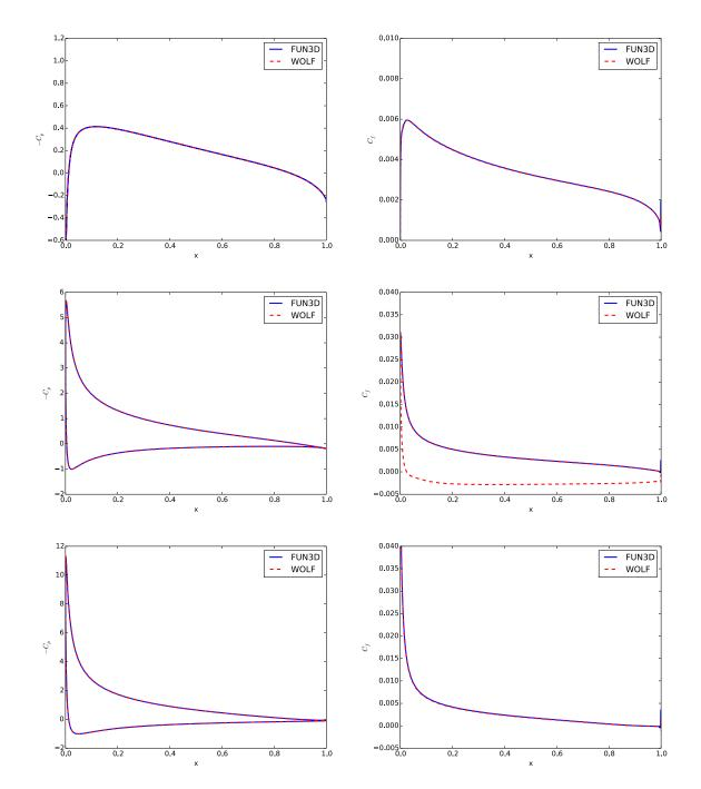
Figure 4.8: NACA0012: Pressure coefficient  $C_p$  (left column) and skin friction coefficient  $C_f$  (right column) for  $\alpha = 0, 10, 15^{\circ}$  (first, second and third line, resp.). Comparison to FUN3D ( $C_p$  and  $C_f$ ).
