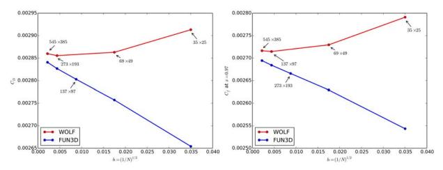
(a) Turbulent flat plate: Drag convergence.
