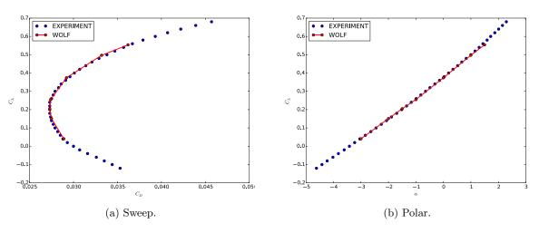
Figure 4.22: DPW2: Results of the drag polar study for the Wing/Body/Nacelle condiguration.
