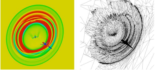
(c) Mesh adaptation result: solution (left) and adapted mesh (right).
