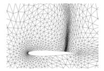
(d) Adapted mesh obtained after 3 stages of Algorithm 1 (2 200 vertices).
