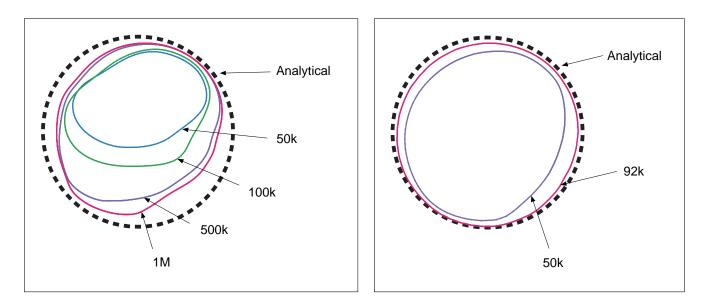
Figure A.8: Comparison of the bubble's interface at  $t = 10\frac{T}{2}$ . Left: uniform meshes. Right: unsteady mesh adaptation.
