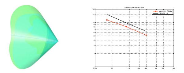
Figure 1.12: Supersonic SSBJ. Left, Mach cone emitted by the SSBJ. The maximal Mach cone diameter is 2.5 km. The solution is accurately propagated in the whole computational domain. Right, global  $L^2$  norm spatial convergence for the local Mach number on a sequence of adapted meshes.
