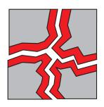
(c) Mesh adaptation is performed in parallel on each partition. The mesh elements constrained by an interface are tagged in red.
