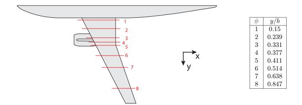
Figure 4.23: Drag Prediction Workshop: Location of the 8 extraction lines. b refers to the wing span.
