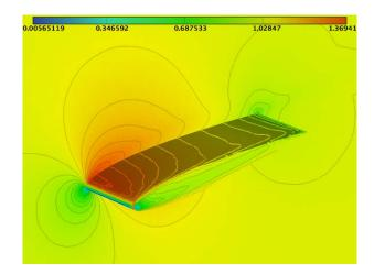
Figure 5.20: 3D subsonic NACA 0012: Solution (velocity).
