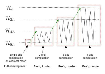
Figure 6.1: Description of the FMG algorithm.  $\rightarrow$  : linear interpolation of the solution
