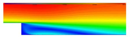
Figure 4.12: 2D step : Mapping of the velocity (finest mesh).
