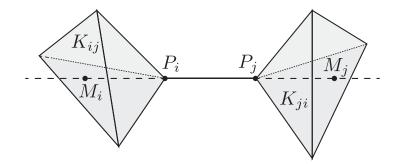
Figure 3.6: Downwind  $K_{ij}$  and upwind  $K_{ji}$  tetrahedra associated to edge  $P_i P_j$ .
