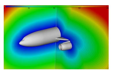
Figure B.1: Mapping of the distance function around a wing/body/nacelle configuration (mesh from the 2nd drag prediction workshop).
