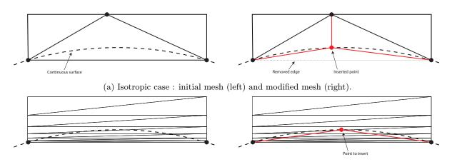
(b) Viscous case. The anisotropy in the immediate vicinity of the surface makes it difficult to refine it.Figure 7.10: Illustration of one difficulty of surface reprojection when boundary layer meshes are involved.
