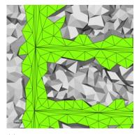
(c) Close-up view of the interface mesh after correction. Cavity elements are added.
