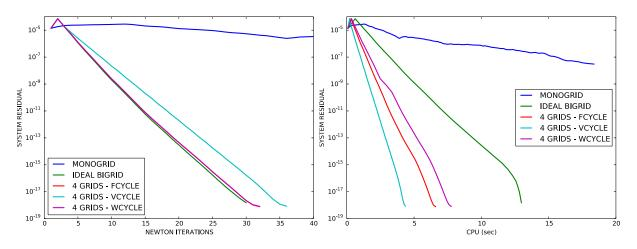
Figure 5.17: Transonic NACA: Comparison of the V, the W and the F cycles (using 4 grid levels) for the convergence of the Newton method after 120 time steps.
