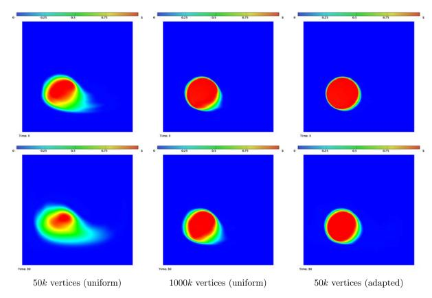
Figure A.13: Comparison of the mapping of the density at times  $t = \frac{T}{2}$  (top row) and  $t = 10\frac{T}{2}$  (bottow row). Three computations are compared: two uniform meshes of 50k vertices and 1M vertices (1st and 2nd column resp.) and adapted meshes (~ 50k vertices each, 3rd column).
