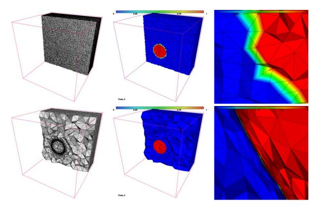
Figure A.3: Steady mesh adaptation at time t = 0. Top: cuts in the initial uniform mesh. Bottom: cuts in the final adapted mesh which is refined at the bubble's interface.
