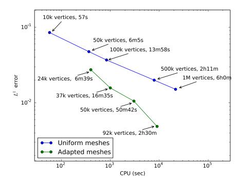
Figure A.12: Spatial  $L^1$  error in 2D at time  $t = 10\frac{T}{2}$  vs the total CPU time of each simulation.
