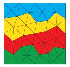
(b) A good partitioning: the blue and the red blocks can be run simultaneously, as well as the yellow and the green.
