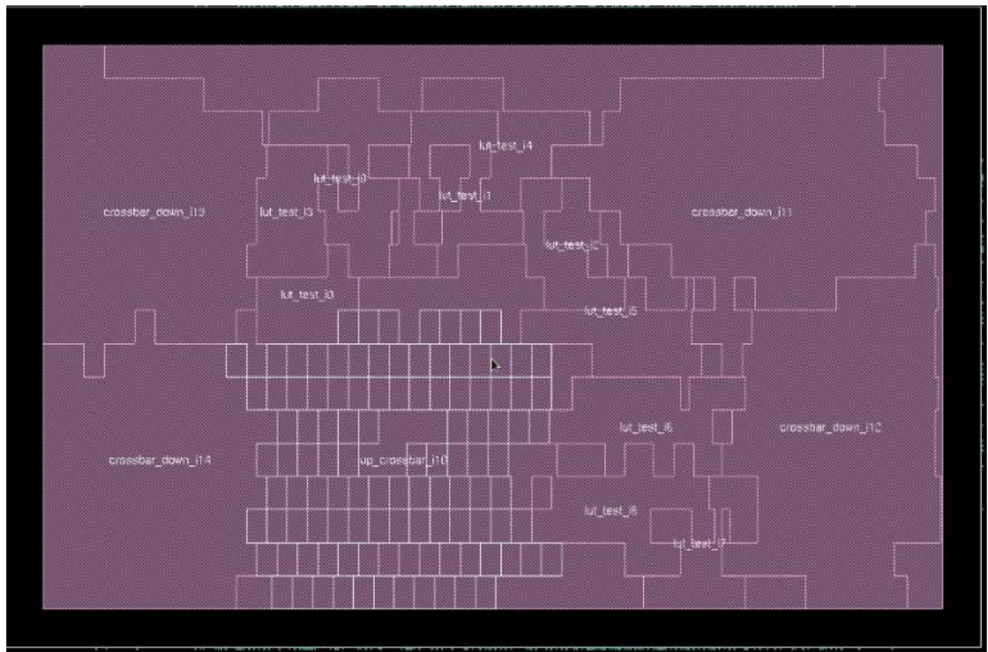
FIGURE 3.14 – Placement d'un cluster
