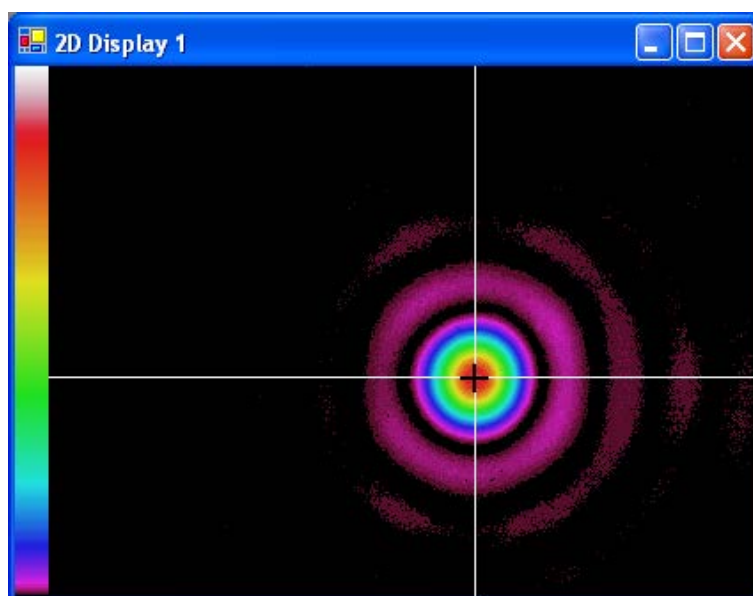
Figure 3.13. Probe beam profile after spatial filtering, measured by a CCD camera. The picture is done at \sim 10 cm after the pinhole. Diffraction pattern around the beam is blocked by following optics and does not propagate to the atoms position in MOT.
