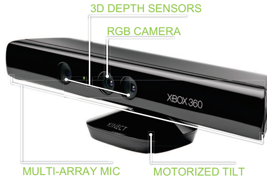
FIGURE 4.8: Kinect Sensor Description. Credits: Microsoft Website.
