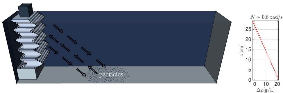
Figure 3.8: Schematics of the experimental setup used to study particle transport by internal gravity waves. The internal waves are generated at the side of the tank thanks to a wave generator. The particles are deposited at the bottom boundary in the region where the internal waves will pass through. On the right is plotted an experimental measurement of the density (crosses) as a function of the water depth.
