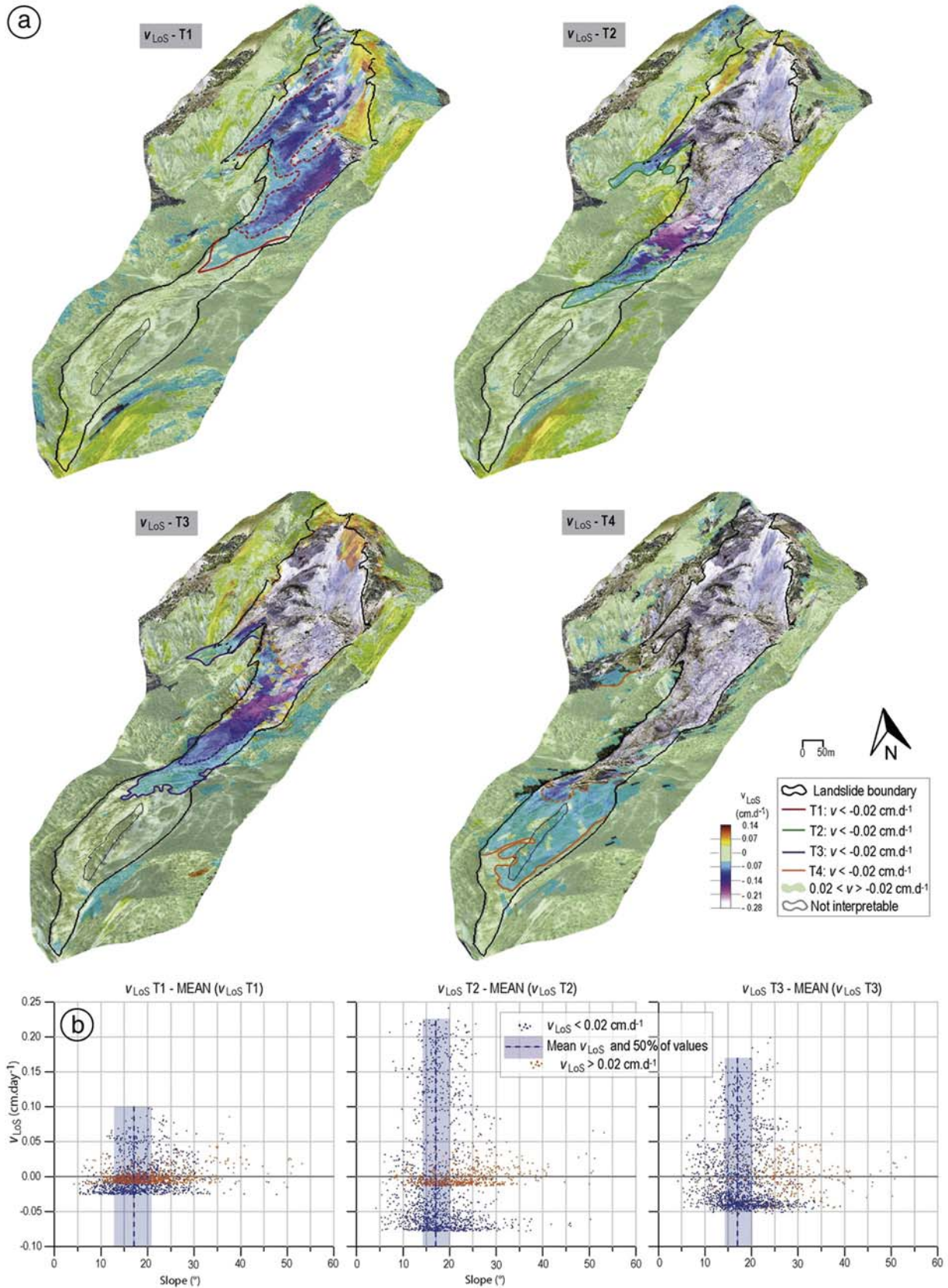
Fig. 14. InSAR displacement rates of the La Valette landslide for three periods in 2007 and 2009. (a) Maps of v_{LoS} values ( cm \cdot day^{-1} ) at T1, T2, T3 and T4; (b) plots of v_{LoS} values as a function of slope angle ( ^{\circ} ). The velocity estimated at one pixel location is represented in relation to the average velocity observed in the subsidence zone ( v_{LoS} > 0.02 \text{ cm} \cdot d^{-1} , in orange) and in the transit zone ( v_{LoS} < 0.02 \text{ cm} \cdot d^{-1} , in blue).
