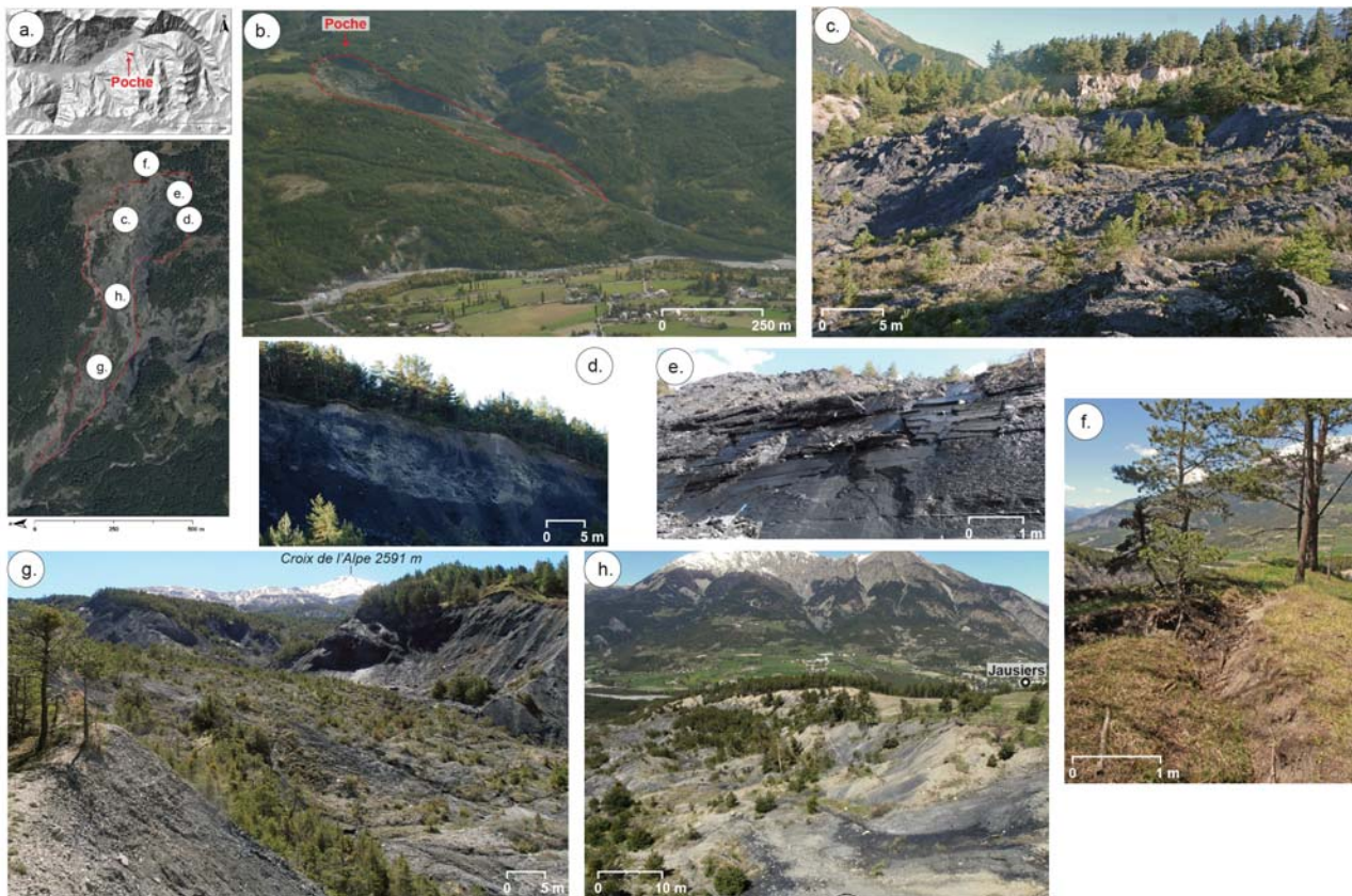
Figure 2-17: Morphology of the Poche landslide. (a) Orthophotograph of 2009 showing the landslide in red and locating the picture views (top represent the eastern direction). (b) View to the south from the opposite crest showing the whole landslide body (outlined in red). (c) View from the landslide body constituted by black marls to the NE part of the main scarp. (d) View of the southern main scarp and the contact between surficial soil, moraine deposits and black marls. (e) View on a rupture plan in the black marls dipping downslope. (f) View to northwest on a deep crack located close to the landslide crown (g) View to the south of the slowly moving landslide tongue. (h) View to the north from the top to the landslide body constituted by mixed moraine and marls deposits.
