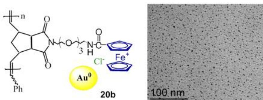
**Figure 15:** TEM analysis of **20b** at 100 nm.
