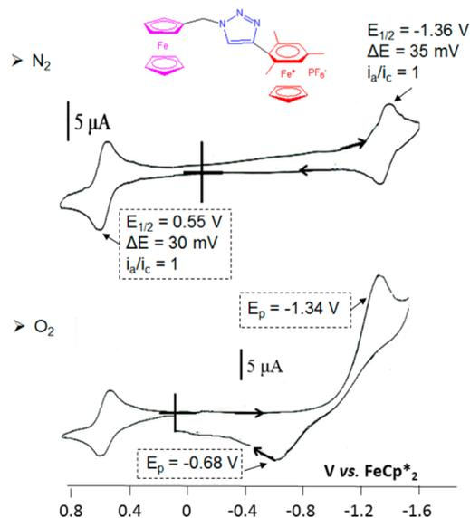
**Figure 1.** CVs of **5** under  $\text{N}_2$  and under  $\text{O}_2$  (air). Solvent, DMF; reference electrode, Ag; working and counter electrodes, Pt; scan rate,  $0.2\text{ V/s}$ ; and supporting electrolyte,  $[\text{n-Bu}_4\text{N}][\text{PF}_6]$ ,  $0.1\text{M}$ .
