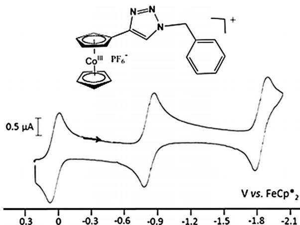
Figure 1. CV of **1** in THF. The wave at 0.0 V corresponds to the internal reference  $\text{FeCp}^*_2$ . Solvent: THF; reference electrode: Ag; working and counter electrodes: Pt; scan rate:  $0.2 \text{ V s}^{-1}$ ; supporting electrolyte:  $[n\text{Bu}_4\text{N}][\text{PF}_6]$ .
