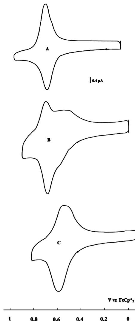
**Figure 7.** CVs for the titration of  $[n\text{-Bu}_4\text{N}]_2[\text{ATP}]$  by the modified Pt electrode with polymer  $6^{50}$  in  $\text{CH}_2\text{Cl}_2$  at  $20^\circ\text{C}$ : (A) before addition of  $[n\text{-Bu}_4\text{N}]_2[\text{ATP}]$ ; (B) during titration of  $[n\text{-Bu}_4\text{N}]_2[\text{ATP}]$ ; (C) after addition of excess  $[n\text{-Bu}_4\text{N}]_2[\text{ATP}]$ .
