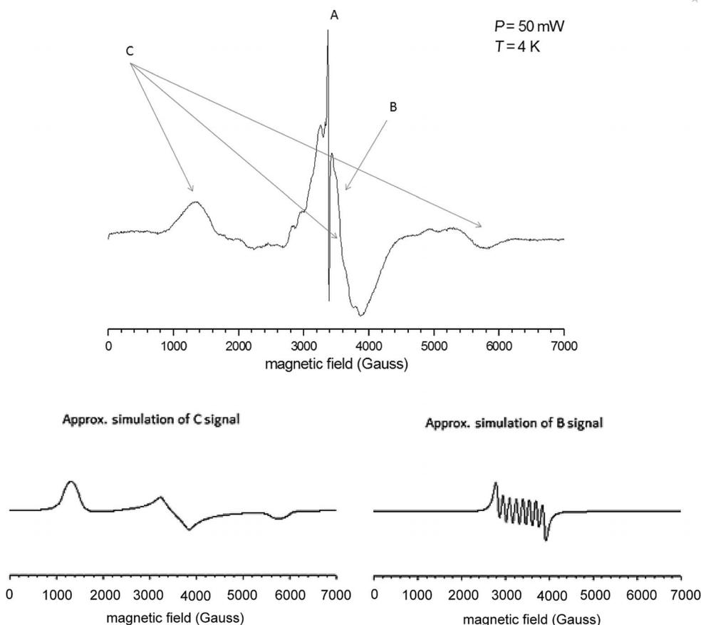
Figure 4. EPR analysis of **9** and approximate simulations of signals **B** and **C**.<sup>[62]</sup> Signal **A** gives  $g_{\parallel} = 2.037$  and  $g_{\perp} = 2.003$ . Signal **B** gives  $g = 2.015$  and the hyperfine coupling constant  $A(\text{Co} - \text{I} = 7/2) = 150$  G. The  $g$  values of signal **C** are  $g_1 = 1.17$ ,  $g_2 = 1.9$ , and  $g_3 = 5.09$ .
