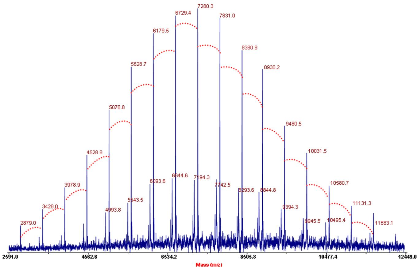
**Figure 3.** MALDI-TOF MS spectrum of polymer 6<sup>16</sup>. The molar feed ratio of monomer 5 to 1 is 16:1. The red dotted lines correspond to the difference between molecular peaks of a value of 550 ± 1 Da (MW of 5).
