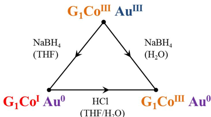
**Figure 7.** Reduction of G<sub>1</sub>Co<sup>III</sup>Au<sup>III</sup> by NaBH<sub>4</sub> leading to the selective reduction of either Co<sup>III</sup> (**AuNPs-10**) or Au<sup>III</sup> (**AuNPs-11**) and selective oxidation of G<sub>1</sub>Co<sup>I</sup>Au<sup>0</sup> (**AuNPs-11**) back to G<sub>1</sub>Co<sup>III</sup>Au<sup>0</sup> (**AuNPs-12**).
