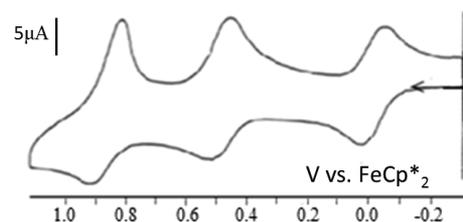
**Figure 3.** CV of the AuNPs 18. Solvent:  $\text{CH}_2\text{Cl}_2$ ; internal reference:  $\text{FeCp}^*_2$  ( $\text{Cp}^* = \eta^5\text{-C}_5\text{Me}_5$ ); reference electrode: Ag; working and counter electrodes: Pt; scan rate: 0.2 V/s; supporting electrolyte:  $[\text{n-Bu}_4\text{N}][\text{PF}_6]$ . The wave at 0.0 V corresponds to decamethylferrocene (reference).<sup>25</sup>
