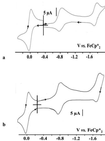
**Figure 5.** (a) CV of **4** in DMF. (b) CV of **5** in DMF. The wave at 0.0 V corresponds to the internal reference  $\text{FeCp}^*_2$ . Solvent: DMF; reference electrode: Ag; working and counter electrodes: Pt; scan rate: 0.2 V/s; supporting electrolyte:  $[\text{n-Bu}_4\text{N}][\text{PF}_6]$ .
