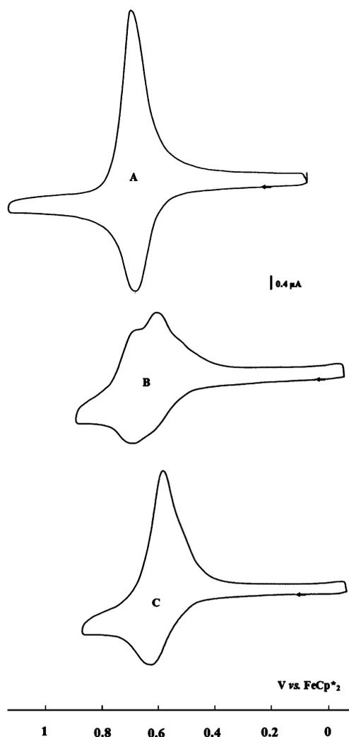
**Figure 5.** CVs for the titration of  $[n\text{-Bu}_4\text{N}]_2[\text{ATP}]$  with polymer  $6^{50}$  in  $\text{CH}_2\text{Cl}_2$  at  $20^\circ\text{C}$  by adding the salt of the anion to the polymer solution: (A) before addition of  $[n\text{-Bu}_4\text{N}]_2[\text{ATP}]$ ; (B) during the titration with 0.25 equiv of  $[n\text{-Bu}_4\text{N}]_2[\text{ATP}]$ ; (C) with 0.5 equiv of  $[n\text{-Bu}_4\text{N}]_2[\text{ATP}]$ .
