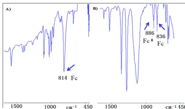
**Figure 3.** FT-IR spectra in KBr pellets of (A) **4**, 814  $\text{cm}^{-1}$  ( $\nu_{\text{Fc}}$ ) and (B)  $4(\text{BAR}_4^{\text{F}})_3$ , 886  $\text{cm}^{-1}$  ( $\nu_{\text{Fc}^+}$ ), 836  $\text{cm}^{-1}$  ( $\nu_{\text{Fc}}$ ), where Fc stands for  $[\text{Fe}(\eta^5\text{-C}_5\text{H}_5)(\eta^5\text{-C}_5\text{H}_4-)]$ .
