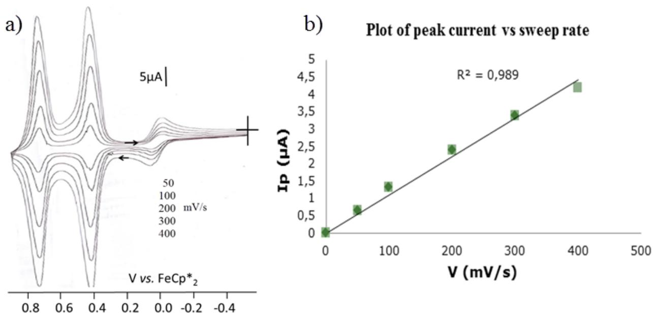
Figure 17: a) Modified Pt electrode of polymer **14** at various scan rates in a DCM solution containing only 0.1 M  $[n\text{-Bu}_4\text{N}][\text{PF}_6]$  as the supporting electrolyte; b) intensity as a function of scan rate; linearity shows the expected behavior of an adsorbed polymer.
