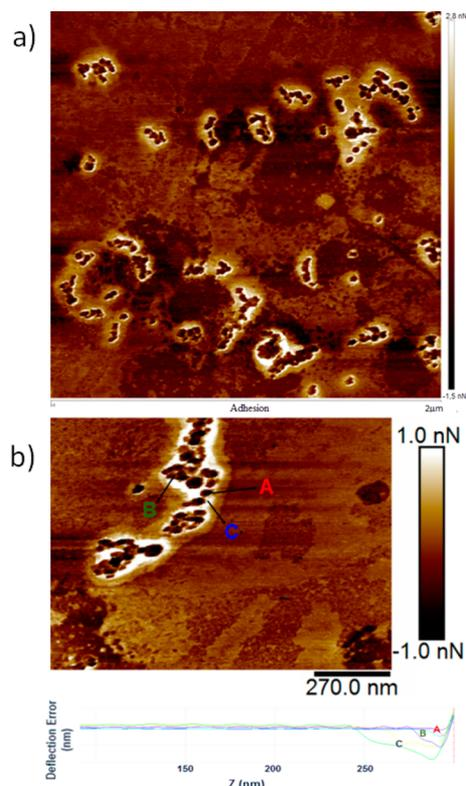
**Figure 4.** AFM adhesion images of biferrocenium chloride polymer-encapsulated AuNPs **8b**: (a) at 2 μm scale, (b) at 270 nm scale at which the force curves of A, B, and C were recorded.
