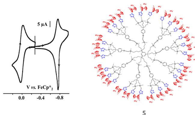
**Figure 3.** CV of **5** in  $\text{CH}_3\text{CN}$ . The wave at 0.0 V corresponds to the internal reference  $\text{FeCp}^*_2$ . Solvent:  $\text{CH}_3\text{CN}$ ; reference electrode: Ag; working and counter electrodes: Pt; scan rate: 0.2 V/s; supporting electrolyte:  $[n\text{-Bu}_4\text{N}][\text{PF}_6]$ .
