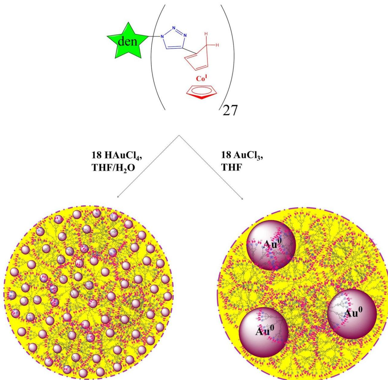
**Figure 6.** Reaction of DHR 5 with H<sub>2</sub>AuCl<sub>4</sub> and AuCl<sub>3</sub> yielding capsules containing AuNPs-8 and AuNPs-9 respectively.
