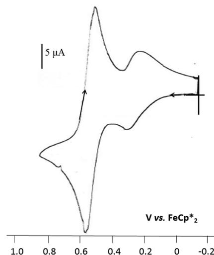
**Figure 1.** CV of 17 in CH<sub>2</sub>Cl<sub>2</sub> solution. Conditions: reference electrode, Ag; working and counter electrodes, Pt; scan rate, 0.2 V/s; supporting electrolyte, [*n*-Bu<sub>4</sub>N][PF<sub>6</sub>].
