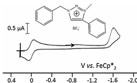
Figure 3. CV of **6** in  $\text{CH}_3\text{CN}$ . The wave at 0.0 V corresponds to the internal reference of  $\text{FeCp}^*_2$ . Solvent:  $\text{CH}_3\text{CN}$ ; reference electrode: Ag; working and counter electrodes: Pt; scan rate:  $0.2 \text{ V s}^{-1}$ ; supporting electrolyte:  $[n\text{Bu}_4\text{N}][\text{PF}_6]$ .
