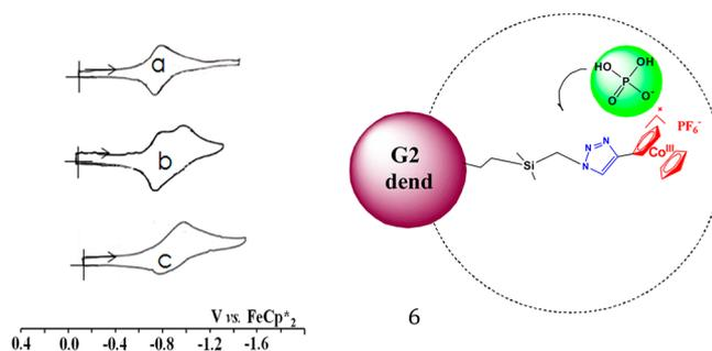
**Figure 6.** CVs of compound **6**: (a) In DMF,  $[\text{n-Bu}_4\text{N}][\text{PF}_6]$  0.1M; see Table 2 for data and conditions; (b) splitting of the reduction CV wave upon addition of  $\text{Bu}_4\text{NH}_2\text{PO}_4$ ; (c) complete disappearance of the first wave upon addition of  $\text{Bu}_4\text{NH}_2\text{PO}_4$ .
