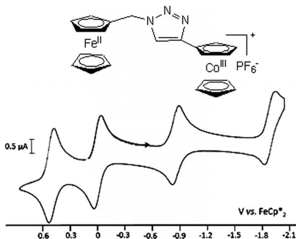
Figure 2. CV of **7** in THF. The wave at 0.0 V corresponds to the internal reference of  $\text{FeCp}^*_2$ . Solvent: THF; reference electrode, Ag; working and counter electrodes: Pt; scan rate:  $0.2 \text{ V s}^{-1}$ ; supporting electrolyte:  $[n\text{Bu}_4\text{N}][\text{PF}_6]$ .
