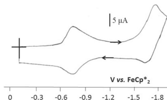
**Fig. 4** CV of **4**. Internal reference:  $\text{FeCp}^*_2$ . Solvent: DMF; 298 K; reference electrode: Ag; working and counter electrodes: Pt; scan rate:  $0.2$   $\text{V/s}^{-1}$ ; supporting electrolyte:  $[\text{n-Bu}_4\text{N}][\text{PF}_6]$
