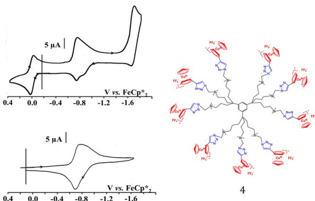
**Figure 4.** CV of **4** in  $\text{CH}_3\text{CN}$ . The wave at 0.0 V corresponds to the internal reference  $\text{FeCp}^*_2$ . Solvent:  $\text{CH}_3\text{CN}$ ; reference electrode: Ag; working and counter electrodes: Pt; scan rate: 0.2 V/s; supporting electrolyte:  $[\text{n-Bu}_4\text{N}][\text{PF}_6]$ .
