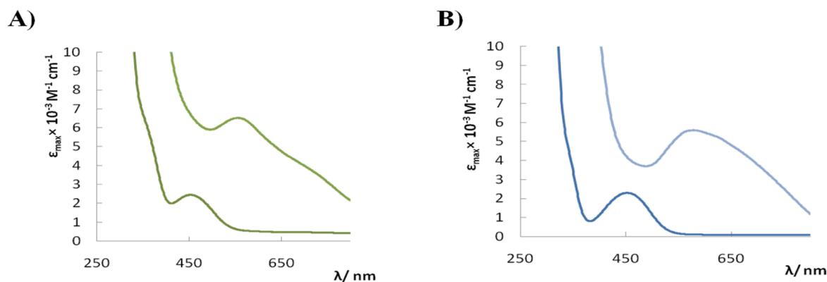
**Figure 4.** (A) Compared UV-vis spectra of **4** and  $4(\text{PF}_6)_3$ :  $\lambda_{\text{max}}$  of **4** = 454 nm (deep green);  $\lambda_{\text{max}}$  of  $4(\text{PF}_6)_3$  = 555 nm (light green). (B) Compared UV-vis spectra of **4** and  $4(\text{BAr}_4^{\text{F}})_3$ :  $\lambda_{\text{max}}$  of **4** = 454 nm (deep blue);  $\lambda_{\text{max}}$  of  $4(\text{BAr}_4^{\text{F}})_3$  = 565 nm (light blue).
