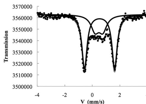
**Figure 2.** Mössbauer spectrum of **6** at zero field and 78 K showing the localized class II mixed valency at 10<sup>7</sup> s<sup>-1</sup> with both ferrocenyl (doublet I.S. = 0.536 mm s<sup>-1</sup> vs. Fe; Q.S. = 2.192 mm s<sup>-1</sup>) and ferricenium groups (doublet I.S. = 0.490 mm s<sup>-1</sup> vs. Fe; Q.S. = 0.571 mm s<sup>-1</sup>).
