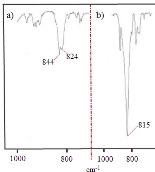
**Figure 13.** FT-IR (KBr) of a) mixed-valent biferrrocenium-stabilized AuNSs **14b**,  $844\text{ cm}^{-1}$  ( $\nu_{\text{Fc}^+}$ ) and  $824\text{ cm}^{-1}$  ( $\nu_{\text{Fc}}$ ), b) polymer **14**,  $815\text{ cm}^{-1}$  ( $\nu_{\text{Fc}}$ ).
