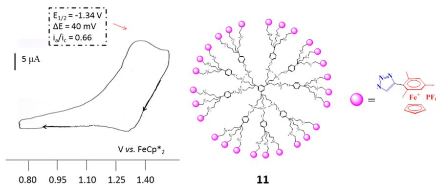
**Figure 3.** CV of dendrimer **11** in DMF under  $N_2$ . Internal reference,  $FeCp^*_2$ ; reference electrode, Ag; working and counter electrodes, Pt; scan rate, 0.2 V/s; supporting electrolyte,  $[n-Bu_4N][PF_6]$ .
