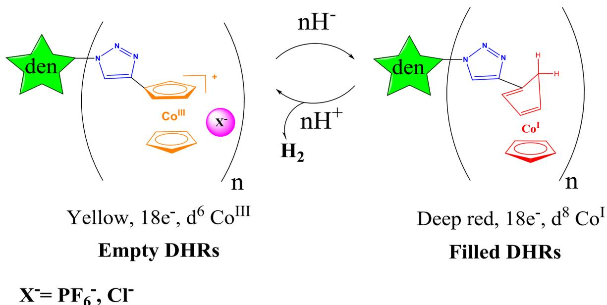
**Figure 2.** Schematic hydride addition/abstraction reversibility between empty DHRs **1**(PF<sub>6</sub><sup>-</sup>) (G<sub>0</sub>), **2**(PF<sub>6</sub><sup>-</sup>) (G<sub>1</sub>) and **3**(PF<sub>6</sub><sup>-</sup>) (G<sub>2</sub>) and filled DHRs **4** (G<sub>0</sub>), **5** (G<sub>1</sub>) and **6** (G<sub>2</sub>). Addition of HCl to filled DHRs **4**, **5** and **6** also leads to empty DHRs **1**(Cl<sup>-</sup>), **2**(Cl<sup>-</sup>) and **3**(Cl<sup>-</sup>) respectively.
