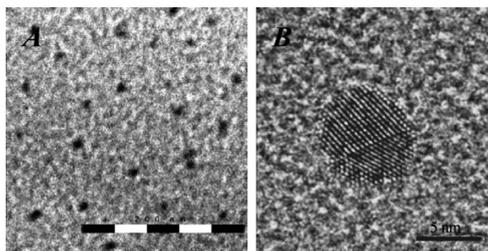
**FIGURE 3.** (a) TEM of the dendrimer **15** + 1 equiv of  $\text{HAuCl}_4$  reduced by  $[\text{Fe}^{\text{I}}\text{Cp}(\eta^6\text{-C}_6\text{Me}_6)]$  and (b) HRTEM of the dendrimer **15** + 1 equiv of  $\text{HAuCl}_4$  reduced by  $[\text{Fe}^{\text{I}}\text{Cp}(\eta^6\text{-C}_6\text{Me}_6)]$ .
