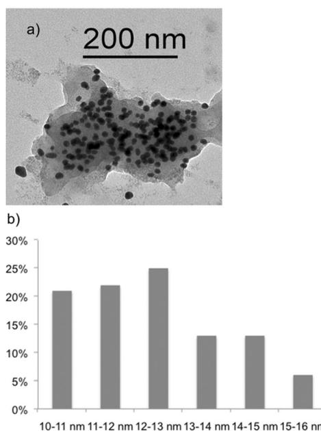
**Figure 4.** a) TEM image of Au NPs synthesized by reduction of Au<sup>III</sup> with **5**. b) Size distribution of the Au NPs present in the TEM picture (average size of 98 Au NPs: (12 ± 2) nm).
