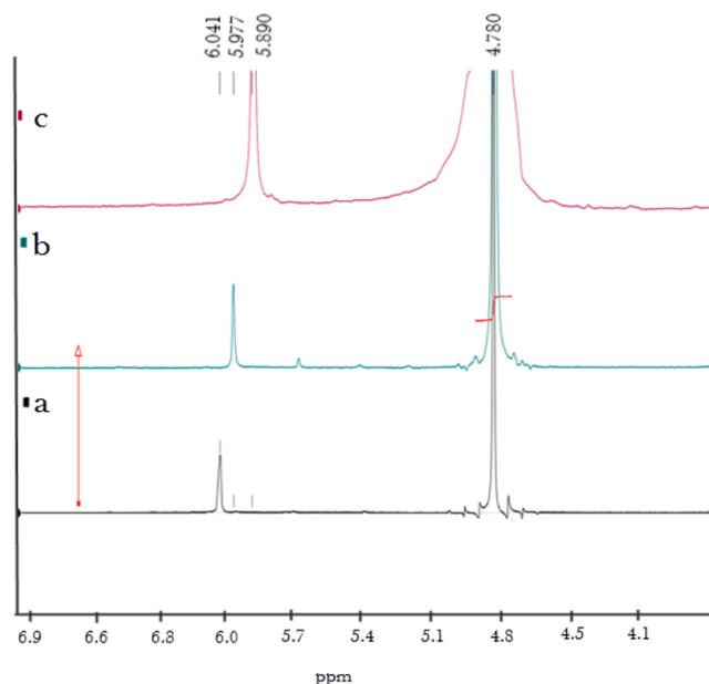
**Figure 1.** Comparative  $^1\text{H}$  NMR spectra in  $\text{D}_2\text{O}$  of  $[\text{RhCp}(\text{Cl})_2]_n$  (**3**),  $[\text{RhCp}_2][\text{Cl}]$  (**4**), and  $[\text{RhCp}_2][\text{PF}_6]$  (**5**): (a) **3**,  $\delta$  6.04 ppm (10H, Cp); (b) **4**,  $\delta$  5.98 ppm (10H, Cp); (c) **5**,  $\delta$  5.89 ppm (10H, Cp).
