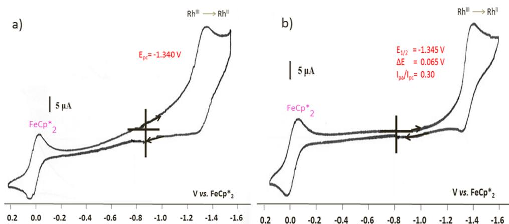
**Figure 3.** Cyclic voltammetry of [RhCp<sub>2</sub>][BAr<sub>4</sub><sup>F</sup>] (6) in THF at (a) 22 °C and (b) –50 °C. The wave at 0.0 V corresponds to the internal reference [FeCp\*<sub>2</sub>].<sup>22</sup> Conditions: reference electrode, Ag; working and counter electrodes, Pt; scan rate, 0.05 V/s; supporting electrolyte, [*n*-Bu<sub>4</sub>N][BAr<sub>4</sub><sup>F</sup>].
