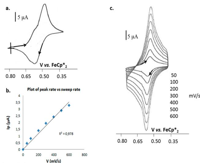
**Figure 3.** Cyclic voltammograms of **16** in  $\text{CH}_2\text{Cl}_2$  solution containing 0.1 M  $[\text{n-Bu}_4\text{N}][\text{PF}_6]$ : (a) in solution; (b) intensity as a function of scan rate (linearity shows the expected behavior of an adsorbed dendrimer); (c) modified Pt electrode at various scan rates in  $\text{CH}_2\text{Cl}_2$  (solution containing only the supporting electrolyte).
