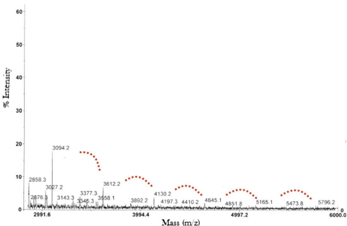
**Fig. 3** MALDI-TOF mass spectrum of polymer **4**
