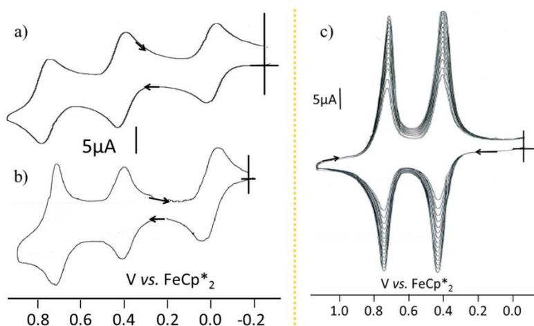
**Figure 2.** CVs of a) monomer **7**, b) polymer **9** and c) progressive adsorption of polymer **9** onto a Pt electrode upon 20 scans around the BiFc potentials. Solvent: DCM ; reference electrode : Ag ; working and counter electrodes: Pt ; scan rate: 0.2 V/s; supporting electrolyte: 0.1 M  $[n\text{-Bu}_4\text{N}][\text{PF}_6]$ . The wave at 0.0V belongs to the internal reference  $\text{FeCp}^*_2$ .
