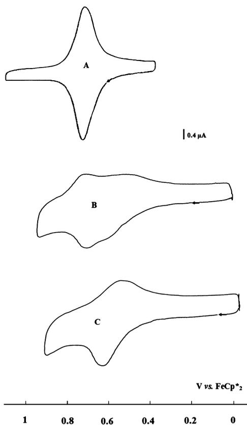
**Figure 11.** CVs for the titration of  $[n\text{-Bu}_4\text{N}]_2[\text{ATP}]$  by the Pt electrode modified with the copolymer  $10^{100/50}$  in DCM at 20 °C: (A) before addition of  $[n\text{-Bu}_4\text{N}]_2[\text{ATP}]$ ; (B) during addition of  $[n\text{-Bu}_4\text{N}]_2[\text{ATP}]$ ; (C) after addition of excess  $[n\text{-Bu}_4\text{N}]_2[\text{ATP}]$ .
