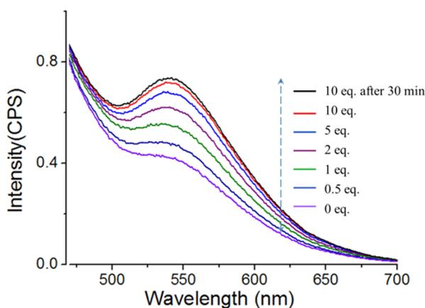
**Figure 6.** Fluorescent emission spectra of AuNP-3 mixed with various amounts of Hcy (1 equiv of analyte = 0.05 mM in the solution;  $\lambda_{\text{ex}}$  = 405 nm; standard quartz cuvette; path length = 1 cm, recorded at 25 °C; see full-scale spectra in Figure S12 in the SI).
