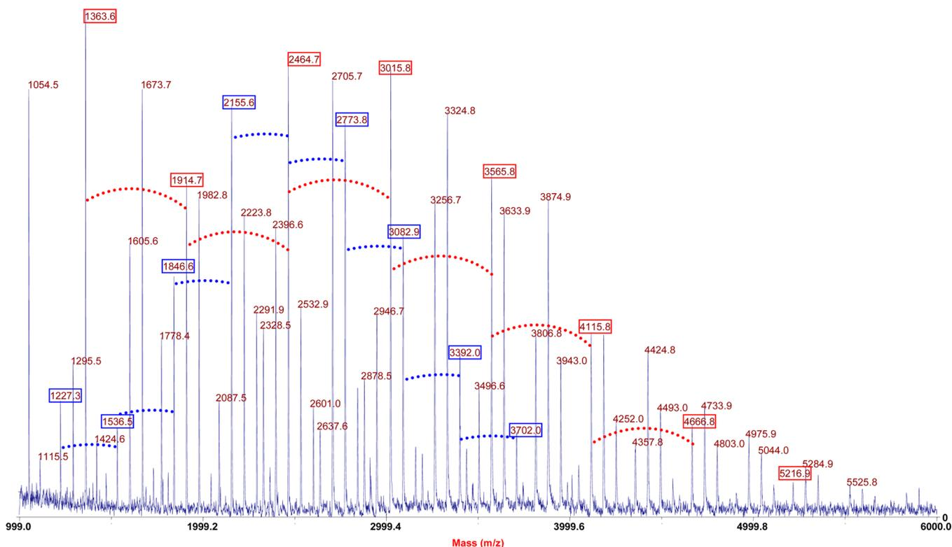
**Figure 9.** MALDI-TOF MS spectrum of the copolymer  $10^{6/3}$ . The molar feed ratio of monomers **8** and **5** to **1** is 6:3:1. The dotted red and blue lines correspond to the difference between molecular peaks of  $550 \pm 1$  (MW of **5**) and  $309 \pm 1$  Da (MW of **8**), respectively.
