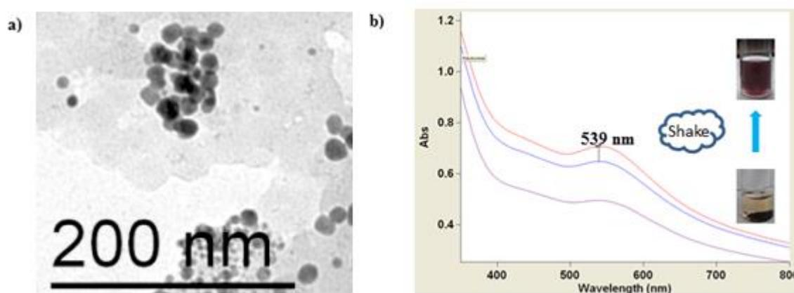
**Figure 12.** a) TEM of AuNPs-14c and b) UV-vis. spectrum of **14c** (blue line). The violet line corresponds to the UV-vis. spectrum after 5 min and the red line is recorded after shaking of the sample. The photograph shows the flocculated AuNPs and their redissolution by shaking.
