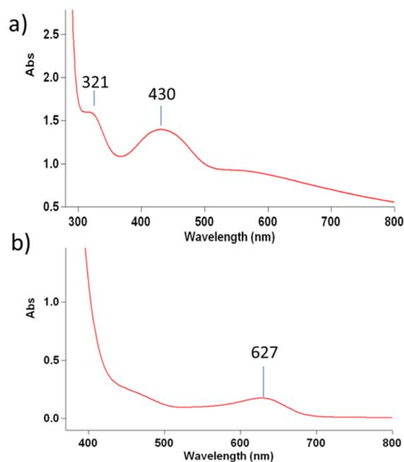
**Figure 2.** UV-vis spectra revealing the characteristic bands of (a) the Fc group in **AuNP-1** (321 and 430 nm) and (b) the ferricenium group in **AuNP-2** (627 nm) (both were recorded in an EtOH solution).
