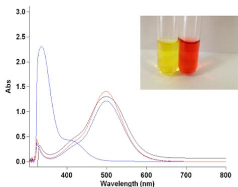
Figure 3. Compared UV–vis spectra of **1** (blue line), cobaltocenium–enamine monomer **4** (red line), cobaltocenium–enamine polymer **5** (black line) and cobaltocenium–enamine polymer **8** (violet line) in acetone. The inset photograph shows the color of **1** (left) and the cobaltocenium–enamine norbornene polymers **5** (right) in acetone.
