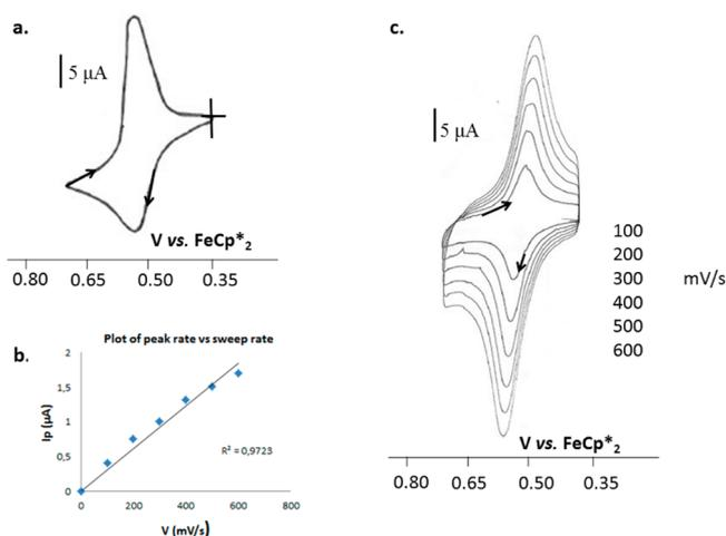
**Figure 2.** Cyclic voltammograms of **14** in  $\text{CH}_2\text{Cl}_2$  solution containing 0.1 M  $[\text{n-Bu}_4\text{N}][\text{PF}_6]$ : (a) in solution; (b) intensity as a function of scan rate (linearity shows the expected behavior of an adsorbed dendrimer); (c) modified Pt electrode at various scan rates in a  $\text{CH}_2\text{Cl}_2$  solution (containing only the supporting electrolyte).
