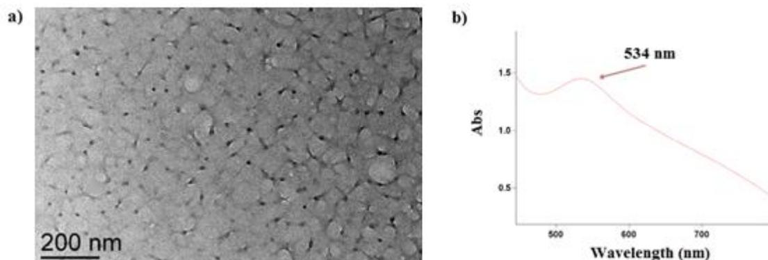
**Figure 14.** a) TEM analysis of AuNNs-**18b** at 200 nm, b) UV-vis. spectrum of AuNNs-**18b** peaking at 534 nm (plasmon band).
