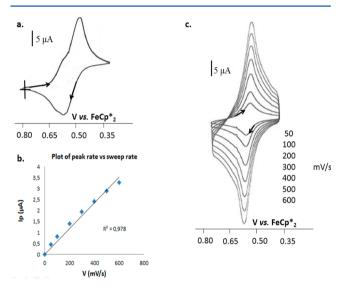
**Figure 3.** Cyclic voltammograms of **16** in  $CH_2Cl_2$  solution containing 0.1 M  $[n\text{-Bu}_4N][PF_6]$ : (a) in solution; (b) intensity as a function of scan rate (linearity shows the expected behavior of an absorbed dendrimer); (c) modified Pt electrode at various scan rates in  $CH_2Cl_2$  (solution containing only the supporting electrolyte).
