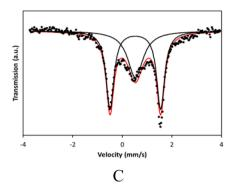
Figure 5. Mössbauer spectra of 4(PF<sub>6</sub>)<sub>3</sub> (A), 5(BAr<sub>4</sub><sup>F</sup>)<sub>2</sub> (B), and 11(BAr<sub>4</sub><sup>F</sup>) (C) at zero field and 78 K.
