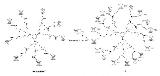
Scheme 5. Synthesis of the bimetallic dendrimer 12 by hydroamination reaction of 1 with nona-NHFc# (Fc# = octamethylferrocenyl).
