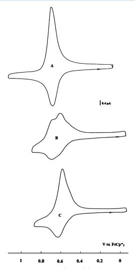
**Figure 5.** CVs for the titration of  $[n\text{-Bu}_4N]_2[ATP]$  with polymer  $6^{50}$  in CH<sub>2</sub>Cl<sub>2</sub> at 20 °C by adding the salt of the anion to the polymer solution: (A) before addition of  $[n\text{-Bu}_4N]_2[ATP]$ ; (B) during the titration with 0.25 equiv of  $[n\text{-Bu}_4N]_2[ATP]$ ; (C) with 0.5 equiv of  $[n\text{-Bu}_4N]_2[ATP]$ .
