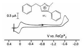
Figure 3. CV of **6** in CH<sub>3</sub>CN. The wave at 0.0 V corresponds to the internal reference of FeCp\*<sub>2</sub>. Solvent: CH<sub>3</sub>CN; reference electrode: Ag; working and counter electrodes: Pt; scan rate: 0.2 V s<sup>-1</sup>; supporting electrolyte: [nBu<sub>4</sub>N][PF<sub>6</sub>].
