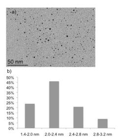
**Figure 3.** a) TEM image of Pd NPs stabilized by **5**. b) Size distribution of the Pd NPs present in the TEM picture (average size of 103 Pd NPs:  $(2.3 \pm 0.6)$  nm).
