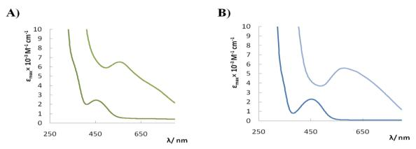
Figure 4. (A) Compared UV-vis spectra of 4 and  $4(PF_6)_3$ :  $\lambda_{max}$  of 4 = 454 nm (deep green);  $\lambda_{max}$  of  $4(PF_6)_3 = 555$  nm (light green). (B) Compared UV-vis spectra of 4 and  $4(BAr_4^F)_3$ :  $\lambda_{max}$  of 4 = 454 nm (deep blue);  $\lambda_{max}$  of  $4(BAr_4^F)_3 = 565$  nm (light blue).
