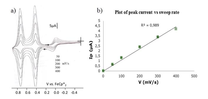
Figure 17: a) Modified Pt electrode of polymer **14** at various scan rates in a DCM solution containing only  $0.1 \text{ M} [n\text{-Bu}_4\text{N}][PF_6]$  as the supporting electrolyte; b) intensity as a function of scan rate; linearity shows the expected behavior of an adsorbed polymer.
