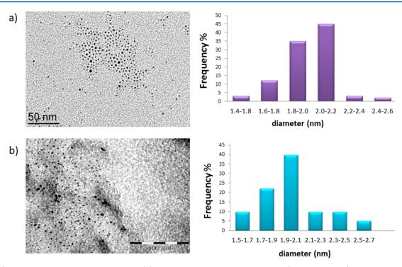
Figure 2. (a) TEM and size distribution of AuNPs 17; (b) TEM and size distribution of AuNPs 18 (bar scale: 100 nm).
