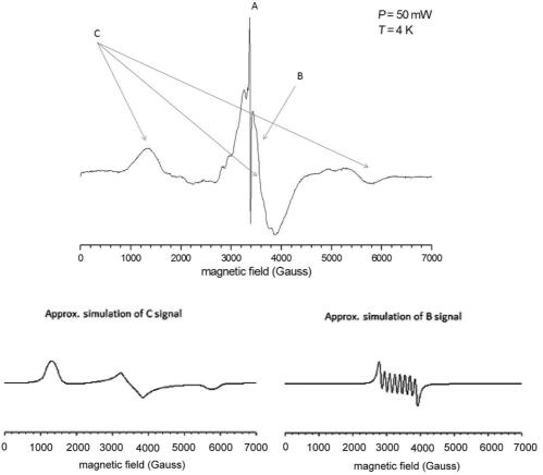
Figure 4. EPR analysis of **9** and approximate simulations of signals B and  $C^{[62]}$ . Signal A gives  $g_{\parallel} = 2.037$  and  $g_{\perp} = 2.003$ . Signal B gives g = 2.015 and the hyperfine coupling constant A (Co – I = 7/2) = 150 G. The g values of signal C are  $g_1 = 1.17$ ,  $g_2 = 1.9$ , and  $g_3 = 5.09$ .
