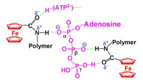
**Figure 6.** Hydrogen-bonding interactions between ATP<sup>2-</sup> and two amidoferrocenyl groups of polymers **6**.
