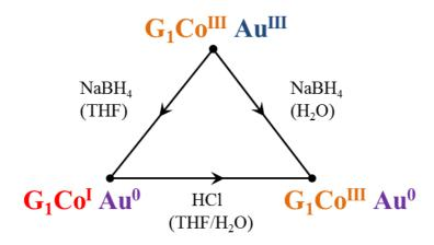
**Figure 7.** Reduction of  $G_1Co^{III}Au^{III}$  by NaBH<sub>4</sub> leading to the selective reduction of either  $Co^{III}$  (**AuNPs-10**) or  $Au^{III}$  (**AuNPs-11**) and selective oxidation of  $G_1Co^IAu^0$  (**AuNPs-11**) back to  $G_1Co^{III}Au^0$  (**AuNPs-12**).
