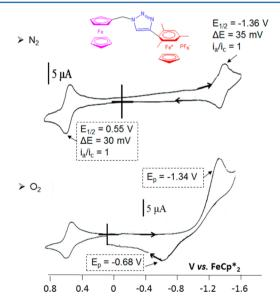
Figure 1. CVs of 5 under  $N_2$  and under  $O_2$  (air). Solvent, DMF; reference electrode, Ag; working and counter electrodes, Pt; scan rate, 0.2 V/s; and supporting electrolyte,  $[n\text{-Bu}_4N][PF_6]$ , 0.1M.
