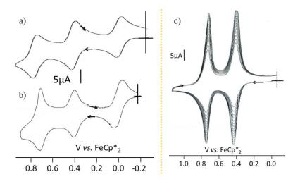
**Figure 2**. CVs of a) monomer **7**, b) polymer **9** and c) progressive adsorption of polymer **9** onto a Pt electrode upon 20 scans around the BiFc potentials. Solvent: DCM; reference electrode: Ag; working and counter electrodes: Pt; scan rate: 0.2 V/s; supporting electrolyte: 0.1 M [*n*-Bu<sub>4</sub>N][PF<sub>6</sub>]. The wave at 0.0V belongs to the internal reference FeCp\*<sub>2</sub>.
