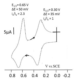
**Figure 18**. Voltammetric response of a platinum electrode modified with polymer **14**, measured in  $H_2O/0.1$  M NaCl; scan rate: 50 mV s<sup>-1</sup>.
