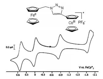
Figure 2. CV of 7 in THF. The wave at 0.0 V corresponds to the internal reference of FeCp\*<sub>2</sub>. Solvent: THF; reference electrode, Ag; working and counter electrodes: Pt; scan rate:  $0.2 \text{ V s}^{-1}$ ; supporting electrolyte:  $[nBu_4N][PF_6]$ .
