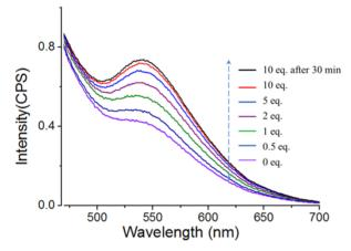
**Figure 6.** Fluorescent emission spectra of **AuNP-3** mixed with various amounts of Hcy (1 equiv of analyte = 0.05 mM in the solution;  $\lambda_{\rm ex}$  = 405 nm; standard quartz cuvette; path length = 1 cm, recorded at 25 °C; see full-scale spectra in Figure S12 in the SI).
