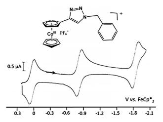
Figure 1. CV of 1 in THF. The wave at 0.0 V corresponds to the internal reference FeCp\*<sub>2</sub>. Solvent: THF; reference electrode: Ag; working and counter electrodes: Pt; scan rate: 0.2 V s<sup>-1</sup>; supporting electrolyte: [nBu<sub>4</sub>N][PF<sub>6</sub>].
