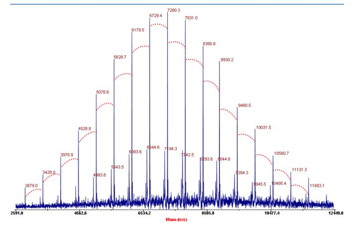
Figure 3. MALDI-TOF MS spectrum of polymer  $6^{16}$ . The molar feed ratio of monomer 5 to 1 is 16:1. The red dotted lines correspond to the difference between molecular peaks of a value of  $550 \pm 1$  Da (MW of 5).
