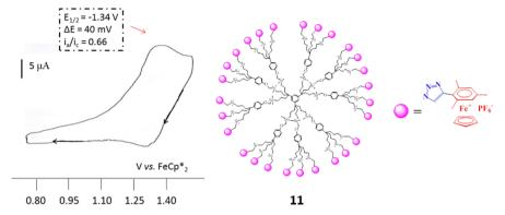
Figure 3. CV of dendrimer 11 in DMF under  $N_2$ . Internal reference, FeCp\*2; reference electrode, Ag; working and counter electrodes, Pt; scan rate, 0.2 V/s; supporting electrolyte,  $[n\text{-Bu}_4N][PF_6]$ .
