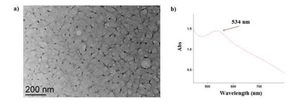
**Figure 14**. a) TEM analysis of AuNNs-**18b** at 200 nm, b) UV-vis. spectrum of AuNNs-**18b** peaking at 534 nm (plasmon band).
