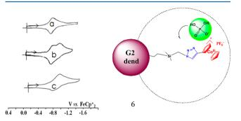
Figure 6. CVs of compound 6: (a) In DMF,  $[n\text{-}Bu_4N][PF_6]$  0.1M; see Table 2 for data and conditions; (b) splitting of the reduction CV wave upon addition of  $Bu_4NH_2PO_4$ ; (c) complete disappearance of the first wave upon addition of  $Bu_4NH_2PO_4$ .
