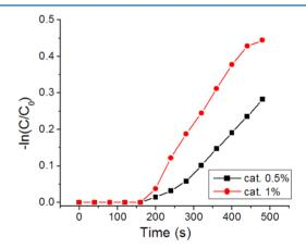
**Figure 4.** Plots of the decreasing rate of 4-NP  $[-\ln(C/C_0)]$  versus the reaction times using two distinct amounts of catalyst **AuNP-2** (0.5% catalyst in the black curve and 1% catalyst in the red curve).
