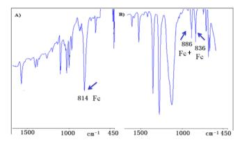
**Figure 3.** FT-IR spectra in KBr pellets of (A) 4, 814 cm<sup>-1</sup> ( $\nu_{Fc}$ ) and (B) 4(BAr<sub>4</sub><sup>F</sup>)<sub>3</sub>, 886 cm<sup>-1</sup> ( $\nu_{Fc}$ +), 836 cm<sup>-1</sup> ( $\nu_{Fc}$ ), where Fc stands for [Fe( $\eta^5$ -C<sub>5</sub>H<sub>5</sub>)( $\eta^5$ -C<sub>5</sub>H<sub>4</sub>-)].
