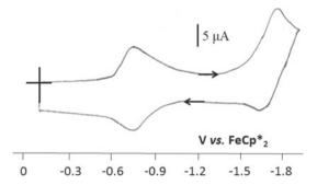
**Fig. 4** CV of **4**. Internal reference: FeCp\*<sub>2</sub>. Solvent: DMF; 298 K; reference electrode: Ag; working and counter electrodes: Pt; scan rate:  $0.2 \text{ V/s}^{-1}$ ; supporting electrolyte:  $[n\text{-Bu}_4\text{N}][\text{PF}_6]$
