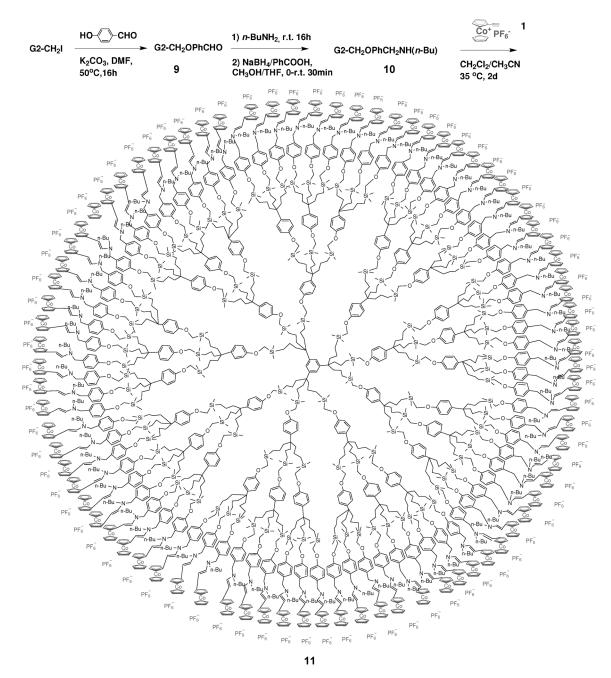
Scheme 4. Synthesis of dendrimer G2-9 by Williamson reaction with G2-CH<sub>2</sub>I (81 branches) and 4-hydroxybenzaldehyde; synthesis of the G2 dendrimer 10 terminated with 81 secondary amine groups and hydroamination of 1 with dendrimer 10 giving the all-trans-enamine-cobaltocenium dendrimer 11.
