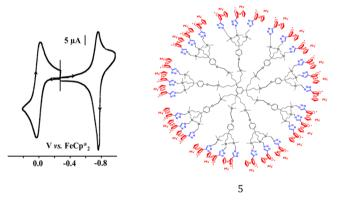
Figure 3. CV of 5 in CH<sub>3</sub>CN. The wave at 0.0 V corresponds to the internal reference FeCp\*<sub>2</sub>. Solvent: CH<sub>3</sub>CN; reference electrode: Ag; working and counter electrodes: Pt; scan rate: 0.2 V/s; supporting electrolyte:  $[n\text{-Bu}_4\text{N}][\text{PF}_6]$ .
