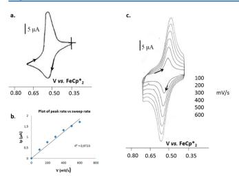
**Figure 2.** Cyclic voltammograms of **14** in  $CH_2Cl_2$  solution containing 0.1 M  $[n\text{-Bu}_4N][PF_6]$ : (a) in solution; (b) intensity as a function of scan rate (linearity shows the expected behavior of an absorbed dendrimer); (c) modified Pt electrode at various scan rates in a  $CH_2Cl_2$  solution (containing only the supporting electrolyte).
