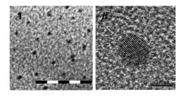
**FIGURE 3.** (a) TEM of the dendrimer **15** + 1 equiv of HAuCl<sub>4</sub> reduced by  $[Fe^{I}Cp(\eta^{6}-C_{6}Me_{6})]$  and (b) HRTEM of the dendrimer **15** + 1 equiv of HAuCl<sub>4</sub> reduced by  $[Fe^{I}Cp(\eta^{6}-C_{6}Me_{6})]$ .
