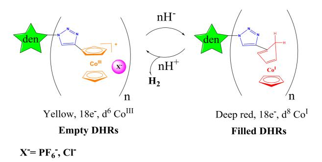
**Figure 2.** Schematic hydride addition/abstraction reversibility between empty DHRs  $\mathbf{1(PF_6)}$   $(G_0)$ ,  $\mathbf{2(PF_6)}$   $(G_1)$  and  $\mathbf{3(PF_6)}$   $(G_2)$  and filled DHRs  $\mathbf{4}$   $(G_0)$ ,  $\mathbf{5}$   $(G_1)$  and  $\mathbf{6}$   $(G_2)$ . Addition of HCl to filled DHRs  $\mathbf{4}$ ,  $\mathbf{5}$  and  $\mathbf{6}$  also leads to empty DHRs  $\mathbf{1(Cl)}$ ,  $\mathbf{2(Cl)}$  and  $\mathbf{3(Cl)}$  respectively.
