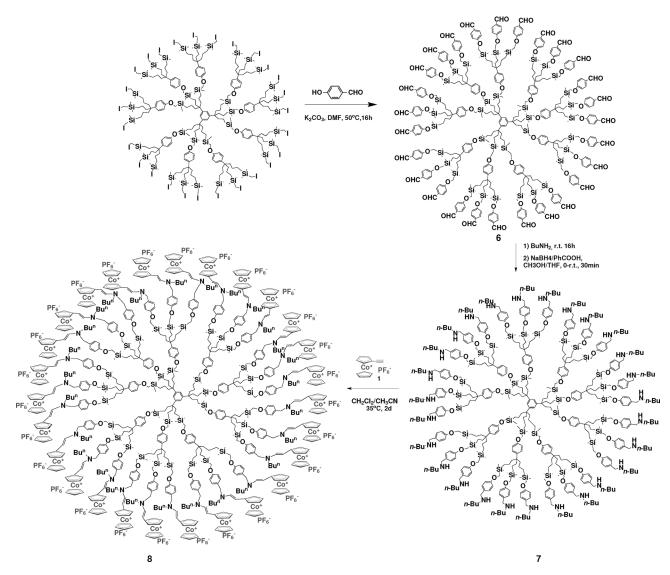
Scheme 3. Synthesis of dendrimer G1-6 by Williamson reaction between G1-CH<sub>2</sub>I (27 branches) and 4-hydroxybenzaldehyde; synthesis of the dendrimer 7 and hydroamination of 1 with dendrimer 7 giving the all-*trans*-enamine-cobalticenium dendrimer 8.
