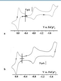
**Figure 5.** (a) CV of 4 in DMF. (b) CV of 5 in DMF. The wave at 0.0 V corresponds to the internal reference FeCp\*<sub>2</sub>. Solvent: DMF; reference electrode: Ag; working and counter electrodes: Pt; scan rate: 0.2 V/s; supporting electrolyte:  $[n\text{-Bu}_4\text{N}][\text{PF}_6]$ .
