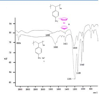
Figure 4. Comparative IR spectra of polymers 7 and 8.
