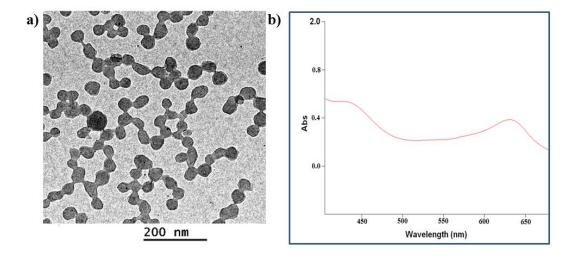
**Figure 16.** a) TEM analysis of **AgNSs-21b**, b) UV-vis. spectrum of **AgNSs-21b** showing the plasmon band of AgNPs at  $\lambda$ = 434 nm and the biferrocenium band at  $\lambda$  = 630 nm.
