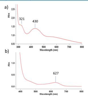
**Figure 2.** UV—vis spectra revealing the characteristic bands of (a) the Fc group in **AuNP-1** (321 and 430 nm) and (b) the ferricenium group in **AuNP-2** (627 nm) (both were recorded in an EtOH solution).
