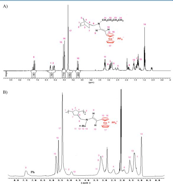
Figure 1. <sup>1</sup>H NMR spectra of the cobalticenium-enamine monomer 4 (A) and homopolymer 5 in CD<sub>3</sub>COCD<sub>3</sub> (B).
