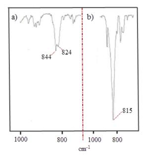
**Figure 13.** FT-IR (KBr) of a) mixed-valent biferrocenium-stabilized AuNSs **14b**, 844 cm<sup>-1</sup> ( $v_{Fc}$ +) and 824 cm<sup>-1</sup> ( $v_{Fc}$ ), b) polymer **14**, 815 cm<sup>-1</sup> ( $v_{Fc}$ ).
