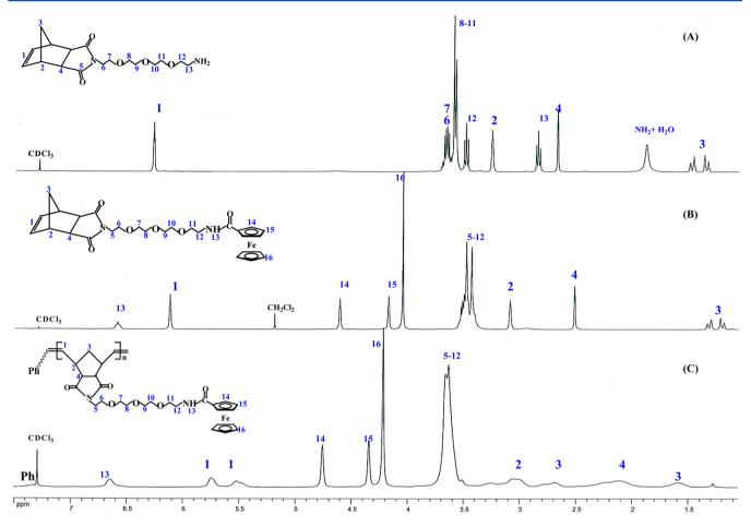
Figure 2. <sup>1</sup>H NMR spectra of 4 (A), monomer 5 (B), and polymer 6 (C) in CDCl<sub>3</sub>.
