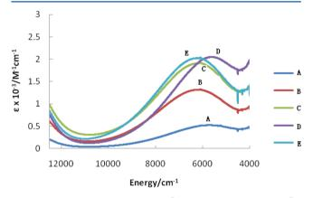
**Figure 6.** Near-IR spectra of  $11(BAr_4^F)$  (A),  $4(PF_6)_3$  (B),  $4(BAr_4^F)_3$  (C),  $5(BAr_4^F)_2$  (D), and  $7(BAr_4^F)_4$  (E) in  $CD_3COCD_3$ .
