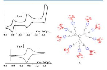
**Figure 4.** CV of **4** in CH<sub>3</sub>CN. The wave at 0.0 V corresponds to the internal reference FeCp\*<sub>2</sub>. Solvent: CH<sub>3</sub>CN; reference electrode: Ag; working and counter electrodes: Pt; scan rate: 0.2 V/s; supporting electrolyte:  $[n\text{-Bu}_4\text{N}][\text{PF}_6]$ .
