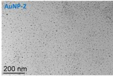
Figure 3. TEM images of AuNP-1 (d = 5 nm) and AuNP-2 (d = 4.4 nm) prepared using two distinct methods.
