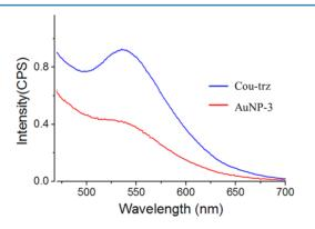
**Figure 5.** Fluorescent emission spectra of Cou-trz (0.2 mM) and Cou-trz-capped **AuNP-3** (both in a DMSO/water solution;  $\lambda_{\rm ex}$  = 405 nm, recorded at 22 °C).
