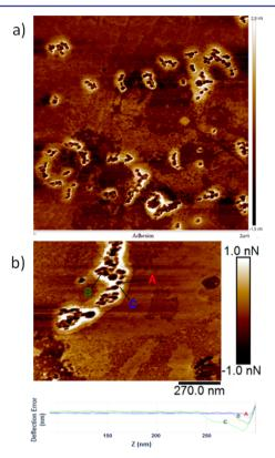
**Figure 4.** AFM adhesion images of biferrocenium chloride polymerencapsulated AuNPs **8b**: (a) at 2  $\mu$ m scale, (b) at 270 nm scale at which the force curves of A, B, and C were recorded.
