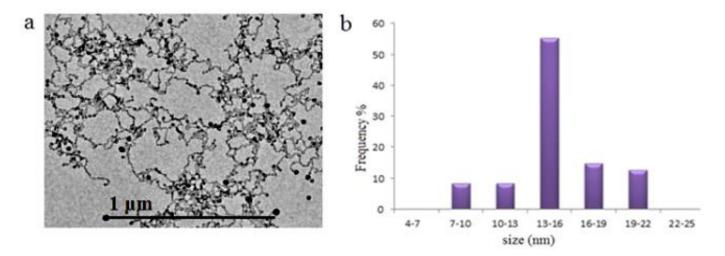
**Figure 10**: a) TEM analysis of mixed-valent biferrocenium polymer-stabilized AuNSs-**14b** at 0.5 μm; b) size distribution of AuNSs.
