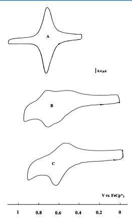
**Figure 11.** CVs for the titration of  $[n\text{-Bu}_4\mathrm{N}]_2[\mathrm{ATP}]$  by the Pt electrode modified with the copolymer  $10^{100/50}$  in DCM at 20 °C: (A) before addition of  $[n\text{-Bu}_4\mathrm{N}]_2[\mathrm{ATP}]$ ; (B) during addition of  $[n\text{-Bu}_4\mathrm{N}]_2[\mathrm{ATP}]$ ; (C) after addition of excess  $[n\text{-Bu}_4\mathrm{N}]_2[\mathrm{ATP}]$ .
