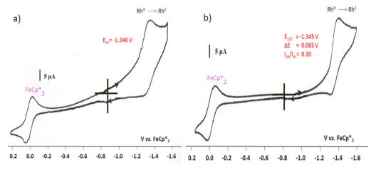
Figure 3. Cyclic voltammetry of  $[RhCp_2][BAr^F_4]$  (6) in THF at (a) 22 °C and (b) -50 °C. The wave at 0.0 V corresponds to the internal reference  $[FeCp^*_2]$ . Conditions: reference electrode, Ag; working and counter electrodes, Pt; scan rate, 0.05 V/s; supporting electrolyte,  $[n-Bu_4N][BAr^F_4]$ .
