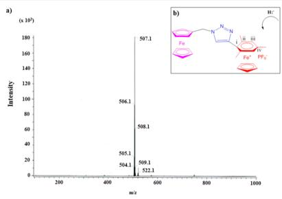
Figure 2. (a) FD-MS of neutral compound 6 and isomers and (b) possible hydride addition on four positions i, ii, iii, and iv of the mesitylene ligand (ii and iv are steroelectronically disfavored).
