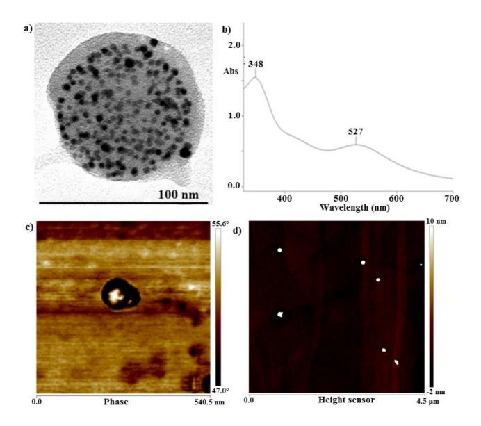
**Figure 4.** a) TEM image of a capsule with **AuNPs-8**, b) UV-vis. spectrum of **AuNPS-8**, c) AFM phase image of a capsule with **AuNPs-8**, d) AFM topology image (height sensor) of **AuNPs-8**.
