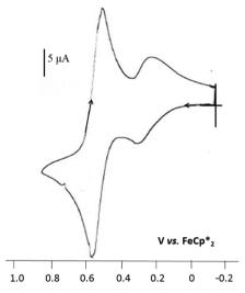
Figure 1. CV of 17 in  $CH_2Cl_2$  solution. Conditions: reference electrode, Ag; working and counter electrodes, Pt; scan rate, 0.2 V/s; supporting electrolyte,  $[n\text{-Bu}_4N][PF_6]$ .
