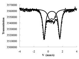
*Figure 2.* Mössbauer spectrum of **6** at zero field and 78 K showing the localized class II mixed valency at  $10^7 \, \text{s}^{-1}$  with both ferrocenyl (doublet l.S. = 0.536 mm s<sup>-1</sup> vs. Fe; Q.S. = 2.192 mm s<sup>-1</sup>) and ferricinium groups (doublet l.S. = 0.490 mm s<sup>-1</sup> vs. Fe; Q.S. = 0.571 mm s<sup>-1</sup>).
