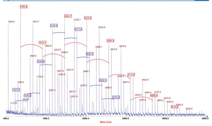
Figure 9. MALDI-TOF MS spectrum of the copolymer  $10^{6/3}$ . The molar feed ratio of monomers 8 and 5 to 1 is 6:3:1. The dotted red and blue lines correspond to the difference between molecular peaks of 550  $\pm$  1 (MW of 5) and 309  $\pm$  1 Da (MW of 8), respectively.
