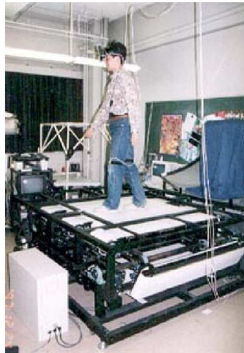
Figure 2.13. La plateforme de locomotion Torus Threadmill — Iwata et al.
