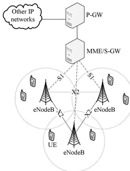
Figure 1.1: LTE/LTE-A system architecture
