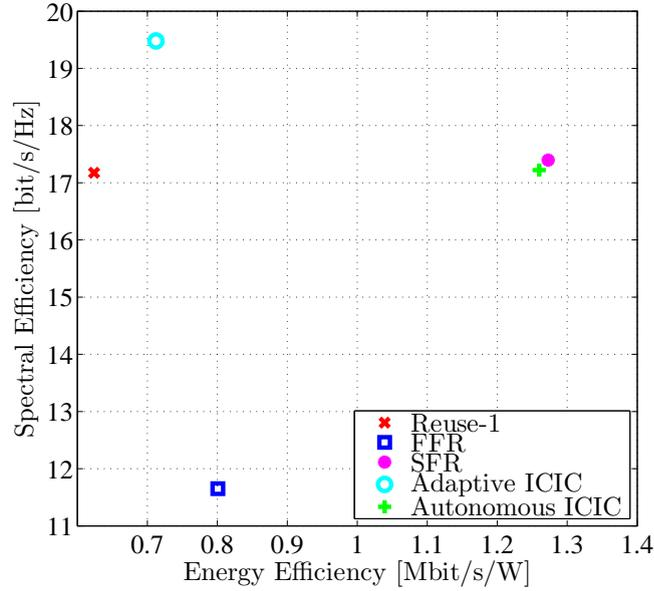
Figure 4.12: Spectral efficiency versus energy efficiency
