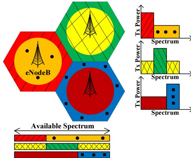
Figure 2.6: Soft frequency reuse technique
