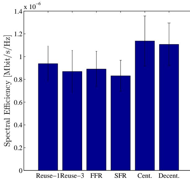
Figure 3.8: Spectral efficiency for several resource allocation approaches
