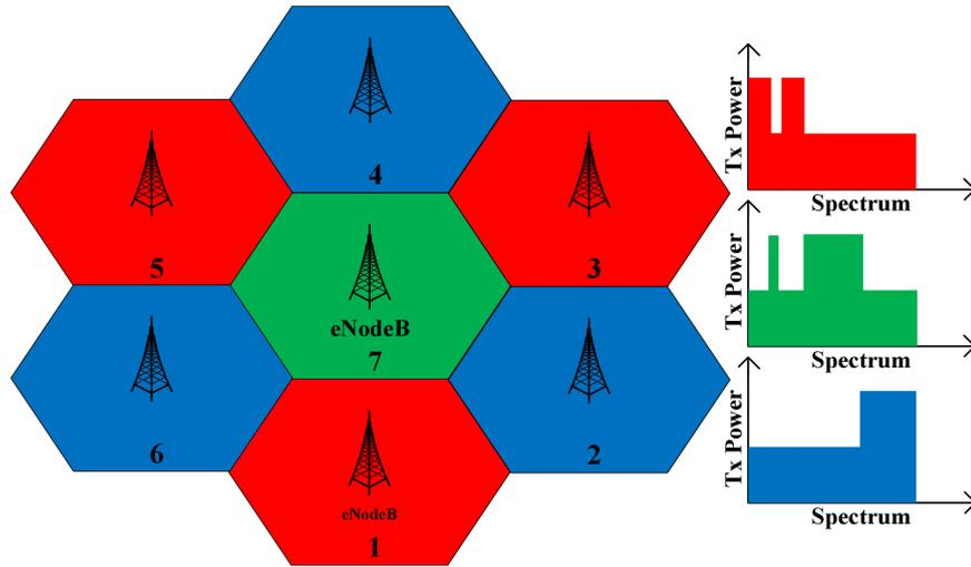
Figure 5.1: LTE/LTE-A network of seven adjacent cells
