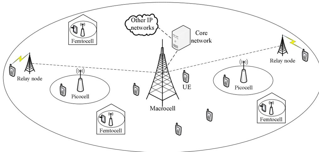
Figure 1.2: LTE/LTE-A macro cell with dense small cell deployment
