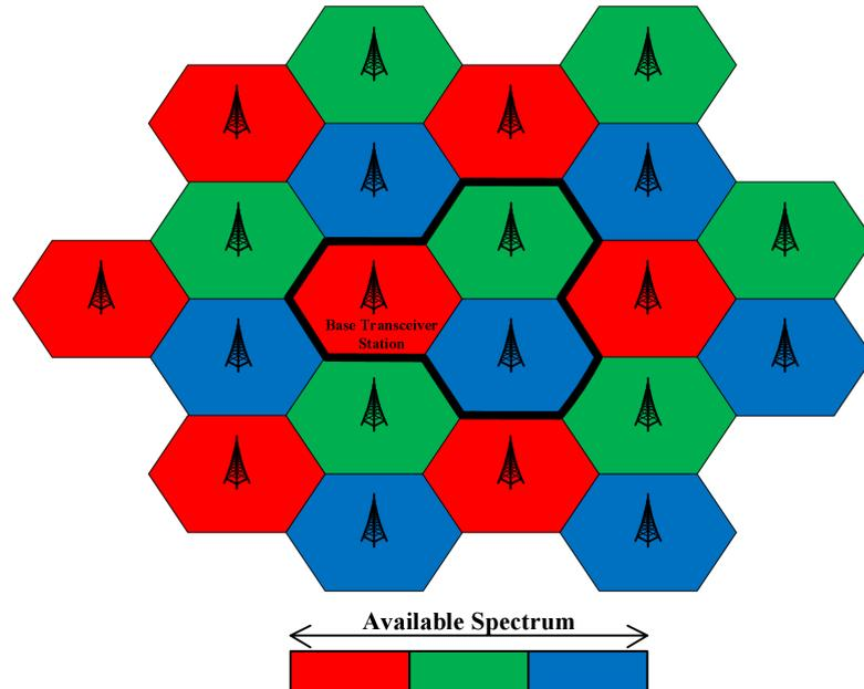
Figure 2.4: The frequency reuse-3 model in GSM
