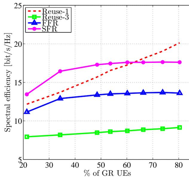
Figure 2.14: Spectral efficiency versus percentage of GR UEs
