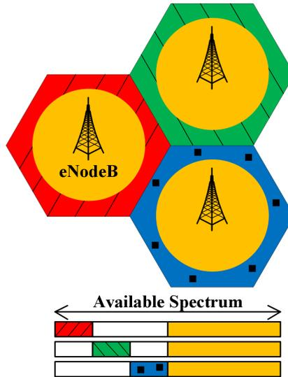
Figure 2.5: Fractional frequency reuse technique
