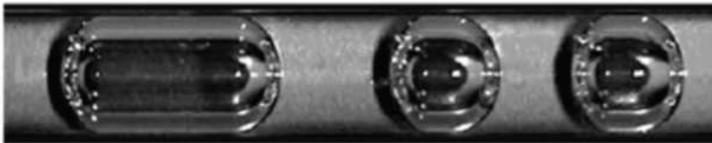
Fig. 2.4: Liquid slug in a PHP ( Khandekar et al. [2.19] ).
