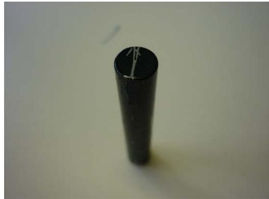
(a) Magnet cylinder with  $B_1$  and  $B_2$  the magnetic field in the vicinity of its two faces and the misalignment angle  $\alpha$ .
