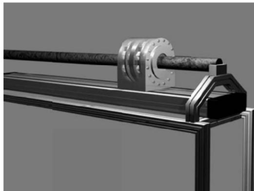
*Figure 2-34: The sliding sensor automatically scans the sample [75].*
