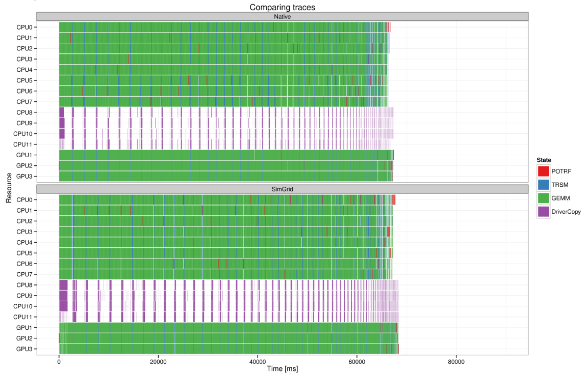
Figure 6.15: Comparing execution traces (native execution on top vs. simulated execution at the bottom) of the Cholesky application with a 72,000 \times 72,000 matrix on the Mirage machine using 8 cores and 3 GPUs as workers. Adding 8 cores, improved the performance by approximately 20% compared to the performances obtained in Figure 6.13.
