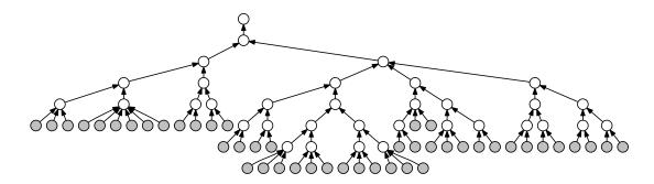
Figure 7.2: Typical elimination tree: each node corresponds to a front and the resulting tree is traversed from the bottom to the top. To reduce the overhead incurred by managing a large number of fronts, subtrees are pruned and aggregated into optimized sequential tasks (Do subtree) depicted in gray.
