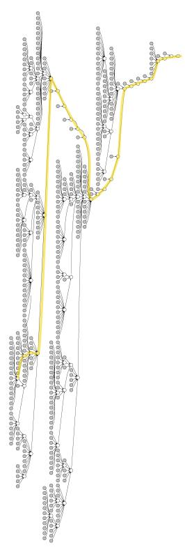
Figure 8.1: Elimination tree for  $cat\_ears\_4\_4$  matrix, rotated for 90 degrees to fit the page. The graph is extremely badly balanced and has a comb-like structure with a huge number of <code>Do\_subtree</code> kernels presented as grey nodes.
