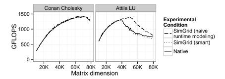
Figure 6.8: Illustrating the influence of modeling runtime. Careless modeling of runtime may be perfectly harmless in some cases, it turns out to be misleading in others.
