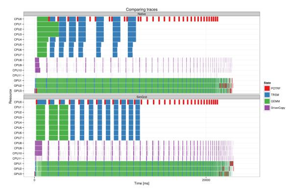
Figure 6.16: Comparing execution traces (native execution on top vs. simulated execution at the bottom) of the Cholesky application with a  $48,000 \times 48,000$  matrix on the Mirage machine using 8 cores and 3 GPUs as workers. Executing kernels on CPUs is much longer since Intel MKL libraries were not used, however simulation predictions are still very precise.
