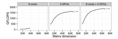
Figure 6.2: For dense linear algebra applications, most of the processing power is provided by GPUs. These plots depict the performance of the Cholesky application on the Mirage machine (see Table 6.1). A clearer view of these performance when restricting to CPU resources (8 cores) is provided in Figure 6.17 (4+4 cores).
