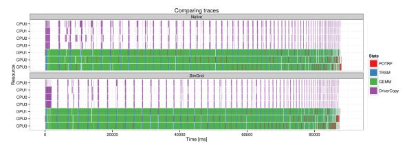
Figure 6.13: Comparing execution traces (native execution on top vs. simulated execution at the bottom) of the Cholesky application with a  $72,000 \times 72,000$  matrix on the Conan machine but using only GPU resources for processing the application.
