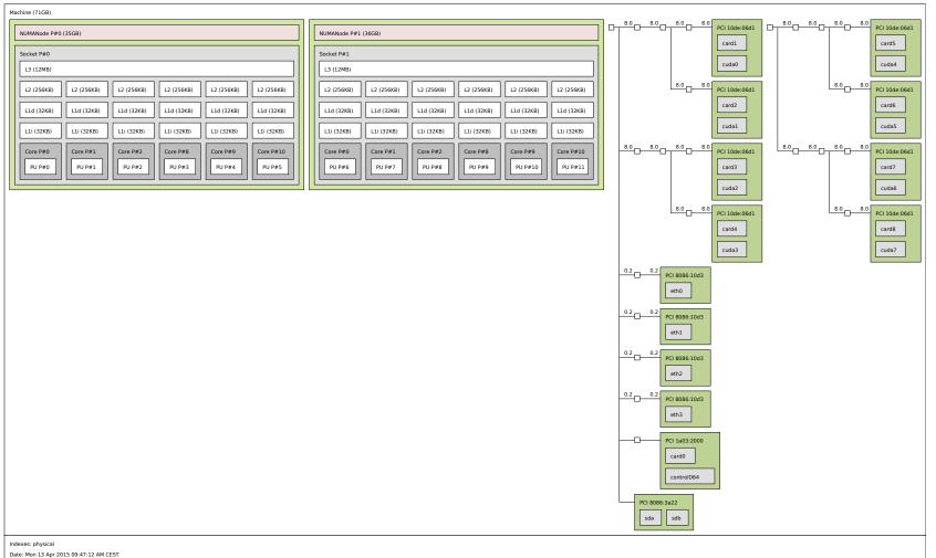
$2~\mathrm{NUMA}$  nodes,  $8~\mathrm{GPUs}$ Figure 5.4: Architecture of the Idgraf machine with 12 cores, distributed on and their interconnect.
