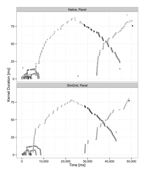
Figure 7.11: Comparing Panel as a time sequence on 8 CPU cores Fourmi machine. Color is related to the task id.
