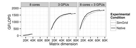
Figure 6.14: Illustrating simulation accuracy for Cholesky application using different resources of the Mirage machine.
