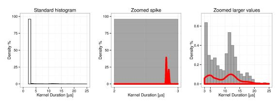
(a) With standard histograms, the bins have uniform width, thus the distribution is poorly captured especially the spike with the lower duration values.
