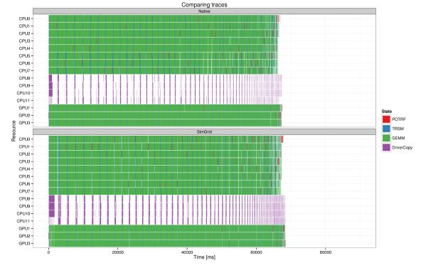
Figure 6.15: Comparing execution traces (native execution on top vs. simulated execution at the bottom) of the Cholesky application with a  $72,000 \times 72,000$  matrix on the Mirage machine using 8 cores and 3 GPUs as workers. Adding 8 cores, improved the performance by approximatelly 20% compared to the performances obtained in Figure 6.13.
