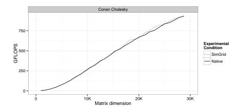
Figure 6.7: Initial results of StarPU simulation for the simplistic use cases were already very accurate. More complex scenarious required more sophisticated models.
