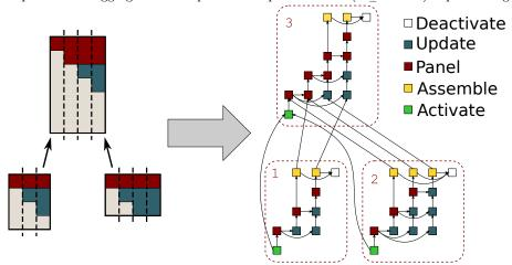
Figure 7.3: Processing a front requires a complexe series of Panel and Update tasks induced by the staircase structure. The dependencies between these operations expressed by the STF code leads to a fine-grain DAG dynamically scheduled by the runtime system.
