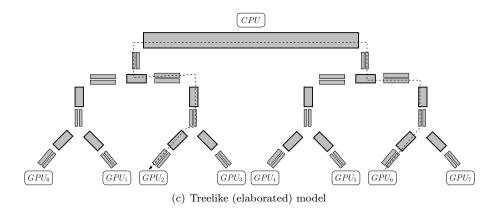
Figure 5.2: Communication and topology modeling alternatives. In the crude modeling, a single link is used and communications do not interfere with each others. The pragmatic complete graph modeling allows for accounting for both the heterogeneity of communications and the global bandwidth limitation imposed by the PCI bus. Complex machine architecture demand for even more elaborated models.
