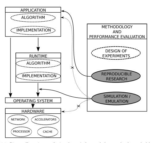
Figure 1.1: Diagram illustrating contributions (in gray) of our work that are related to methodology and performance evaluation. In this thesis, for the simulation aspect of our work we consider solely the case where applications rely on a runtime. Our workflow for doing reproducible research is however completely general.
