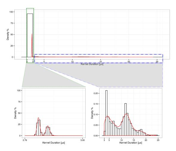
Figure 6.5: Distribution of GEMM kernel durations on a GPU in a single  $72,000 \times 72,000$  Cholesky factorization. Top plot presents the distribution constructed for all observations, while bottom ones are reconstucted for two separate groups of observation depending on their duration value.
