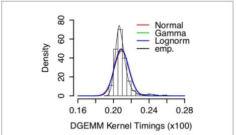
Fig. 4: A plot of the kernel execution times of the DGEMM (part of the Cholesky factorization) kernel along with the fitted distribution curves. The kernel execution times are multiplied by 100 for readability. The simple distributions do not fit quite as well as the DTSMQR kernels, but they seem to model the kernel execution times better than a constant or uniform distribution.
