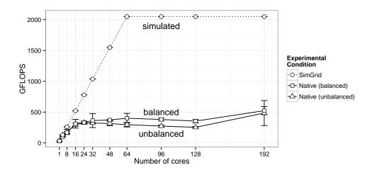
Figure 6.18: Simulation predictions of Cholesky application with a  $32,000 \times 32,000$  matrix (block size  $320 \times 320$ ) on large NUMA Idchire machine are precise for a small number of cores, but scale badly. The reason is that the memory is shared, while models are not taking into account various NUMA effects.
