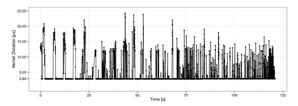
Figure 6.4: GEMM kernel durations on a GPU in a single  $72,000 \times 72,000$  Cholesky factorization, presented as a time sequence. Most of the values are around 2.84 microseconds, but there is a significant number of higher durations as well.
