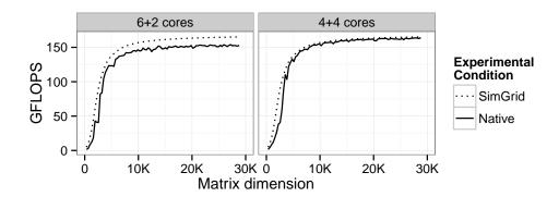
Figure 6.17: Illustrating the impact of deployment when using 8 cores on two NUMA nodes on the Mirage machine.
