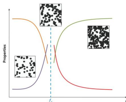
**Fig.1-22** Schematic of nonlinear changes in the properties of composites neat the percolation threshold. The insets demonstrate the geometric phase transistion of conducting fillers.[233]
