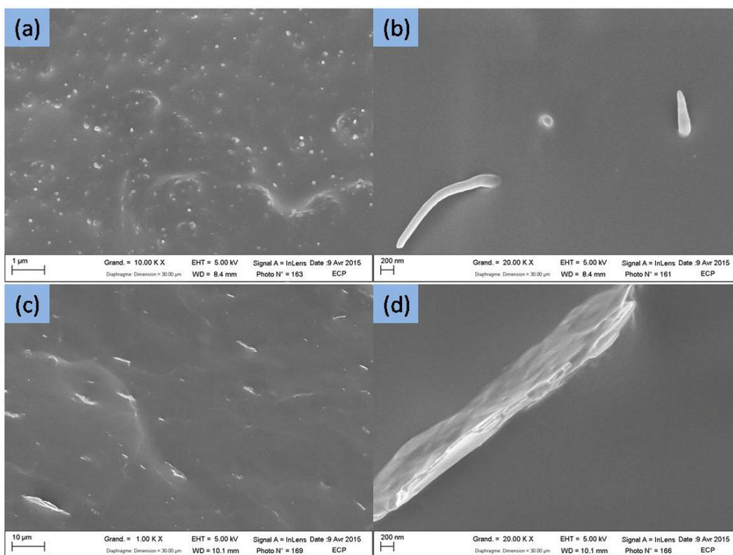
**Fig.4-14** Typical SEM images of fractured surface of (a) CNTs/PDMS composite and (c) GNPs/PDMS composite. (b) and (d) are the high-magnification images of (a) and (c), respectively.
