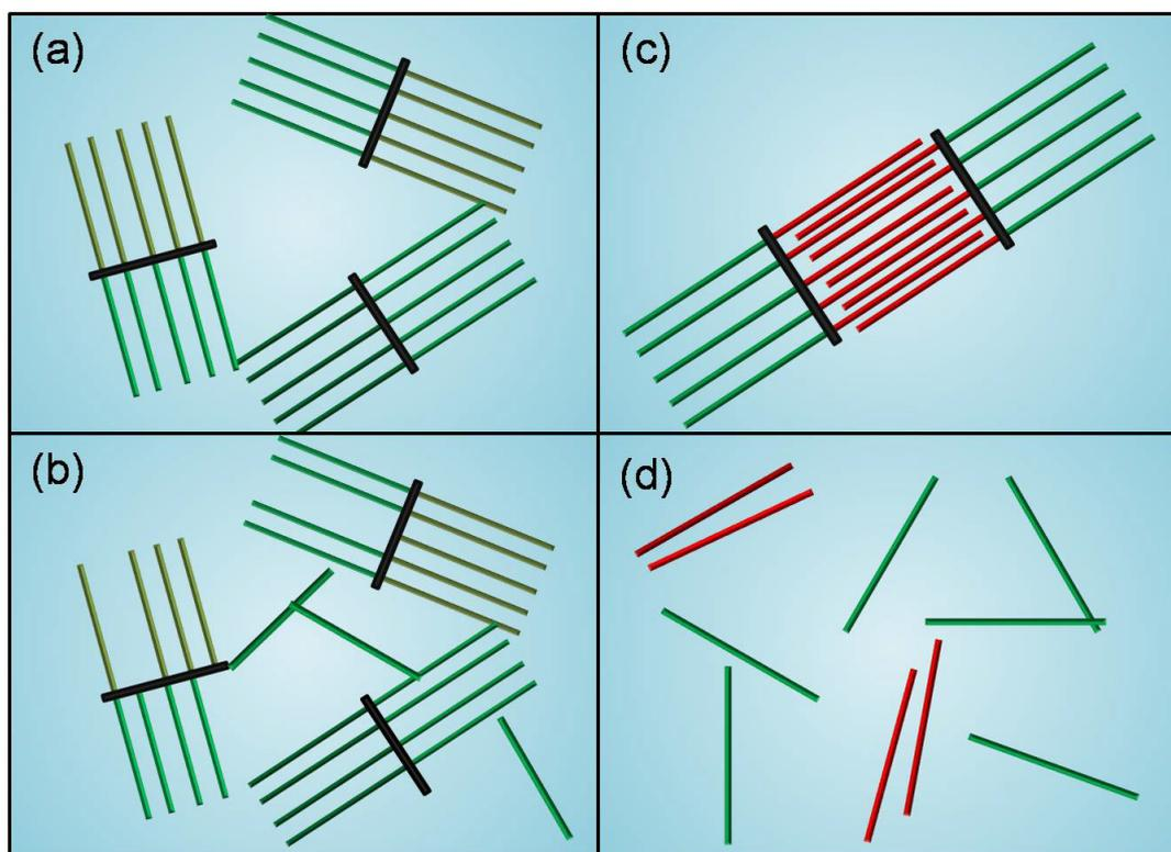
**Fig.3-8** Schematic diagrams of four different potential interaction approaches among the conducting phase of GCHs/PVDF binary composite: the electrical conducting among (a) GCHs-GCHs and (b) GCHs-CNTs, the microcapacitor construction formed by (c) GCHs-GCHs and (d) CNT-CNT. The synthesized CNTs, GNP substrate and microcapacitor construction are demonstrated as green sticks, black sticks and pairs of red sticks.
