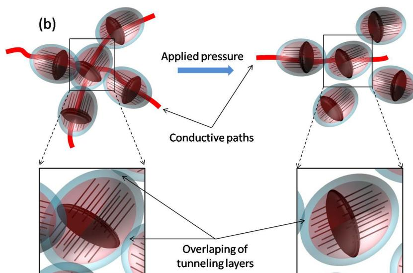
**Fig.4-8** Schematic of (a) the construction of GCHs with improved interfacial area and effectively conductive space. (b) the “hub” structure of GCHs is capable of multi-point communicating with neighboring particles via direct contact or tunneling effect. While, the multi-point communicating is easily influenced by applied pressure, transforming the conductive “traffic hub” to the “isolated island”
