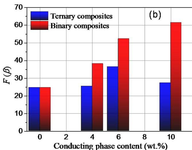
**Fig.3-10** Comparison of (a) FTIR spectroscopy and (b) fraction of  $\beta$ -phase of pure PVDF polymer, GCHs/PVDF binary composites and GNPs/CNTs/PVDF ternary composites with equivalent conducting phases of 4 wt.%, 6 wt.% and 10 wt.%, respectively.
