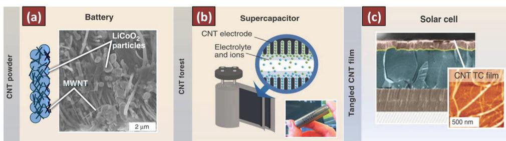
**Fig.1-10** Energy-related applications of CNTs.(a) Mixture of MWCNTs and functional particles for battery electrode. (b) CNTs forest apply to supercapacitor (c) Solar cell using a CNT-based transparent conductor.[50]
