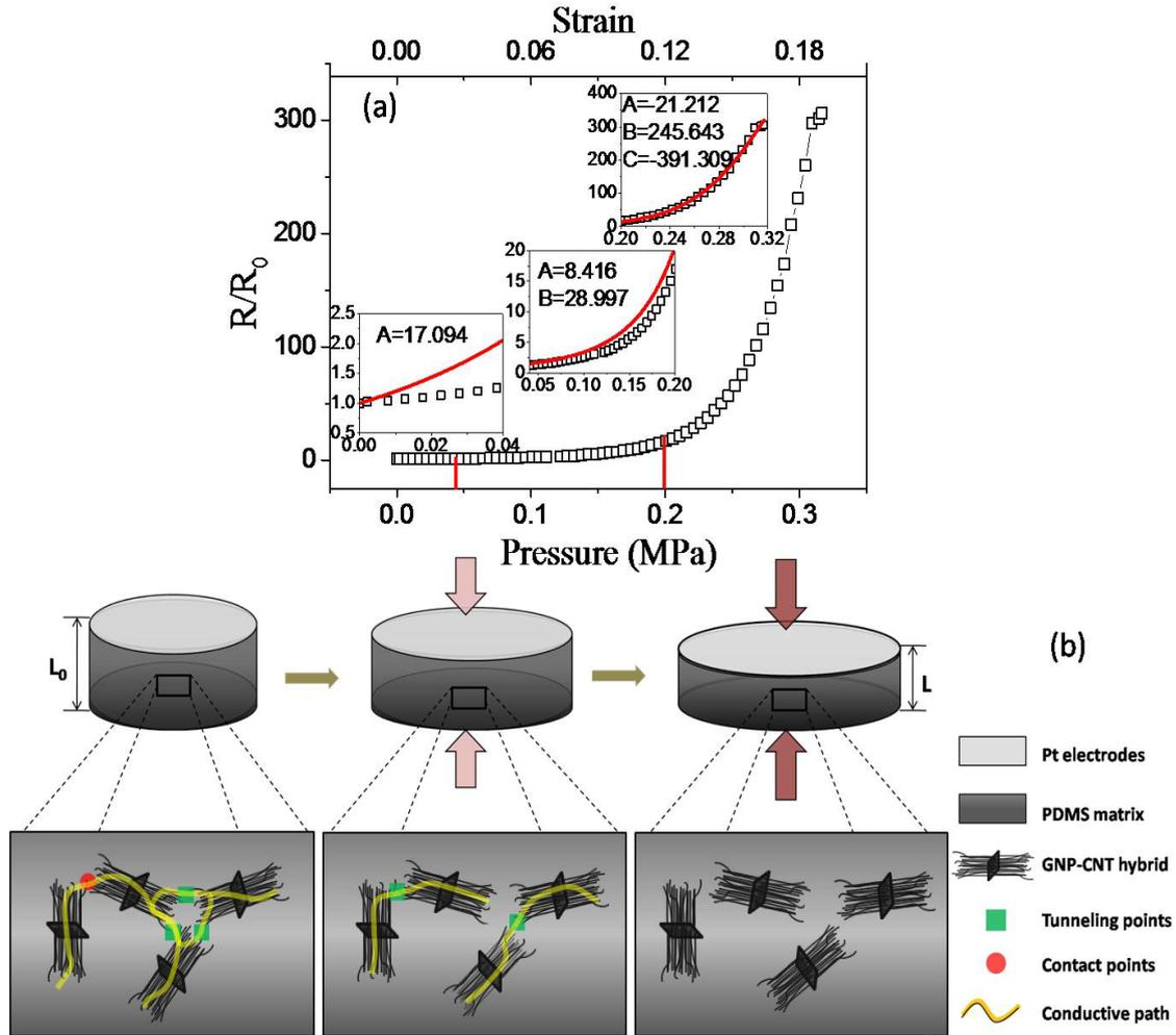
**Fig.4-9** (a) The resistance change on the applied pressure and strain of GCHs/PDMS composite with 0.8 vol.% GCHs. The inset images show the 3-step theoretical fit of experimental data. (b) Schematic diagram of the dependence between the internal conductive network structure and the external applied pressure of 3 steps.
