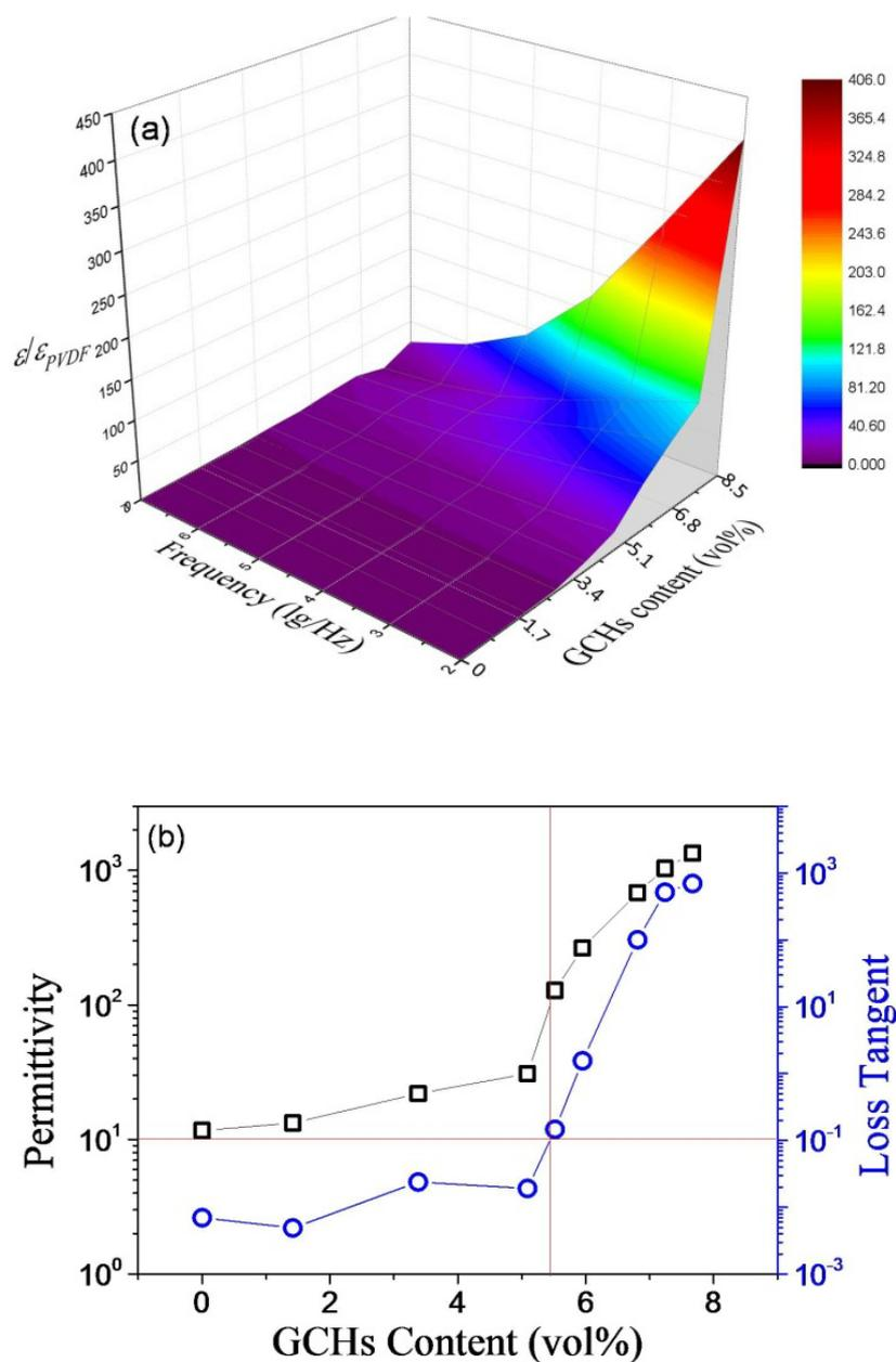
**Fig.3-7** (a)Dependence of the relative enhancement of the dielectric permittivity  $\epsilon/\epsilon_{PVDF}$  on frequency and GCHs volume fractions; (b)Relative permittivity, loss tangent at 1kHz vs. GCHs volume fraction curves
