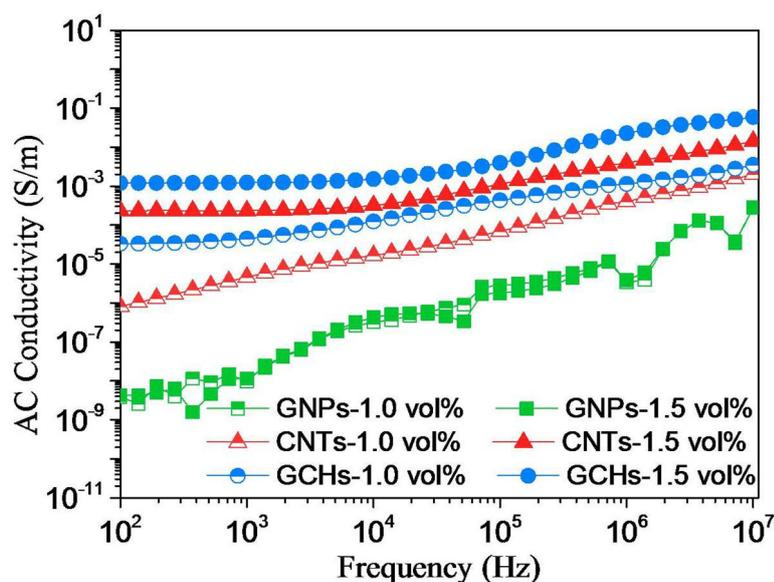
**Fig.4-15** The AC conductivity of PDMS-based composites loading GNPs, CNTs and GCHs with volume fraction of 1.0 vol.% and 1.5 vol.%, respectively.
