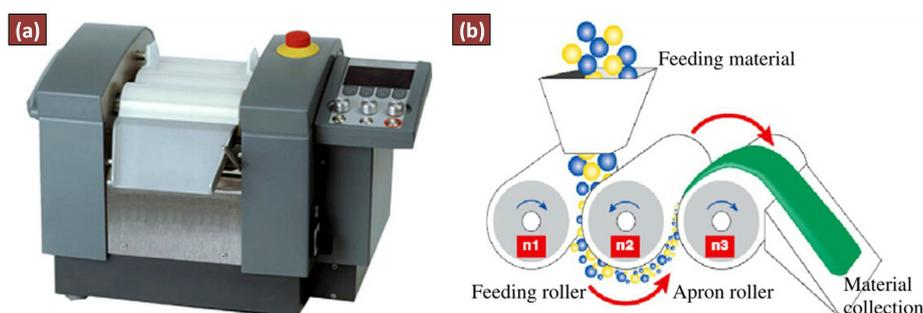
**Fig.1-14** (a) Commercial three roll mills machine and (b) its working mechanism[111]
