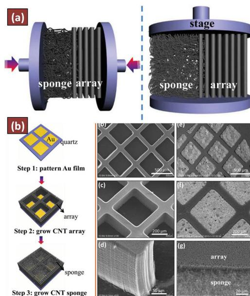
**Fig.1-9** Schematic illustration of (a) compression test and (b) fabrication of patterned parallel structures of three-dimensional CNT sponge-array architectures.[38]
