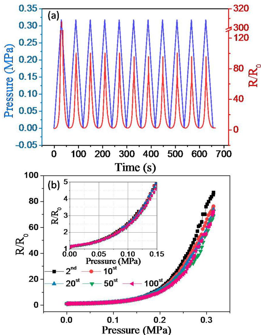
**Fig.4-10** (a) The relative resistance ( $R/R_0$ ) and applied pressure vs. time under periodic loading-unloading tests; (b) ( $R/R_0$ ) under 100 loading-unloading cycles with the pressure ranging from 0-0.31MPa. The inset shows the consistent PR response under 100 loading-unloading cycles with the small applied pressure ranging from 0-0.15MPa.
