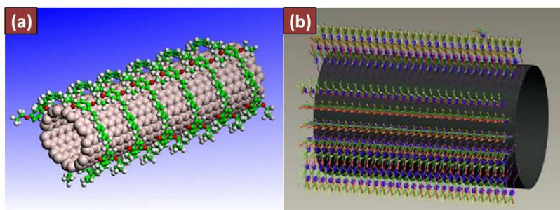
**Fig.1-17** Schematics of CNT functionalization using non-covalent methods. (a) polymer wrapping and (b) surfactant adsorption.[111]
