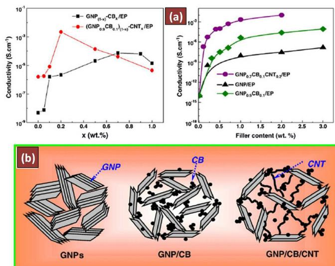
**Fig.1-24** (a) The electrical conductivity of multi-formed conducting particles filled composites. (b) Schematic illustration of the synergistic effect of GNPs, CB and CNTs.
