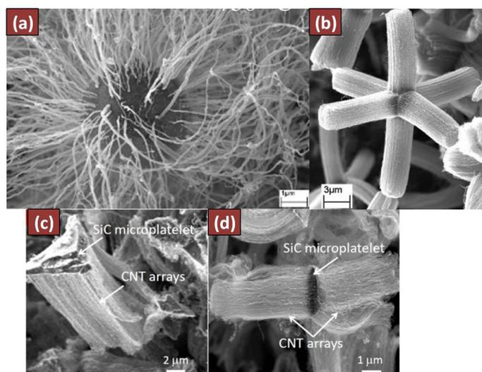
**Fig.1-18** SEM morphologies of (a) the urchin-like and (b) the six-branch structure of  $Al_2O_3$ -MWCNTs hybrid constructions. (c) “single-direction” and (d) “two-direction” SiC-CNT hybrid.[31, 206]
