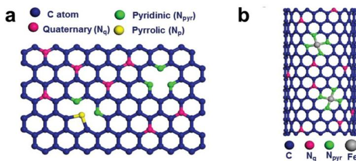
**Fig.1-16** N-doping of CNTs and graphene. (a) possible configurations of N-doping and (b) Fe-N<sub>4</sub> complex hybridized CNT.[193]
