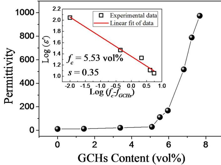
**Fig.3-6** Dependence of the dielectric permittivity (measured at 1 kHz) of the GCHs/PVDF binary composites as a function of the GCHs volume fraction measured at room temperature. The inset shows the best fit of the permittivity to Equation 3-4.
