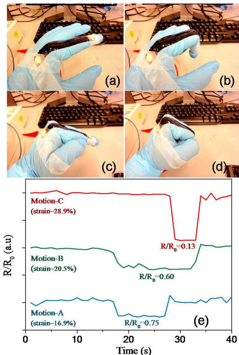
**Fig.4-13** The GCHs/PDMS composite film served as finger movements detections. (a) Photograph of the relaxing state of finger. (b-d) Photographs of three distinct motions (A, B and C) that bending the second joint, the third joint of index finger and clenching, respectively. (e) Relative resistance changes for each independent movement.
