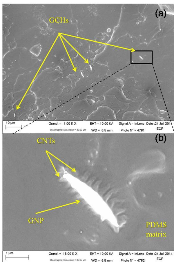
**Fig.4-2** (a) SEM image of the fracture surface of the GCHs/PDMS composite. (b) High-magnification image of GCH particle well embedded in the matrix.
