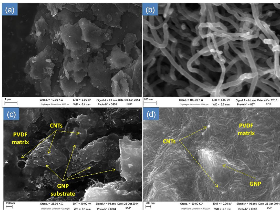
**Fig.3-2** SEM image of (a) as-received GNPs particles with stacked multi-layer constructions and (b) as-received frizzy CNTs structures. The SEM morphology of the fractured surface of (c) GCHs/PVDF binary composite and (f) GNP/CNTs/PVDF ternary composite.
