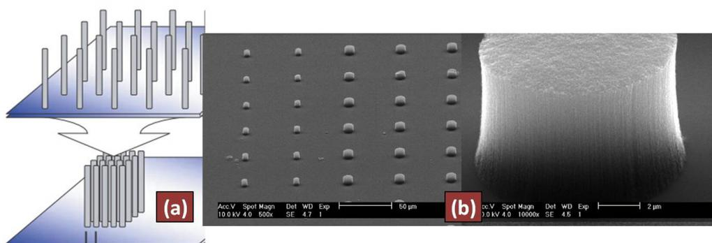
**Fig.1-6** SWCNT forests with ultra-high area density by controlling the CVD process
