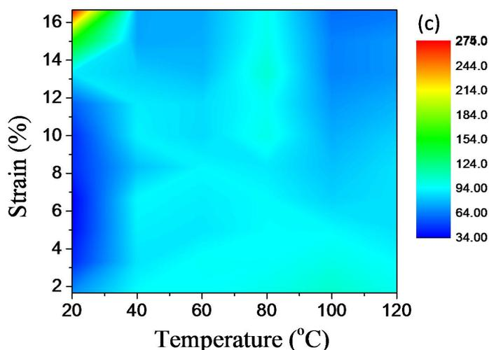
**Fig.4-11.** Temperature-dependent PR property of GCHs/PDMS composites. (a) Resistance change (b) relative resistance enhancement at the function of temperature and applied strain. (c) The distribution of gauge factor in the temperature-strain matrix.
