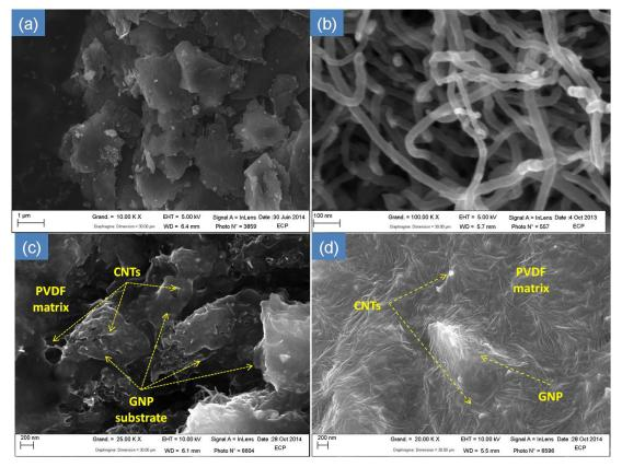
**Fig.3-2** SEM image of (a) as-received GNPs particles with stacked multi-layer constructions and (b) as-received frizzy CNTs structures. The SEM morphology of the fractured surface of (c) GCHs/PVDF binary composite and (f) GNPs/CNTs/PVDF ternary composite.
