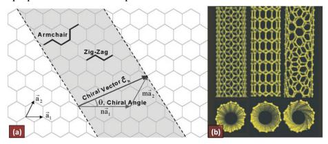
Fig.1-2 (a) Schematic diagram showing the hexagonal sheet structure of CNT and (b) armchair, zigzag and chiral SWCNTs.[7, 9]
