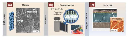
**Fig.1-10** Energy-related applications of CNTs.(a) Mixture of MWCNTs and functional particles for battery electrode. (b) CNTs forest apply to supercapacitor (c) Solar cell using a CNT-based transparent conductor.[50]
