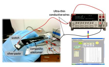
**Fig.4-12** Setup of the finger sensor testing system using the the typical GCHs / PDMS composite film as sensor.
