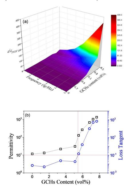
**Fig.3-7** (a) Dependence of the relative enhancement of the dielectric permittivity  $\varepsilon/\varepsilon_{PVDF}$  on frequency and GCHs volume fractions; (b) Relative permittivity, loss tangent at 1kHz vs. GCHs volume fraction curves
