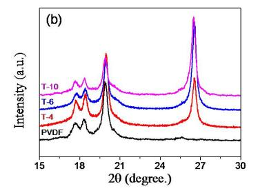
**Fig.3-9** X-ray diffraction patterns of pure PVDF polymer and (a) GCHs/PVDF binary composite: B-4, B-6, B-9 and B-10 and (b) GNPs/CNTs/PVDF ternary composite: T-4, T-6 and T-10.
