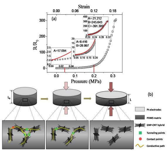
**Fig.4-9** (a) The resistance change on the applied pressure and strain of GCHs/PDMS composite with 0.8 vol.%. GCHs. The inset images show the 3-step theoretical fit of experimental data. (b) Schematic diagram of the dependence between the internal conductive network structure and the external applied pressure of 3 steps.
