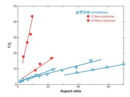
*Fig.1-23* Dependence of the percolation threshold on the aspect ratio of the fillers in composistes filled with randomly oriented fibers.[233]
