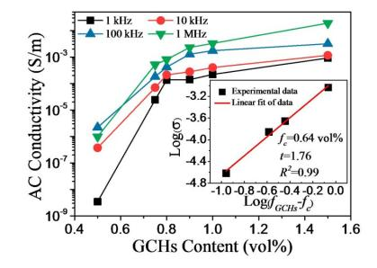
**Fig.4-4** AC conductivity of the GCHs/PDMS composites with different GCHs loading at room temperature. The inset shows the best fit of  $log(\sigma)$  vs.  $log(f_{GCHs}-f_c)$
