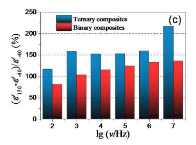
**Fig.3-11** Dependence of relative permittivity on frequency and temperature for (a) GCHs/PVDF binary composite B-6.5, and (b) GNPs/CNTs/PVDF ternary composite T-6.5. (c) The dependence of variation percentages of permittivity on frequency at two testing boundary temperatures: -40 °C and 150 °C.
