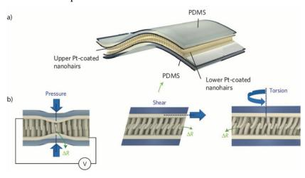
Fig.1-27 Conceptual images of the device composed of interlocking pillars used for detecting multiple stimuli. [254]
