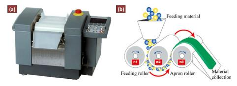
Fig.1-14 (a) Commercial three roll mills machine and (b) its working mechanism[111]
