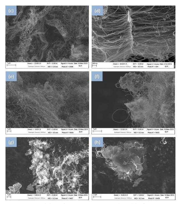
**Fig.2-2** SEM morphology of GCHs constructions synthesized by floating CCVD process at different temperature. (a),(b) 550 °C; (c),(d) 650 °C; (e),(f) 750 °C; (g),(h) 850 °C.
