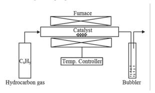
Fig. 1-4 Schematic illustration of catalytic CVD process
