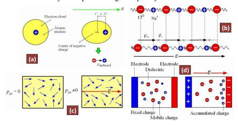
Fig.1-19 Electrical mechanism of (a) electron, (b) ionic, (c) dipole and (d) interfacial polarization.[217]
