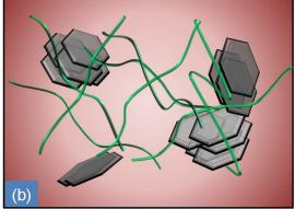
Fig.3-1 Schematic illustration of the difference between (a) GCHs/PVDF binary composites and (b) GNPs/CNTs/PVDF ternary composites
