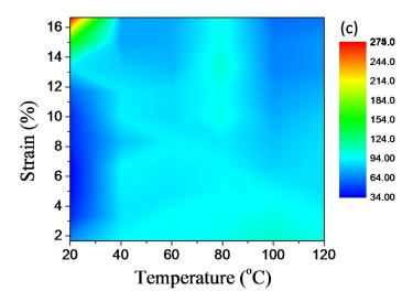
**Fig.4-11.** Temperature-dependent PR property of GCHs/PDMS composites. (a) Resistance change (b) relative resistance enhancement at the function of temperature and applied strain. (c) The distribution of gauge factor in the temperature-strain matrix.
