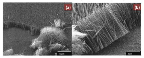
Fig.1-5 SEM morphologies of straightness of MWCNTs grown on the glass through CVD.
