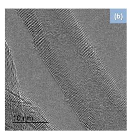
**Fig. 2-9** (a) Typical TEM image of the part of GCHs (b) High-resolution TEM image of synthesized CNT with detailed displayed structure.
