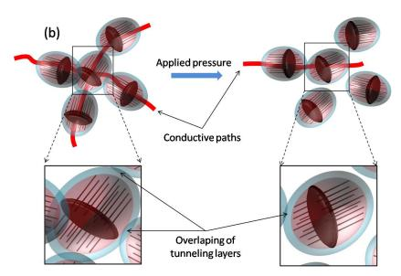
Fig.4-8 Schematic of (a) the construction of GCHs with improved interfacial area and effectively conductive space. (b) the "hub" structure of GCHs is capable of multipoint communicating with neighboring particles via direct contact or tunneling effect. While, the multi-point communicating is easily influenced by applied pressure, transforming the conductive "traffic hub" to the "isolated island"
