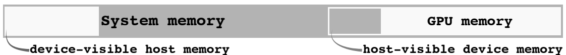
FIGURE 3.8: An illustration of the different memory partitions of an APU. The system memory and the host-visible device memory are visible to the CPU cores. The GPU memory (being a sub-partition of the system memory) and the device-visible host memory are visible to the integrated GPU compute units.
