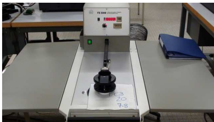
Figure 6. 6 : Air Perméability Tester FX 3300
