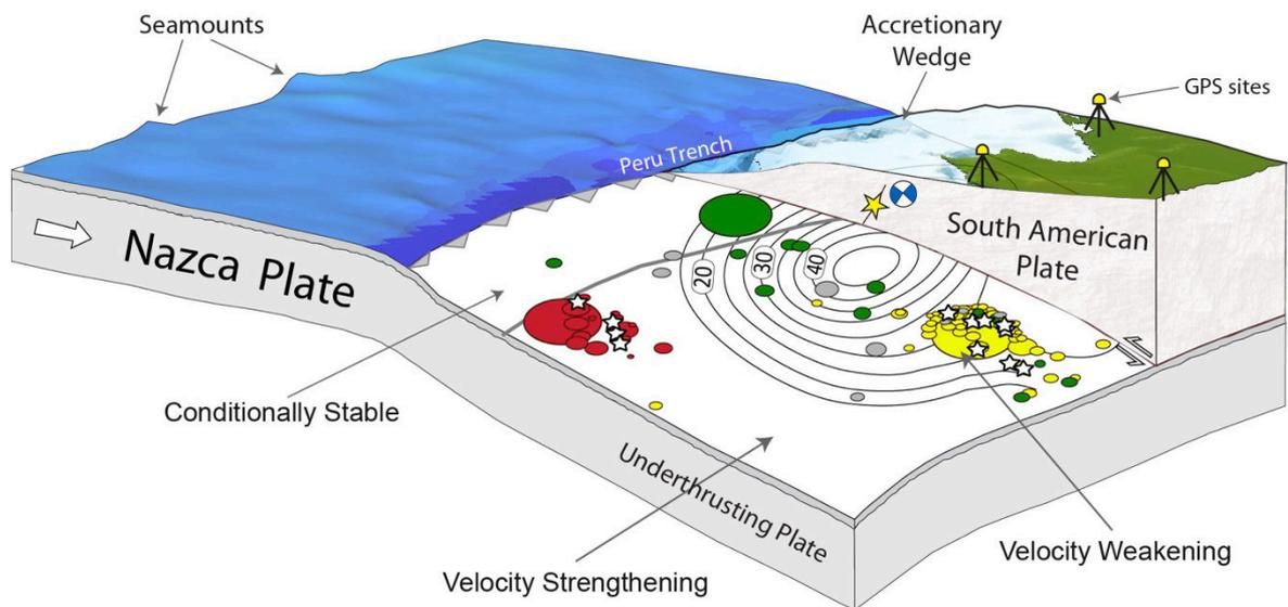
**Figure 4.4.** Cartoon illustrating the spatially variable frictional properties of the subduction interface in the Bayovar area. The plate interface is predominantly velocity-strengthening with small localized patches of velocity weakening and a conditionally stable friction region in the shallowest part of the interface close to the trench.
