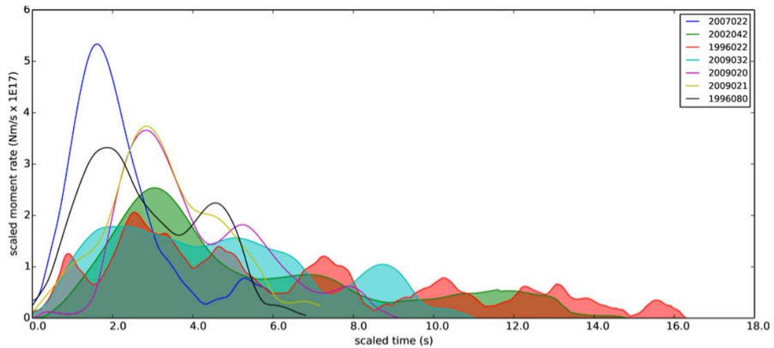
**Figure 4.3.** Source Time Function (STF) comparison for shallow interface earthquakes in northern Peru. Abnormally long STF are shown filled colors between the curve and the x-axis. The 2002 abnormally long earthquake occurred in the same area as the 2009 sequence.
