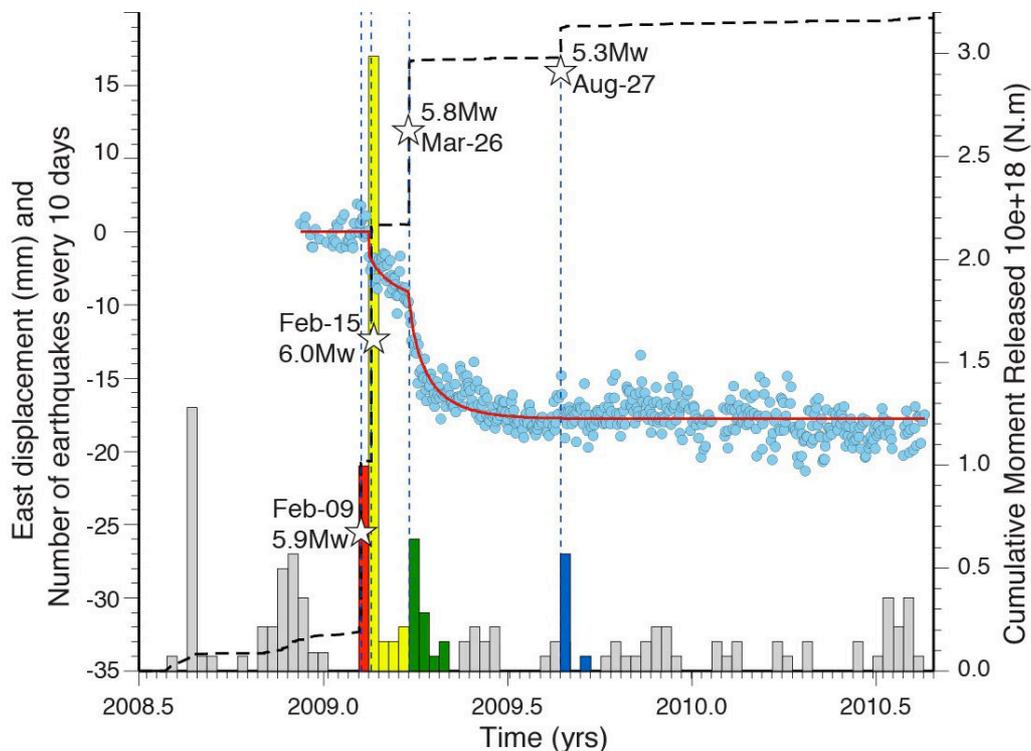
**Figure 4.1.** Geodetic time series and seismicity rate from 2008.5 to 2010.65. Blue dots indicate the east displacement recorded by the CGPS BAYO expressed with respect to the overriding plate. Histogram bars show the number of seismic events in 10 days intervals and the colors correspond to the time periods of the seismic sub-sequences shown in Figure 4.2.
