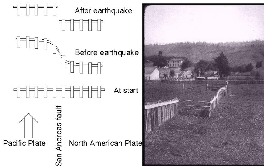
**Figure 1.2:** Left: Schematic representation of the elastic rebound model after Reid, [1910]. Right: picture showing a fence that was offset due to the fault slip during 1906 San Francisco earthquake. USGS image: (<http://earthquake.usgs.gov/regional/nca/1906/18april/reid.php>).
