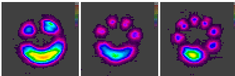
Figure 5.23 – ECR laser beam profiles. Those modes can be observed using a lens after the output coupler to image the “rings” on the camera. On the left, the lower order mode observed. On the right, higher order modes.
