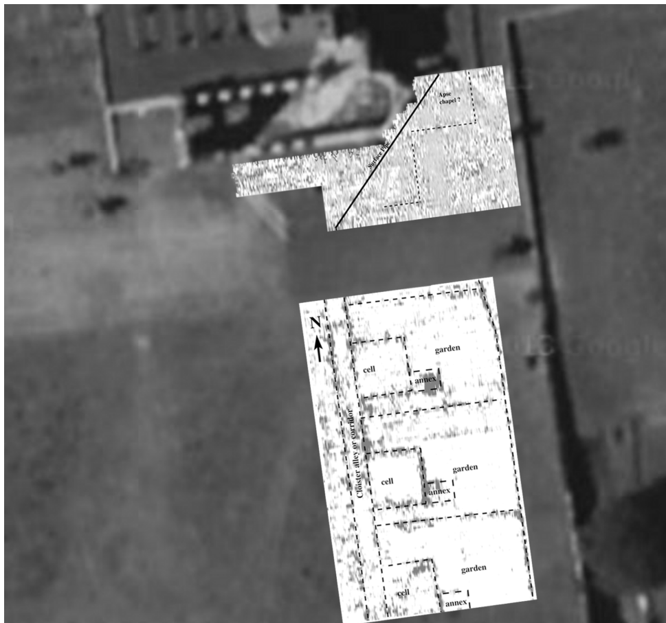
FIGURE A.8 – Superposition of the GPR surveys over a satellite image of the area.
