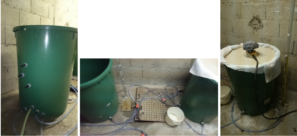
FIGURE 4.8 – Pictures of the experiments. On the left is presented the tank filled with water, with its overflow connections. Middle picture shows the tubing linking both tanks. The picture on the right displays the sand tank with the GPR set at the top with a load on it.
