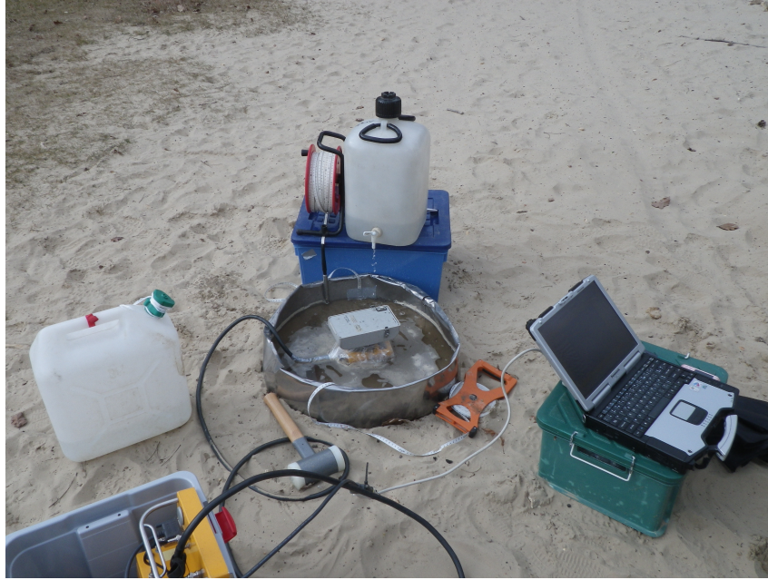
FIGURE 2.2 – Picture of the experiment. Ring infiltrometer filled with 5 cm of water. The 1.6 GHz antennae are in the middle protected from water by a plastic cover. We used a water level controller coupled with a tap-tank to maintain the 5 cm of water.
