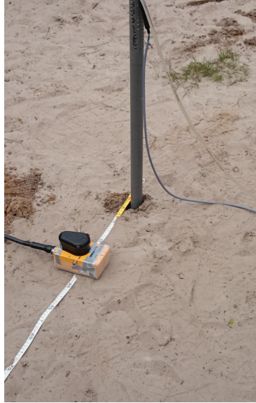
FIGURE 3.2 – Picture of the experiment. The antennae are centered on 1600 MHz. The PVC tube was inserted 30 cm into the soil. A piezometer and a tube for water supply were inserted in it.
