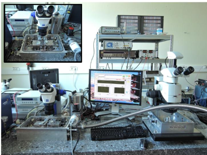
*Figure 4.18:* Picture of the probe station used for I(V) and C(V) characterization of the samples. The sample characterization is made under vacuum ( $<10^{-3}$  Torr) and in the dark to avoid any effects due to optical excitation. The temperature is controlled with a Linkam cooling system from liquid nitrogen temperature to 600 °C.
