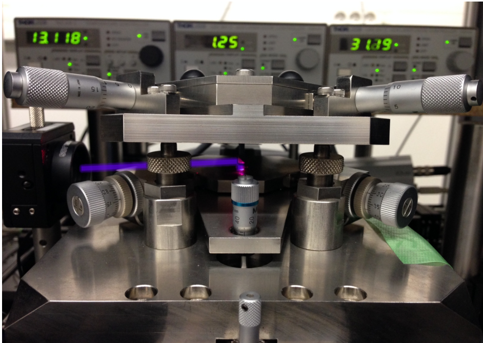
Fig. 4.8: A prism is mounted on HS-AFM microscope head to direct the excitation laser toward the sample.
