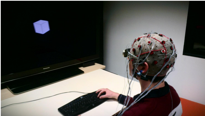
Figure 5.4 – Setup of the experiment, with a participant being presented with stereoscopic images while his EEG signals are being recorded.
