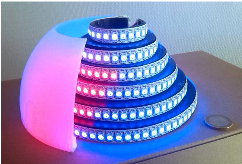
Figure 10.13 – Prototype of a spherical display composed of LEDs (Adafruit NeoPixels) that could replace projection to display EEG signals with spatial augmented reality.
