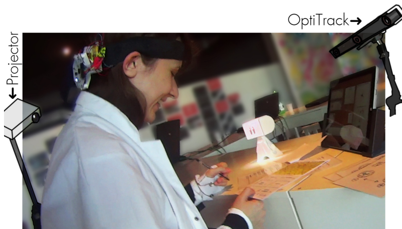
Figure 11.10 – In a scientific museum, various activities were proposed to visitors in order to prompt self-investigation. The setup consists of a projector handling the augmentation and an OptiTrack for the tracking.
