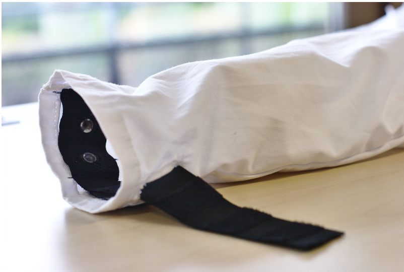
Figure 11.4 – Wearables: coat embedding ECG sensors.
