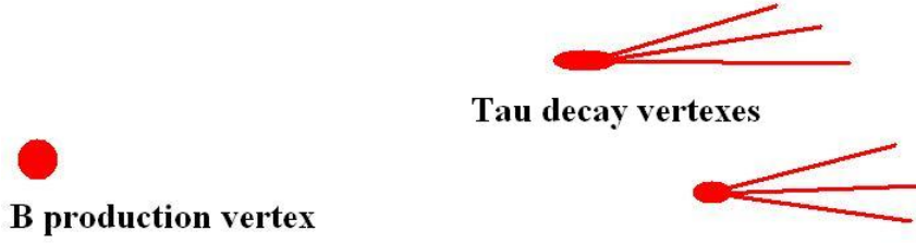
Figure 4.2: Schematic representation of how a B_{(s)}^0 \rightarrow \tau^+(\rightarrow (3\pi)^+\nu_\tau)\tau^-(\rightarrow (3\pi)^-\nu_\tau) decay is reconstructed with the LHCb detector: only the B production vertex and the two three-prongs \tau decay vertices can be directly reconstructed.
