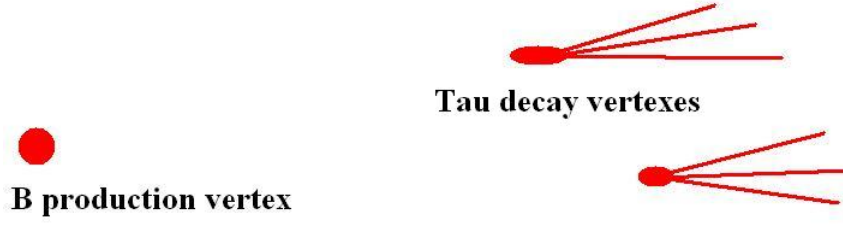
Figure 4.2: Schematic representation of how a B_{(s)}^0 \rightarrow \tau^+(\rightarrow (3\pi)^+\nu_\tau)\tau^-(\rightarrow (3\pi)^-\nu_\tau) decay is reconstructed with the LHCb detector: only the B production vertex and the two three-prongs \tau decay vertices can be directly reconstructed.
