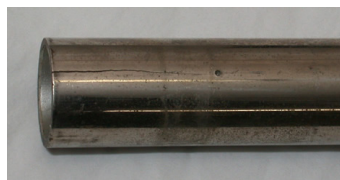
Figure 1.2: Steam generator tubes.
