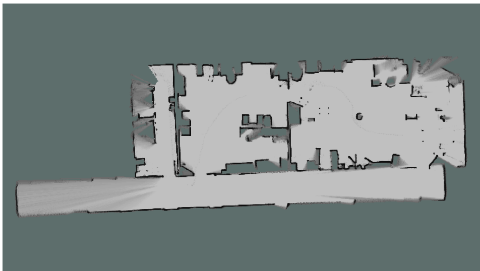
Figure 2.3: An occupancy grid. White represents free cells, black are occupied cells and gray are unexplored. This map was produced by our perception pipeline using the HectorSlam algorithm (Kohlbrecher et al. 2011).
