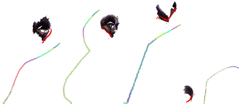
Figure 5.6: Sample of 4 trajectories for the black armchair from the dataset. Regions with the same color represent the same view from the TLD dictionary. They are placed where the robot has perceived them. We can see that the trajectories share resemblances, and that it could be possible to recognize the object with a few of them as references.
