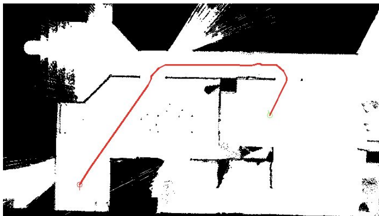
Figure 3.6: Example of a smoothed global path. The white represents traversable cells and black forbidden ones. The computed path is represented by the red line.
