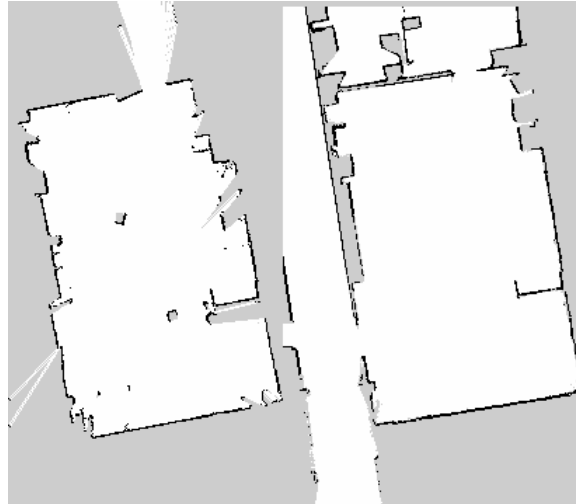
Figure 3.8: A map of a room after a first arbitrary run of the robot, the same static map after several runs.
