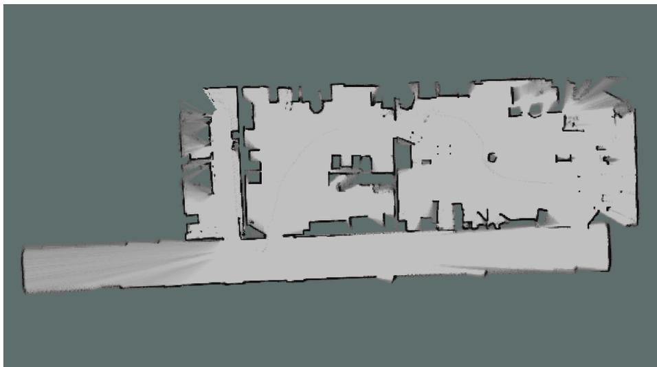
Figure 2.3: An occupancy grid. White represents free cells, black are occupied cells and gray are unexplored. This map was produced by our perception pipeline using the HectorSlam algorithm (Kohlbrecher et al. 2011).
