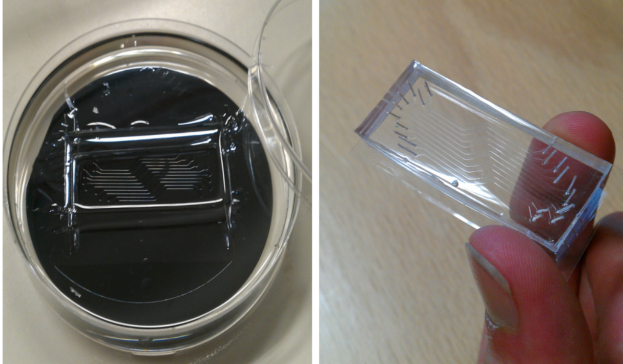
Figure 21 - Picture of one microfluidic chips used in this work (parallel-H-Shaped). Left: picture of a wafer covered in hardened PDMS and which acts as a mold. Right: Once cut out from the wafer, a chip is punched, plasma-cleaned and bonded to a coverslip.
