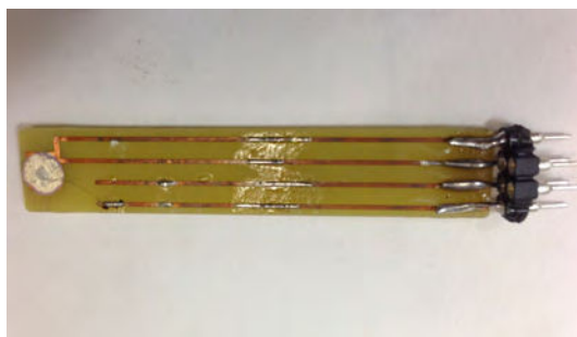
Figure 2.13: The sample holder used for pyroelectric current measurement.
