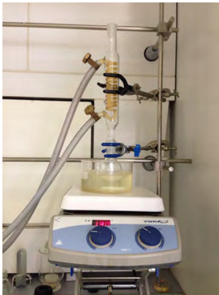
Figure 2.3: The device with condenser we used to obtain the precursor by sol-gel method.
