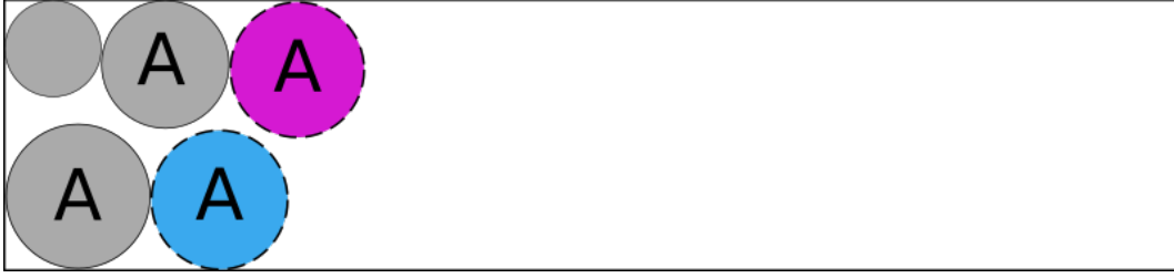
Figure 5.7 – A node in the DP tree. Shape-positions in grey have been fixed. The stack in blue is a valid shape-position at this node, but not the stack in purple as it violates the alternate rule. However, if we fix the stack in blue, then the stack in purple becomes valid in this child node. (top view)
