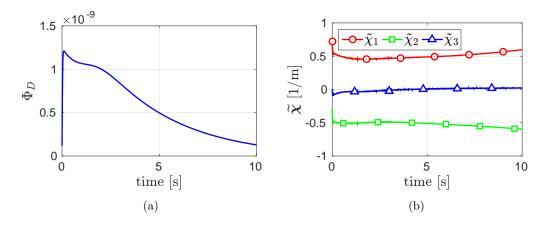
Figure 5.12 – Simulation results obtained by employing the classical discrete moment set  $(x_g, y_g, \mu_{20} + \mu_{02})$  and optimizing for the camera linear velocity  $\boldsymbol{v}$ . In this case  $\Phi_D(t)$  keeps very close to zero (the scale of Fig. (a) is  $10^{-9}$ ) and as a consequence the estimation error  $\tilde{\boldsymbol{\chi}}(t)$  does not converge (Fig. (b)).
