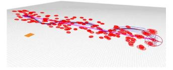
Figure 3.2 - **Trajectory planning to minimize uncertainty for micro aerial vehicles**. The objective is to reach the final pose (to the left) while minimizing the localization uncertainty. The resulting trajectory (black line) is more informative than the direct magenta path. From [AWCS13].
