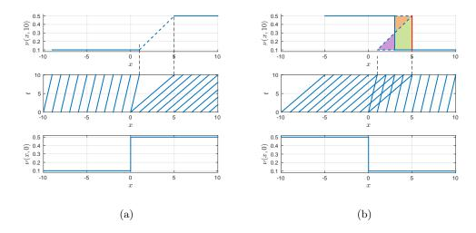
Figure B.5 – Time-space evolution of a rarefaction and shock wave. Fig. (a): evolution of a rarefaction wave. Fig. (b): evolution of a shock wave. For both figures, from bottom to top we show: (i) the initial condition  $\nu(x, 0)$ , (ii) some of the characteristic curves emanating from x = -10 + k with k = 0, 1, ..., 20, and (iii) the final condition  $\nu(x, 10)$ . This picture is similar to some reported in [LeV02].
