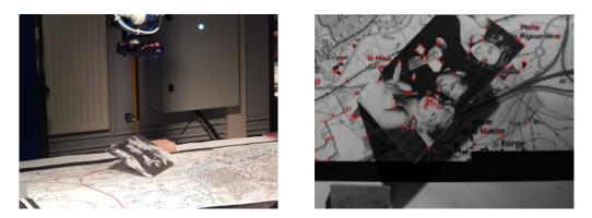
Figure 5.9 – Experimental setup for the estimation of the plane parameters in presence of outlier measurements. Note the introduction of the inclined picture in the observed scene on the right.
