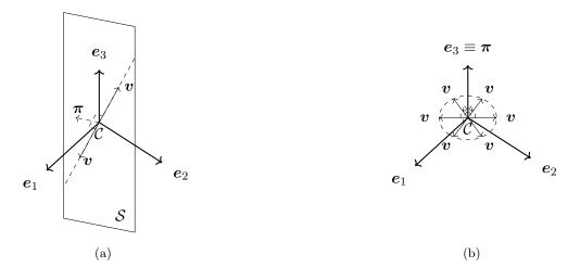
Figure 4.1 – Optimality conditions for the camera linear velocity v as dictated by system (4.33). Fig. (a): when  $\pi \neq e_3$ , vector v must be orthogonal to  $\pi$  and lie on the plane S spanned by  $\pi$  and  $e_3$  (that is, v must belong to a specific straight line). Fig. (b): when  $\pi = e_3$ , any  $v \perp e_3$  is a valid solution to (4.33).
