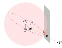
Figure 2.4 – Planar and spherical perspective projection models.
