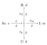
Figure C.3 – Bond graph representation of the mass-spring-damper system. The constitive equations for each element are R:  $e_d = d\dot{x}$ ; I:  $e_k = k \int \dot{x}(\tau) d\tau$ ; C:  $\dot{x} = \frac{1}{m} \int e_m(\tau) d\tau$ , and finally, for the 1-junction,  $e - e_k - e_d - e_m = 0$  where the signs in the summation were chosen according to the direction of positive power represented by the half-arrows.
