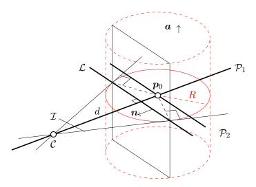
Figure 4.5 – Geometry of a cylindrical object. Camera C and cylindrical target  $\mathcal{O}_C$  with the planar limb surface  $\mathcal{L}$  and the other planes of interest  $\mathcal{P}_1$  and  $\mathcal{P}_2$
