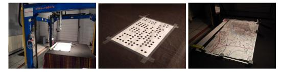
Figure 5.6 – **Experimental set-up for plane estimation** with the dotted pattern and the topographic map used for feature extraction and tracking.
