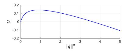
Figure 6.1 – A representative graph of the cost function used to calculate the **IBVS secondary task** in (6.8) plotted against  $\|\dot{\boldsymbol{q}}\|$  for  $k_{\sigma} = 1$ ,  $k_d = 0.2$ ,  $\gamma = 0.1$ , and assuming  $\sigma_1^2 = \|\dot{\boldsymbol{q}}\|^2$ . Note the presence of a finite upper bound for  $\mathcal{V}(\dot{\boldsymbol{q}})$  as desired.
