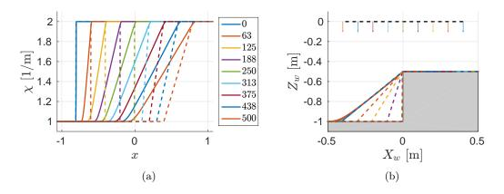
Figure B.6 – Photometric depth estimation for a rarefaction wave. Fig. (a) evolution of the actual (dashed) and numerically propagated (solid) disparity map at equally spaced iterations (check the legend). Fig. (b) reconstruction of the environment from the actual (dashed) and numerically propagated depth maps with arrows representing the camera position and the direction of the optical axis, and using the same color code as in Fig. (a).
