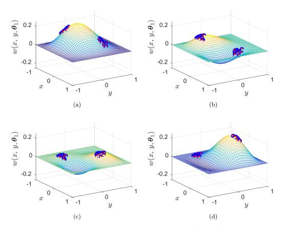
Figure 5.16 – Four snapshots of the weighting function  $w(x, y, \theta_1)$  taken during the camera motion. It is interesting to visualize how function  $w(\cdot)$  automatically adjusts its shape as a function of the observed scene (e.g., it tends to peak around clusters of points).
