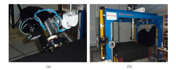
Figure 5.1 – **Experimental setup.** The Point Grey Dragonfly2 greyscale camera Fig. (a) and the 6-DOFs Gantry robot Fig. (b) used for all experiments.
