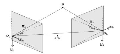
Figure 2.5 – Geometrical representation of the epipolar constraint. The points  ${}^{a}\pi$  and  ${}^{b}\pi$  represent the projections of the same point p from two camera vantage points related by the rigid transformation described by the rotation matrix  ${}^{a}\mathbf{R}_{b}$  and the translation vector  ${}^{a}_{a}\mathbf{t}_{b}$ .
