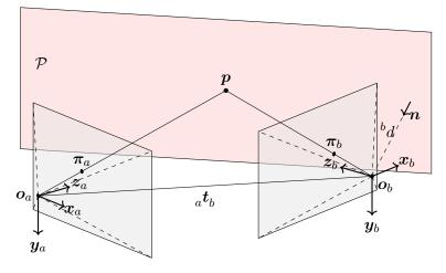
Figure 2.6 – Geometrical representation of the homography constraint. The points  ${}^{a}\pi$  and  ${}^{b}\pi$  represent the projections of the same point p from two camera vantage points related by the rigid transformation described by the rotation matrix  ${}^{a}\mathbf{R}_{b}$  and the translation vector  ${}^{a}_{a}\mathbf{t}_{b}$ .
