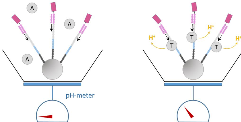
FIGURE 1.6 – Sequencing with Ion Torrent technology. A single sphere coated with clonal DNAs is introduced into each well. Each dNTP is introduced sequentially. If the dNTP is incorporated by polymerisation, it releases  $H^+$  ions which are detected by pH-meter under each well.
