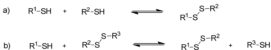
Scheme 1.5 The general equation for a) disulfide formation (involves oxidation, with H_2 as the other formal product) and b) disulfide exchange (also involves oxidation state changes at sulfur).
