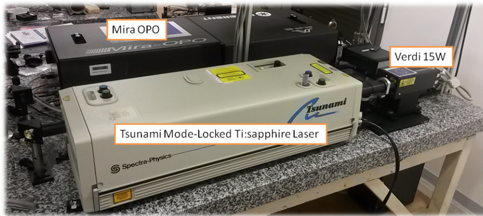
Figure 24: Picture of our picosecond pulsed laser chain.
