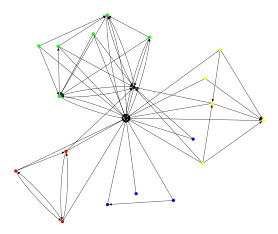
Figure 3.3: Scheme of a multi-community (architecture) overlay network
