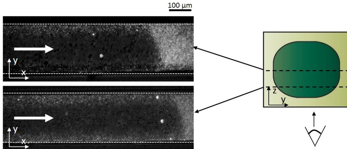
**Figure 5.10** – Film left behind the interface for the displacement of a microgel 2.2% by a microgel 1.6% at a pressure drop of 0.5 bar with no slip at the walls. The focus of the microscope objective is made at the symmetry plan (top line) of the channel and denser to the bottom of the channel (bottom). the film thickness varies weakly in the center part of the channel.
