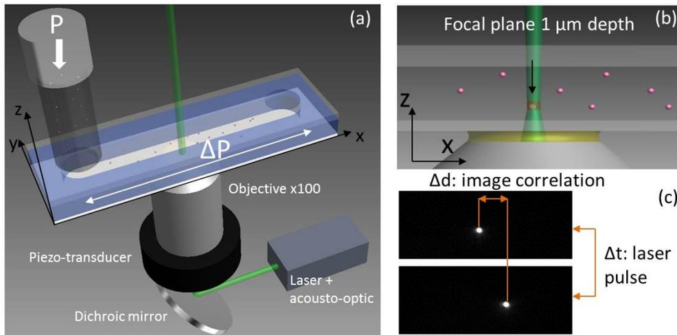
**Figure 3.6** – Experimental  $\mu$ PIV set-up. (a) The tracers in the fluid are excited by epifluorescence with a laser beam modulated by an acousto-optic modulator. The emitted signal is transmitted to the camera thanks to the dichroic mirror. (b) The precision of the experiment depends mostly on the focal plan depth which is  $1\ \mu\text{m}$ . (c) The displacement of the beads is determined by image correlation, the images are filtered to remove background noise.
