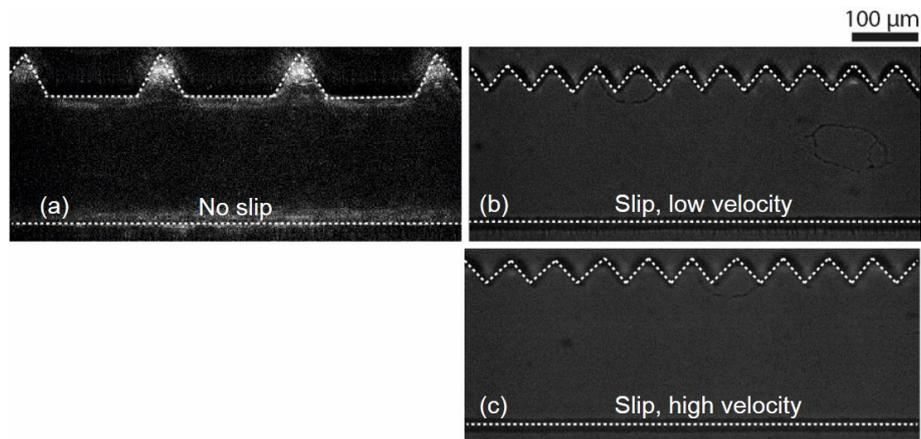
**Figure 5.26** – Pictures of the corrugations when 4 channel volumes have been injected for the displacement of a microgel 3% with a microgel 1.6% (a) with no slip at 0.8 bar, (b) with slip at 0.6 bar and (c) with slip at 0.8 bar.
