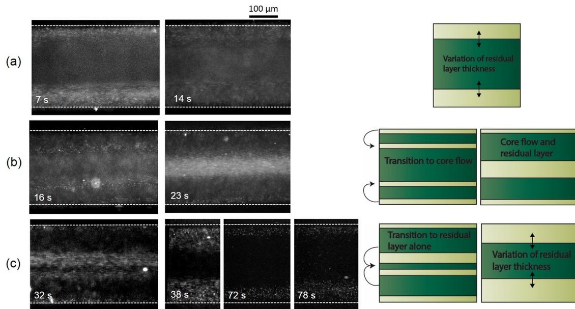
**Figure 5.28** – From (a) to (c) Time evolution of the flow of a microgel 2.2% displaced by a microgel 1.6% with no slip at the walls at a constant pressure drop of 0.5 bar after the meniscus has exited the channel: a complex dynamic takes place where the two phases exchange position.
