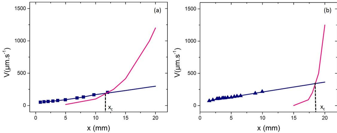
**Figure D.4** – Evolution of the velocity of the interface as a function of its x-position for the displacement of (a) a microgel 2.2% and of (b) a microgel 3% by a microgel 1.6% at a pressure drop of 0.3 bar. The symbols are the experimental measurements. The blue lines corresponds to the linear fit of the slip regime observed at the beginning of the experiment. The pink line corresponds to the calcul of the velocity of the interface with no slip boundary conditions.
