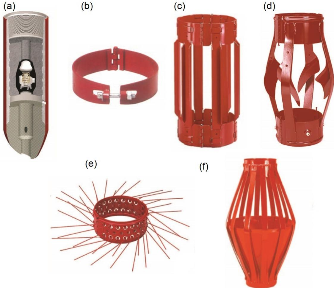
**Figure 1.7** – Hardware outside the casing: (a) a guide shoe with a rounded nose, (b) a stop collar, (c) a rigid centralizer, (d) a turbolizer: a turbulence-inducing centralizer, (e) a scratcher and (f) a cement basket. Reproduction from [133].
