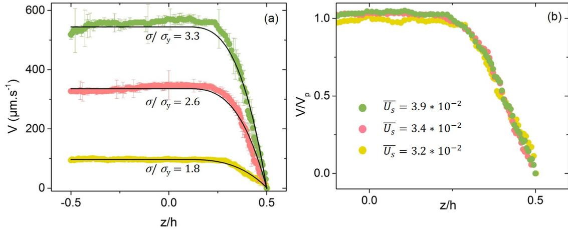
**Figure 4.14** – (a) Truncated plug-flow profiles in an asymmetric channel (slip - no slip) at various reduced stress: 1.8 (yellow), 2.6 (pink), 3.3 (green). The solid lines are the best fits to the theoretical asymmetric Herschel-Bulkley profiles. (b) Truncated plug-flow profiles near the rough no slip surface. The velocity profiles are scaled by the central plug velocity.
