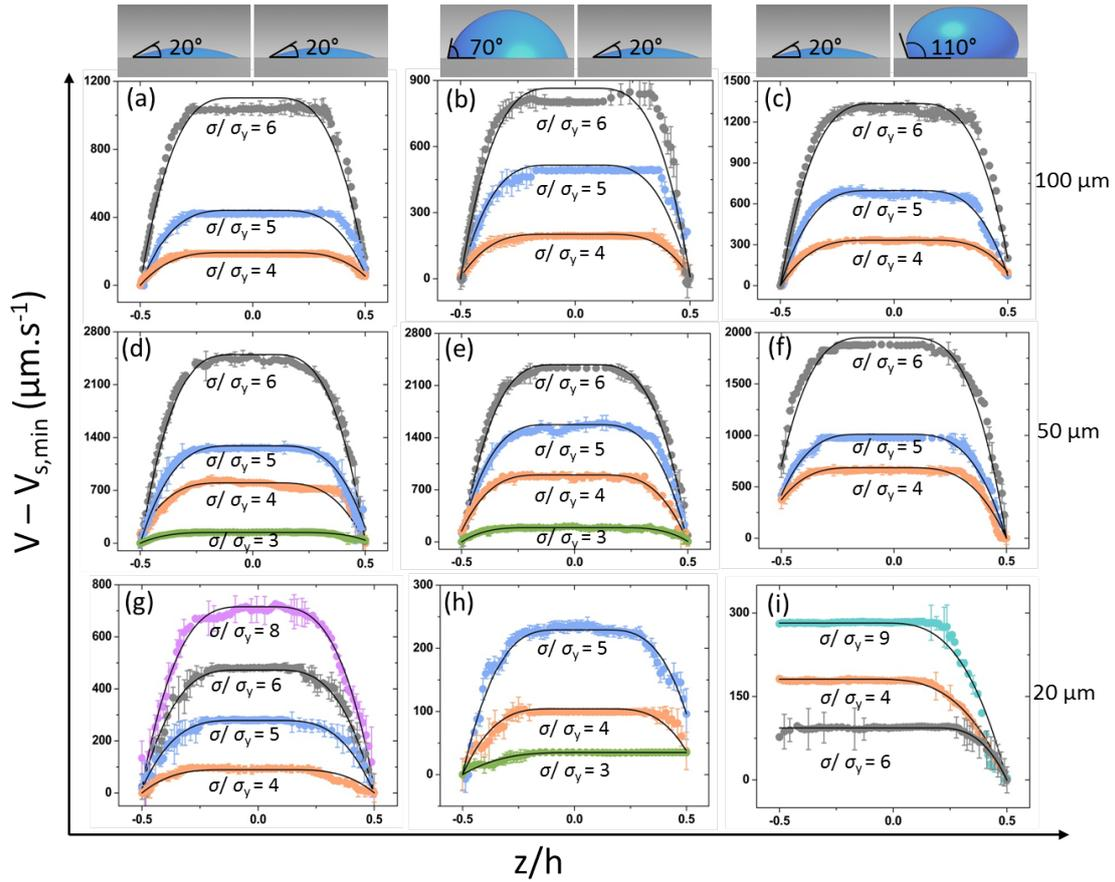
**Figure 4.7** – Velocity profiles  $V$  corrected from the slip velocity  $V_{s,min}$  for various heights, boundary conditions, and reduced stress  $\sigma/\sigma_y = 9$  (dark cyan), 8 (purple), 6 (gray), 5 (blue), 4 (red), 3 (green). The solid lines are the best fits to the theoretical expression of the velocity profiles calculated in the asymmetric Herschel-Bulkley flow model 4.2.3.
