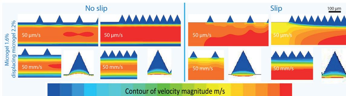
**Figure 6.21** – Velocity field near the corrugations obtained for the simulations of the displacements of a microgel 2.2% by a microgel 1.6% in the geometries A and B with no slip (left panel) and slip (right panel) at velocities of  $50 \mu\text{m s}^{-1}$  (top line) and  $50 \text{mm s}^{-1}$  (bottom line). The velocity field is taken at the time the interface leaves the channel.
