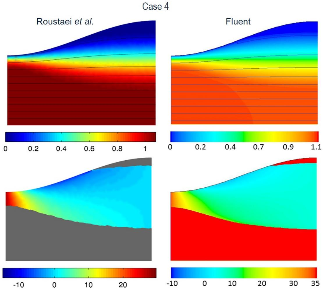
**Figure 6.10** – Comparison of case 4:  $B = 10$ ;  $h = 0.5$  and  $\delta = 0.25$  between the results of Roustaei *et al.* (left panel) and our results with Fluent (right panel). Top: Velocity field (m/s). Bottom: Pressure field (Pa).
