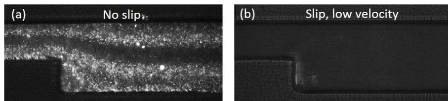
**Figure 5.22** – Film thickness at the time the interface leaves the channel for (a) no slip and (b) slip at low velocity for the displacement of a microgel 2.2% by a microgel 1.6%.
