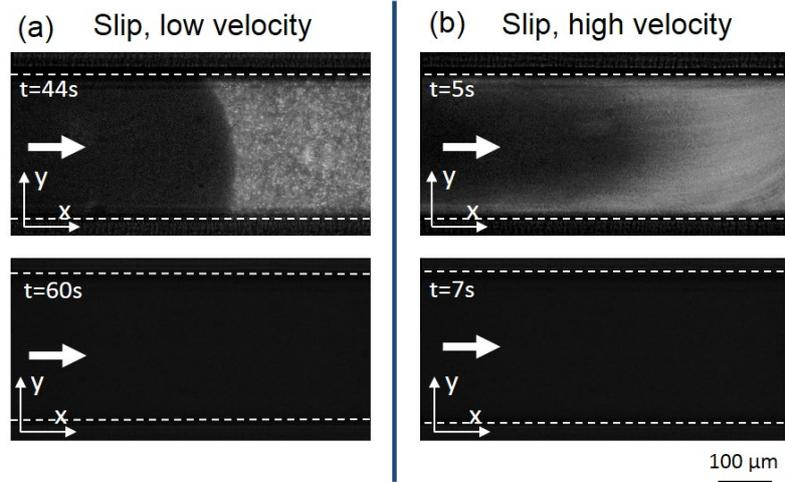
**Figure 5.14** – Stages of the displacement in a square channel of a microgel 2.2% by a microgel 1.6% with slip at 0.3 bar (left panel) and at 2.5 bar (right panel) at different times. The reference for the time scale corresponds to the beginning of the experiment.
