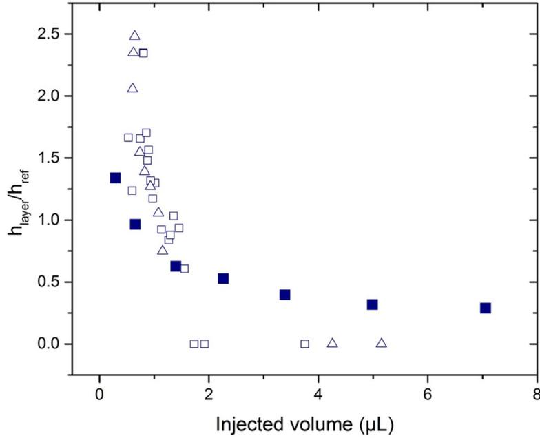
**Figure 6.14** – Thickness of the layer after breakthrough of the displacing fluid scaled by its thickness before breakthrough as a function of the injected volume in case of the displacement of a microgel 2.2% (square) and a microgel 3% (triangle) by a microgel 1.6% obtained in the experiments (open symbols) and in the three-dimensional simulations (full symbols) at a velocity of  $5 \text{ mm s}^{-1}$ .
