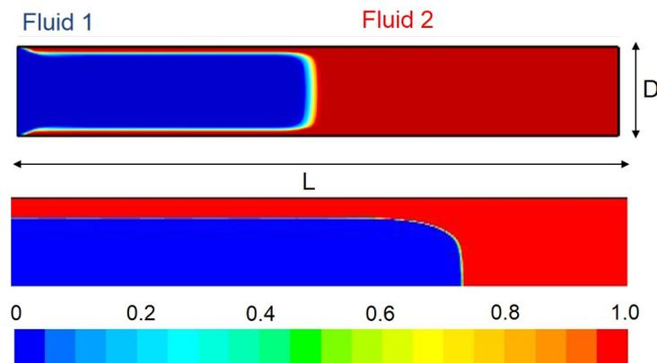
**Figure 6.11** – Volume fraction of fluid 2 for the displacement of two Bingham fluids:  $Re = 0.1$ ,  $M = 0.1$  and  $B = 100$ . Top: result extracted from [187], bottom: our result with Fluent. In both cases a sharp interface is defined between the fluids.
