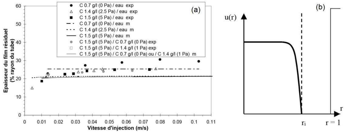
**Figure 5.4** – Reproduction from [58]. (a) Thickness of the layer scaled by the tube radius as a function of the injection velocity. (b) Velocity profile of the fluids as a function of the radial component  $r$ .  $r_i$  is the position of the interface between the fluids. The layer is fully static.
