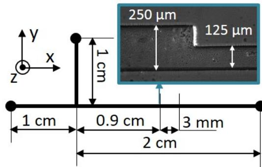
**Figure 5.18** – Geometry of the restriction channel.
