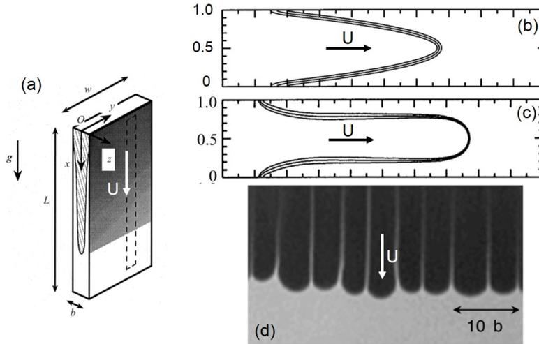
**Figure 5.3** – (a) Sketch of the finger across the gap of the Hele-Shaw cell for miscible displacements, reproduction from [95]. (b) Concentration profiles during miscible displacements at high  $Pe$  and for viscosity ratio (c)  $M = 1$  and (d)  $M = 100$ , reproduction from [155]. (d) Picture of the 3D instability observed by Lajeunesse *et al.* [94].
