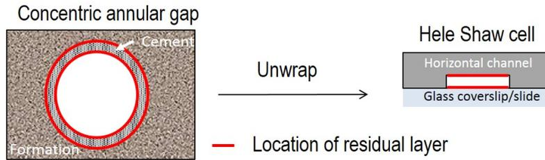
**Figure 5.6** – From annular gap to Hele-Shaw cell.
