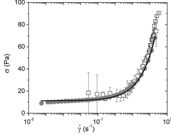
**Figure 4.10** – Shear stress versus shear rate for  $C = 0.016$  g/g: closed gray circles, macroscopic measurements; open black squares, data extracted from the velocity profiles shown in figures 4.7 (g)-(h); and solid line, best fit to the Herschel-Bulkley equation ( $\sigma_y = 11.2$  Pa,  $n = 0.5$ , and  $k = 4.1$  Pa s $^{1/2}$ ).
