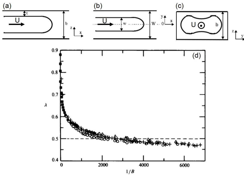
**Figure 5.2** – (a) Side view, (b) top view and (c) front view of the propagation of a single finger in a Hele-Shaw cell, reproduction from [104].  $t$  is the thickness of the wetting film left by the finger in the gap direction. (d) Effect of the wetting film: at high velocity, the relative width of the finger  $\lambda$  as a function of the dimensionless number  $1/B$ .  $\lambda$  goes below the limit 0.5 found by Saffman and Taylor [159]. Reproduction from [173].
