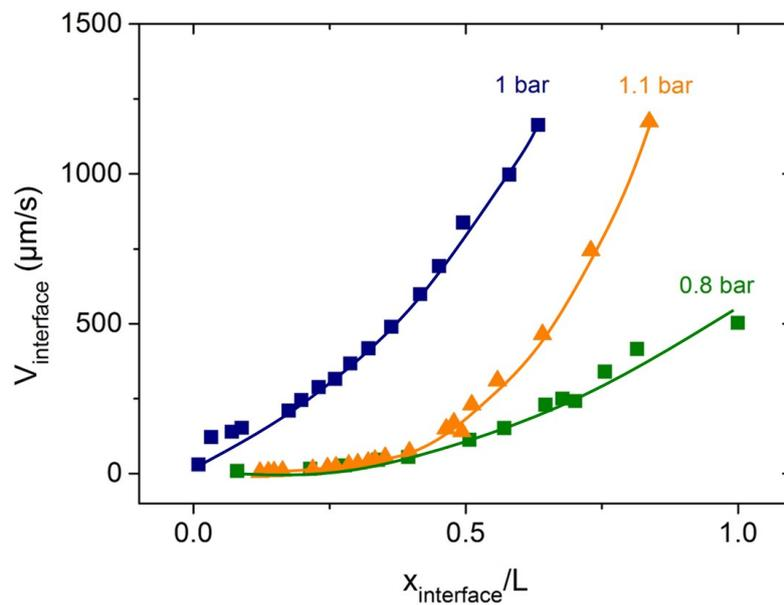
**Figure 5.15** – Representation of the velocity of the interface as a function of its position along the  $x$ -axis scaled by the channel length  $L$ , in the case of the displacement of a microgel 2.2% (square) and a microgel 3% (triangle) at several imposed pressure drop: 0.8 bar (green), 1 bar (dark blue), 1.1 bar (orange). The solid lines are guides for the eyes.
