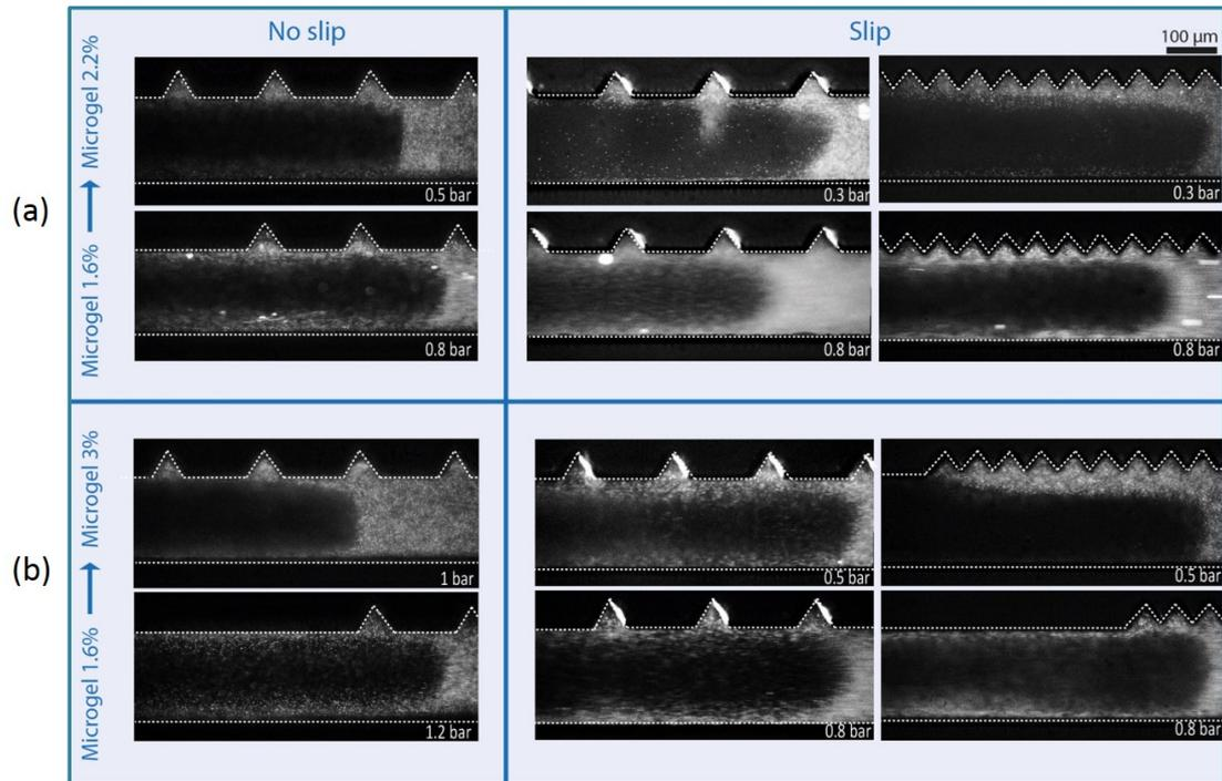
**Figure 5.24** – Displacement of a microgel 2.2% (a) and 3% (b) by a microgel 1.6% in the geometry of type A and B with slip and no slip at various constant pressure drops and at a time such that the interface passes along the corrugations. In the slip regime, important differences are observed between the geometries of types A and B during the advancement of the interface along the corrugations.
