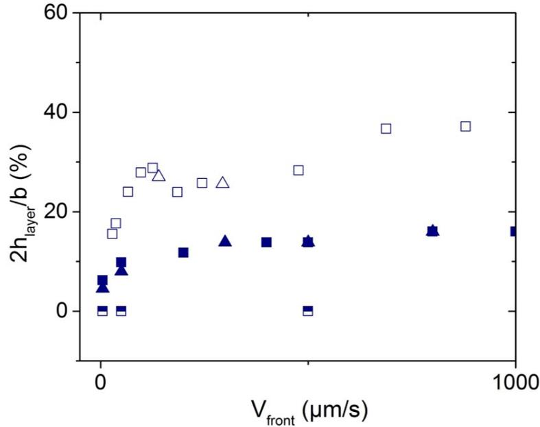
**Figure 6.13** – Thickness of the layer scaled by the width of the channel as a function of the front velocity in case of the displacement of a microgel 2.2% (square) and a microgel 3% (triangle) by a microgel 1.6% obtained in the experiments (open symbols) and in the two-dimensional simulations (full symbols).
