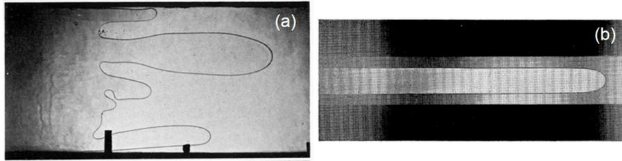
**Figure 5.1** – Reproduction from [159]. Top view of the displacement of immiscible fluid in a Hele-Shaw cell. (a) A finger gets ahead of its neighbour. (b) A single finger of water penetrating oil, the width of the finger is equal to the half of the channel width.
