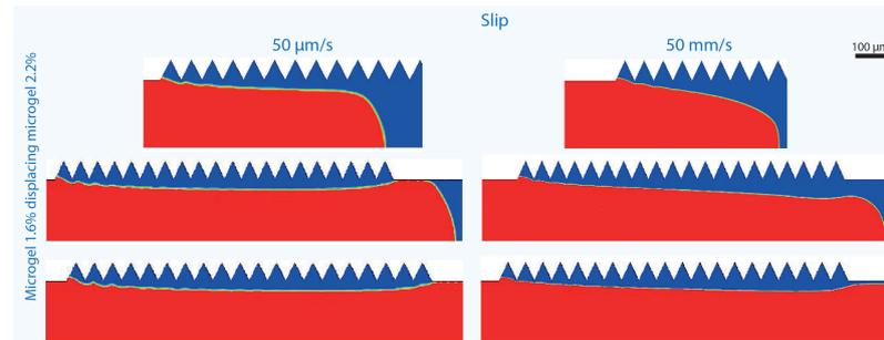
**Figure 6.20** – Shape of the interface near the corrugations obtained for the simulations of the displacements of a microgel 2.2% by a microgel 1.6% in the geometry B with slip at  $50 \mu\text{m s}^{-1}$  (left) and  $50 \text{mm s}^{-1}$  (right). The displacement is shown at increasing time steps from top to bottom.
