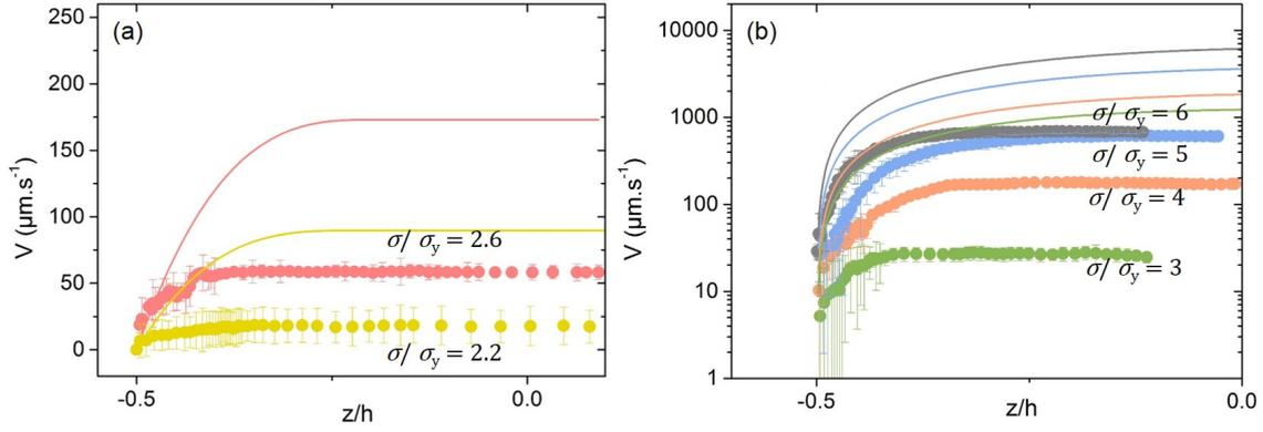
**Figure 5.8** – Half velocity profiles  $V$  of a microgel 1.6% flowing in (a) a Hele-Shaw cell with  $h = 80 \mu\text{m}$  and in (b) a square channel with  $b = 250 \mu\text{m}$  for various reduced stress  $\sigma/\sigma_y = 6$  (gray), 5 (blue), 4 (red), 3 (green), 2.6 (pink), 2.2 (yellow) with PEI treated walls. There is no slip in the channels. Solid lines are the theoretical Herschel-Bulkley velocity profiles.
