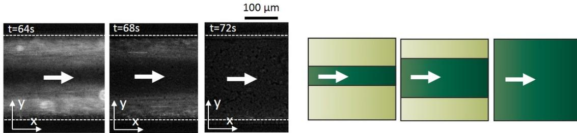
**Figure 5.13** – Evolution of the film with time for the displacement experiment in a square channel with a microgel 1.6% displacing a microgel 2.2% at a pressure drop of 0.5 bar with no slip at the walls. From left to right: the film is progressively removed from the channel. The reference for the time scale corresponds to the beginning of the experiment.
