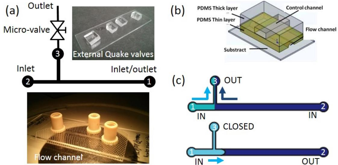
**Figure 3.7** – Experimental set-up for the study of fluid displacements. (a) Scheme of the experimental set-up, picture of the glass flow channel made with NOA. (b) In the Quake valve, the control channel is above the flow channel and can seal it when it is being pressurized. Reproduction from [166]. (c) Fluids sequence to initialize the displacement experiment.
