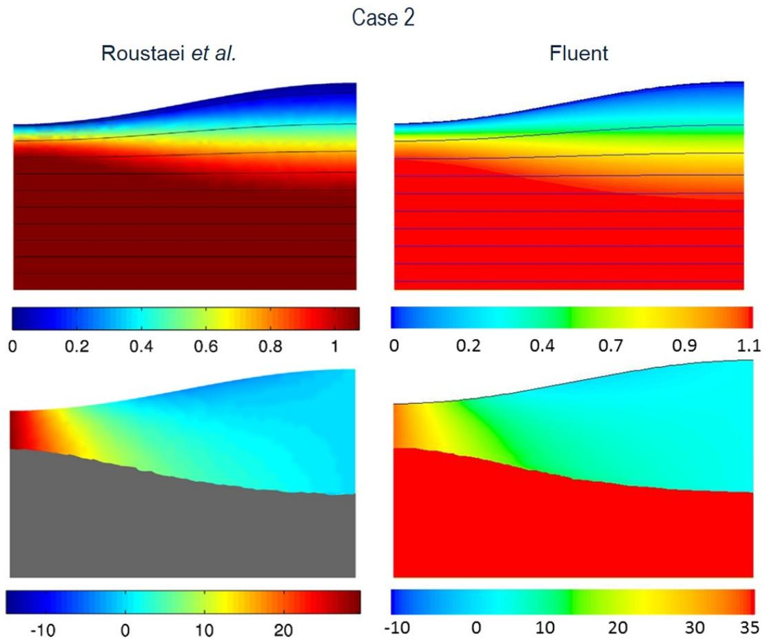
**Figure 6.8** – Comparison of case 2:  $B = 10$ ;  $h = 0.25$  and  $\delta = 0.25$  between the results of Roustaei *et al.* (left panel) and our results with Fluent (right panel). Top: Velocity field (m/s). Bottom: Pressure field (Pa).
