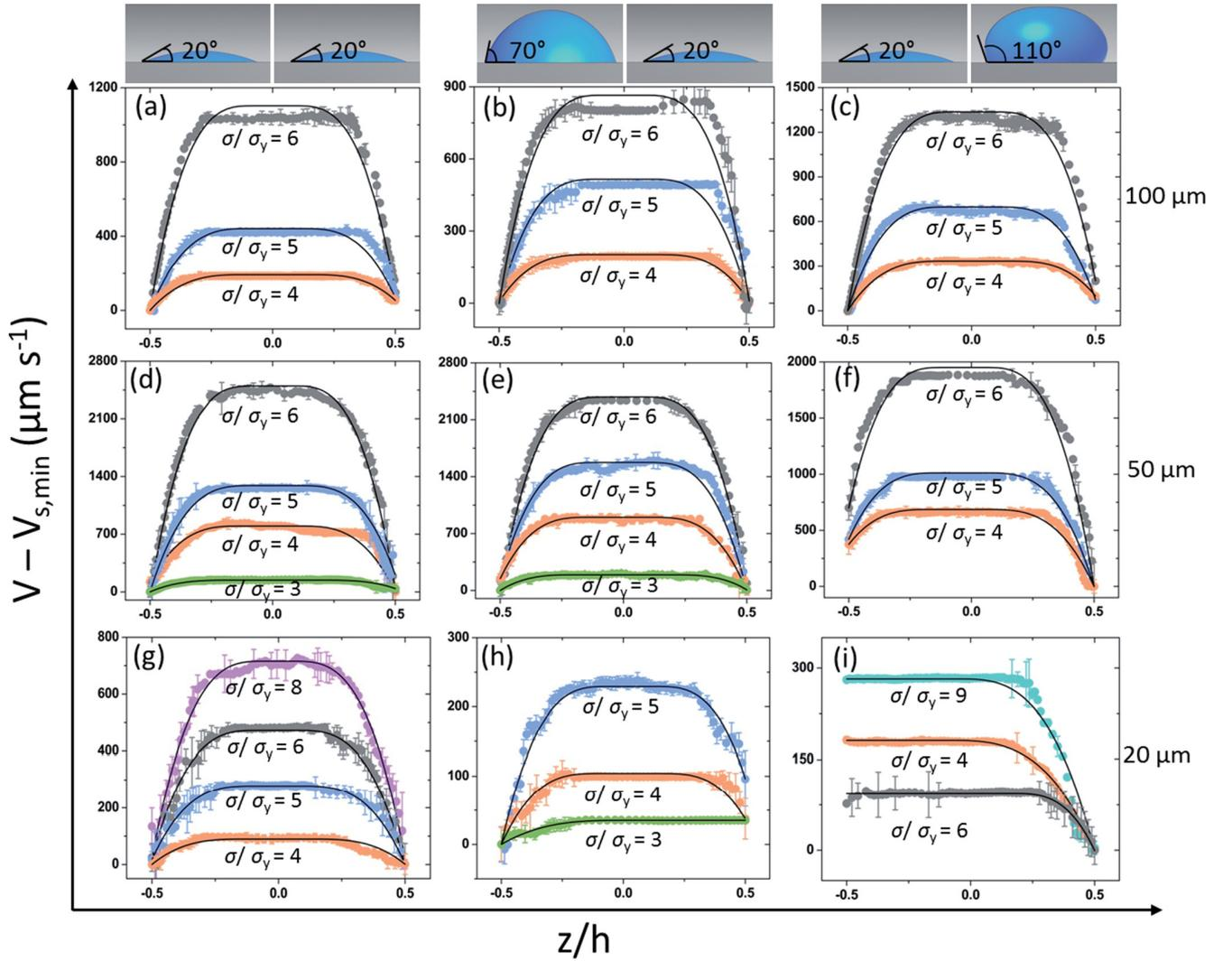
FIG. 2. (Color online) Velocity profiles  $V$  corrected from the slip velocity  $V_{s,\min}$  for various heights, boundary conditions, and reduced stress  $\sigma/\sigma_y = 9$  (dark cyan), 8 (purple), 6 (gray), 5 (blue), 4 (red), and 3 (green). The solid lines are the best fits to the theoretical expression of the velocity profiles calculated in the asymmetric Herschel-Bulkley flow model Eq. (3).
