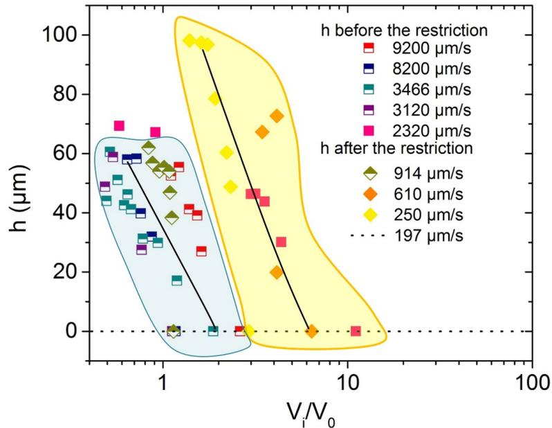
**Figure 5.21** – The evolution of the thickness of the layer as a function of the number of injected channels volume  $V_i/V_0$  for slip (half full symbols) and no slip (full symbols) boundary conditions. The solid lines are guides for the eyes.
