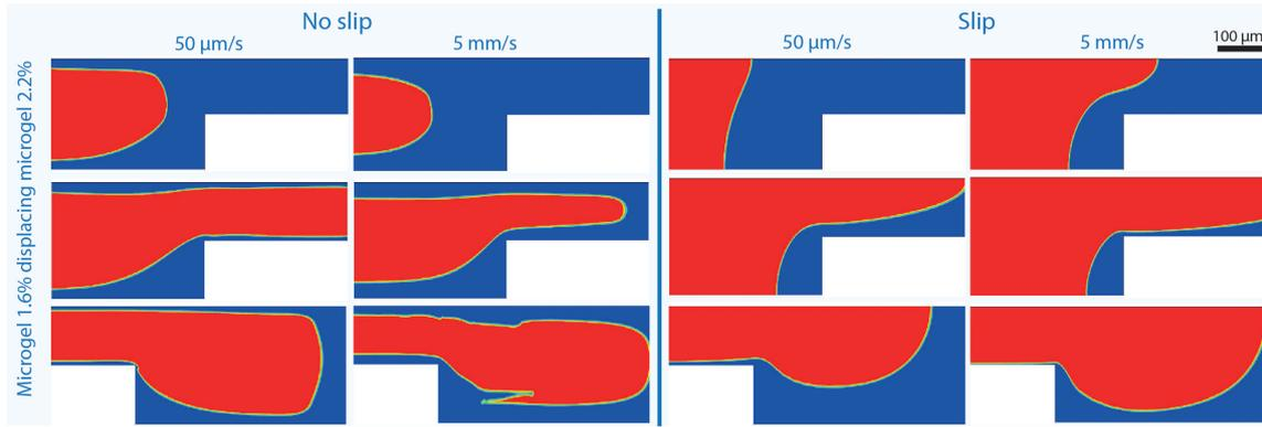
**Figure 6.17** – Shape of the interface for a displacement of a microgel 2.2% by a microgel 1.6% with no slip (left panel) and slip (right panel) at the walls from before (top line) to after the restriction (bottom line) and as a function of the imposed velocity:  $50 \mu\text{m s}^{-1}$  and  $5 \text{mm s}^{-1}$  (from left to right).
