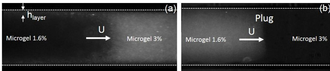
**Figure 5.29** – Comparison of the shape of the interface between no slip (a) and slip (b) during the displacement of a microgel 3% by a microgel 1.6% at 0.5 bar. No film is left at the walls in the case of slippage.
