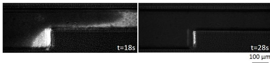
**Figure 5.20** – Displacements of a microgel 2.2% by a microgel 1.6% in restriction channels with slip. The restriction retains some of the displaced fluid but only for a short time. The reference for the time scale corresponds to the beginning of the experiment.
