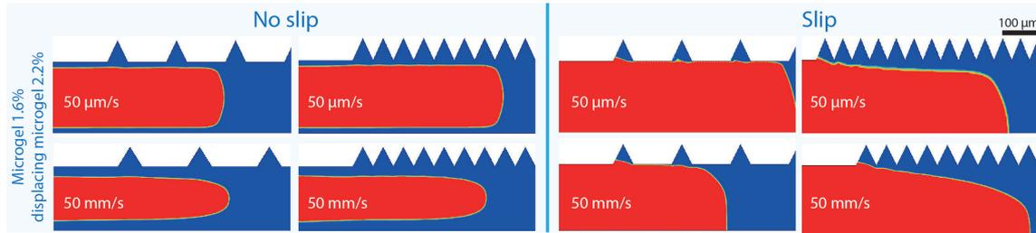
**Figure 6.19** – Shape of the interface near the corrugations obtained for the simulations of the displacements of a microgel 2.2% by a microgel 1.6% in the geometries A and B with no slip (left panel) and slip (right panel) at velocities of  $50 \mu\text{m s}^{-1}$  (top line) and  $50 \text{mm s}^{-1}$  (bottom line).
