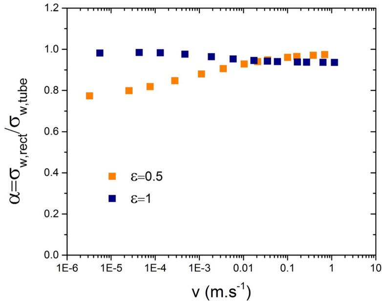
**Figure D.2** – Ratio of the wall shear stress obtained in a rectangular channel to the wall shear stress in a tube of equivalent hydraulic diameter as a function of the mean velocity of a Herschel-Bulkley fluid. The aspect ratio of the rectangular channels are  $\epsilon = 1$  (blue) (it is a square channel) and  $\epsilon = 0.5$  (orange) which corresponds to the restriction geometry of chapter 5.
