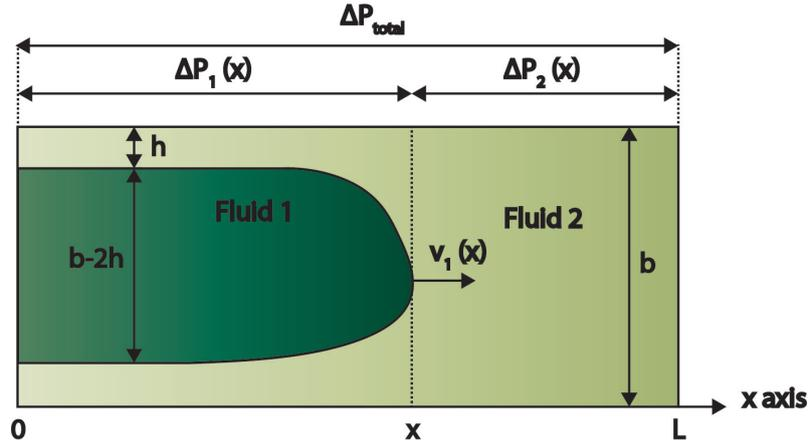
**Figure D.1** – As the interface advances in the channel under a constant pressure drop applied  $\Delta P_{total}$ , the pressure drop over fluid 1  $\Delta P_1(x)$  increases and the pressure drop over fluid 2  $\Delta P_2(L-x)$  decreases and the velocity of the interface  $v_1$  increases.
