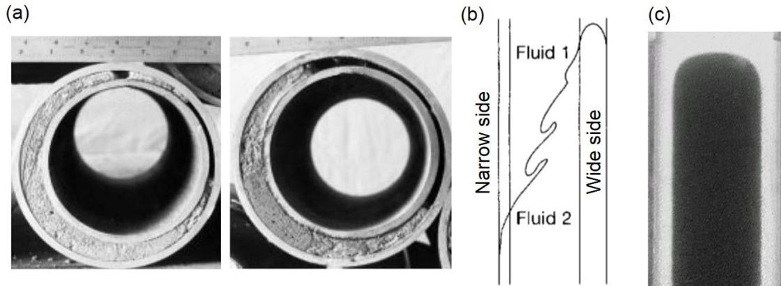
**Figure 1.4** – (a) Unsuccessful mud-displacement experiment in an eccentric annulus: the narrow gap is not filled with cement, reproduction from [89]. (b) Gravitational instabilities that promote an azimuthal flow from the wide side to the narrow side of the annulus, reproduction from [177]. (c) Viscous fingering during the iso-density displacement of a Herschel-Bulkley fluid by another one with a lower yield stress, reproduction from [58].
