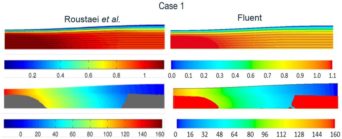
**Figure 6.7** – Comparison of case 1:  $B = 10$ ;  $h = 0.25$  and  $\delta = 0.05$  between the results of Roustaei *et al.* (left panel) and our results with Fluent (right panel). Top: Velocity field (m/s). Bottom: Pressure field (Pa).
