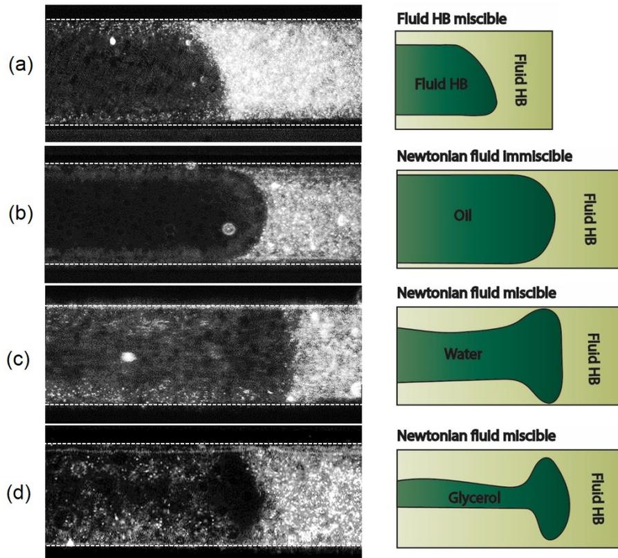
**Figure 5.11** – Interface shape between a microgel 2.2% displaced by (from top to bottom): (a) a less viscous microgel 1.6%, (b) immiscible oil  $\eta = 25 \cdot 10^{-3}$  Pa s, (c) miscible water  $\eta = 10^{-3}$  Pa s and (d) miscible glycerol  $\eta = 25 \cdot 10^{-3}$  Pa s.
