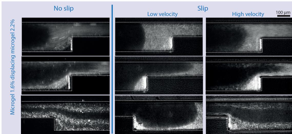
**Figure 5.19** – Displacements of a microgel 2.2% by a microgel 1.6% in restriction channels with slip and no slip. With slip, the displacements at low velocities and high velocities exhibit different behaviours, namely a film forms in the latter case.
