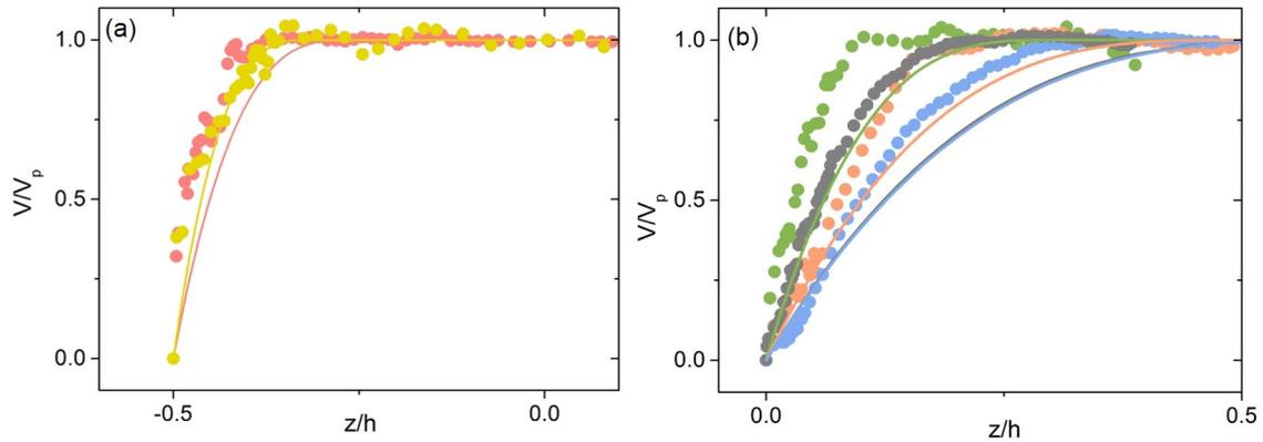
**Figure 5.9** – Velocity profiles scaled by the plateau velocity of a microgel concentrations 0.016 g/g flowing in a (a) Hele-Shaw channel of height  $80 \mu\text{m}$  and in a (b) square channel with no slip at various reduced shear stress:  $\sigma/\sigma_y = 6$  (gray), 5 (blue), 4 (red), 3 (green), 2.6 (pink), 2.2 (yellow). The solid lines are the theoretical shapes of the velocity profiles whose pressure gradients have been adjusted to match the experimental central plug velocities.
