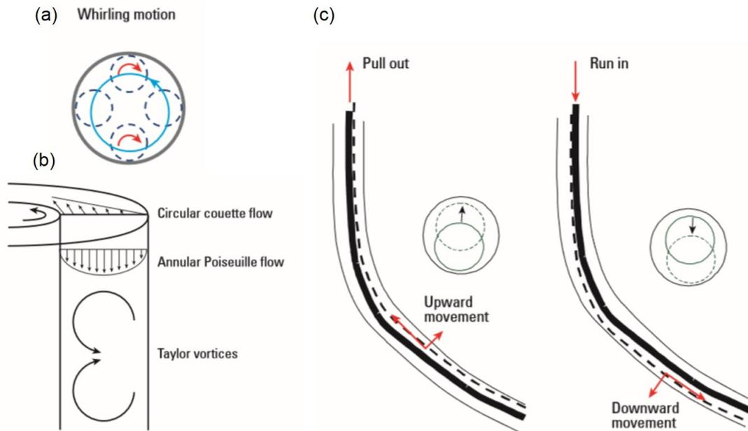
**Figure 1.8** – Reproduction from [133]. (a) Whirling movement of the casing induced by its rotation at high speeds. (b) Taylor vortices in the annular gap created by the combination of axial and azimuthal flows during casing rotation. (c) Axial and lateral movements of the casing during reciprocation.
