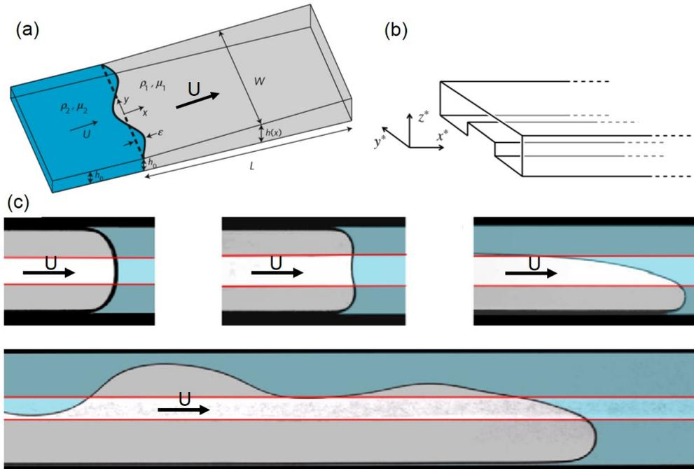
**Figure 5.5** – (a) Displacement in a diverging-converging gap Hele-Shaw cell [1]. (b) Schematic view of a Hele-Shaw cell with an obstruction in the gap direction [178]. (c) Examples of the fingering patterns obtained in the obstructed Hele-Shaw cell (b) [178].
