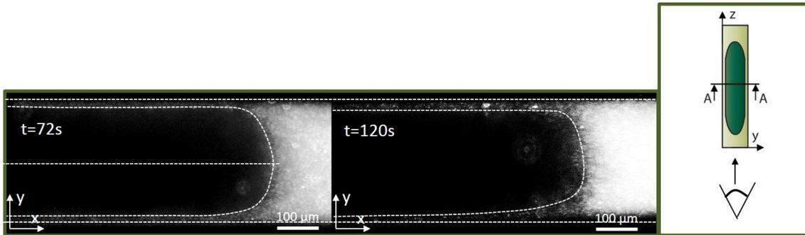
**Figure 5.27** – Propagation of the interface in the moving frame of reference of the finger in a canyon channel without slip when a microgel 1.6% is displacing a microgel 2.2% at a constant pressure drop of 0.5 bar. A film is formed behind the interface. The reference for the time scale corresponds to the beginning of the experiment.
