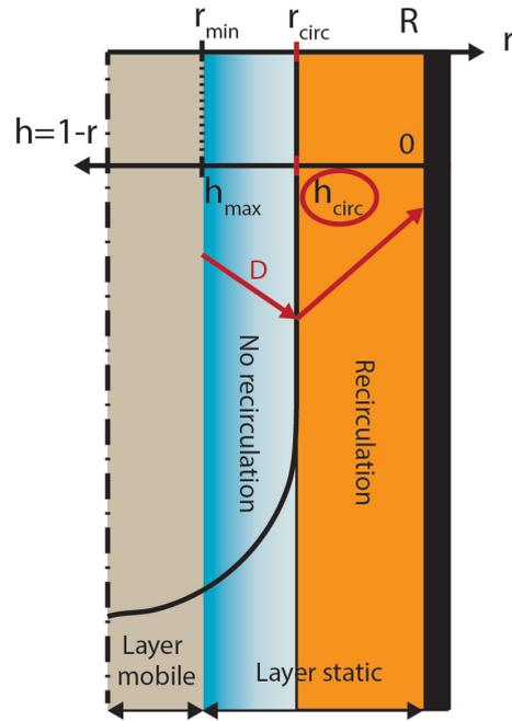
**Figure B.2** – Schematic representation of the front of the finger and of the limits for the layer thickness:  $h_{max}$  is the maximal thickness the layer can reach while staying static,  $h_{circ}$  sets the onset of the recirculation in fluid 2 at the front of the finger.
