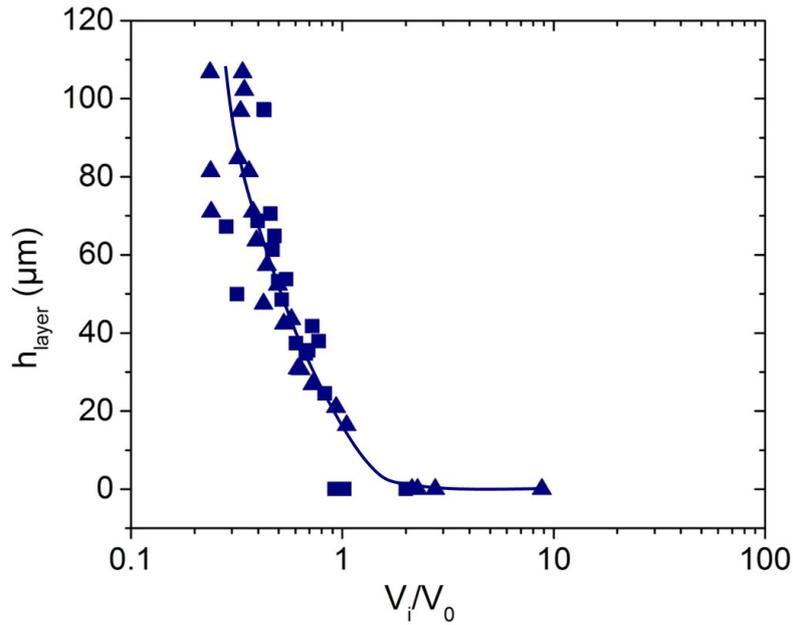
**Figure 5.17** – Thickness of the film left at the walls as a function of the number of injected channels volume  $V_i/V_0$  for the displacement of a microgel 2.2% (square) and a microgel 3% (triangle) by a microgel 1.6% at different pressure drops (0.8 to 1.4 bar). The solid line is a guide for the eyes.
