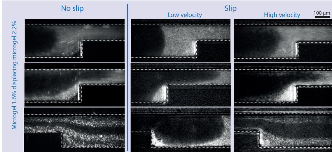
**Figure 6.16** – Displacement of a microgel 2.2% by a microgel 1.6% in a channel with a restriction with slip and no slip boundary conditions. With slip boundary conditions, the displacements at low velocity and high velocity exhibit different behaviours, namely a film forms in the latter case.
