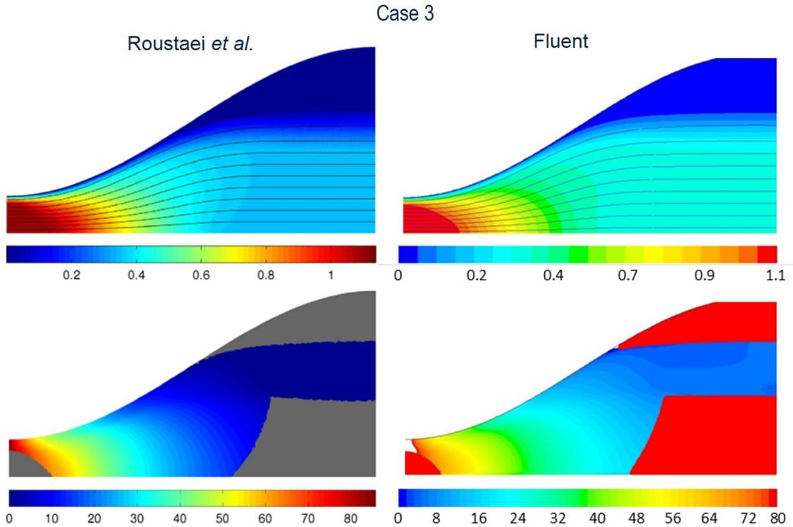
**Figure 6.9** – Comparison of case 3:  $B = 10$ ;  $h = 4$  and  $\delta = 0.05$  between the results of Roustaei *et al.* (left panel) and our results with Fluent (right panel). Top: Velocity field (m/s). Bottom: Pressure field (Pa).
