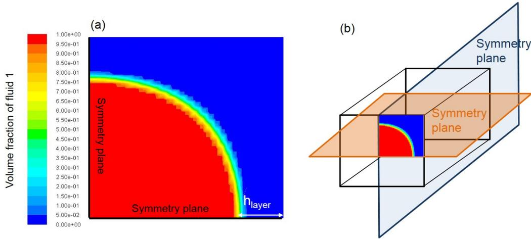
**Figure 6.15** – (a) Cross section of a three-dimensional square channel with the measure of the thickness of the layer. (b) Position of the symmetry planes. The simulation is performed only on a quarter of the square channel.
