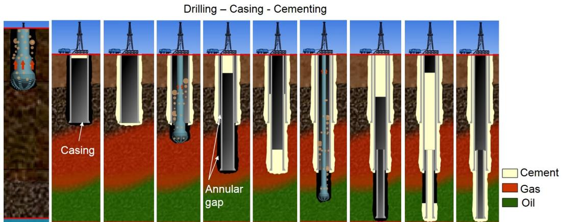
**Figure 1.1** – From left to right: repetition of the drilling, casing and cementing stages for the construction of a well.
