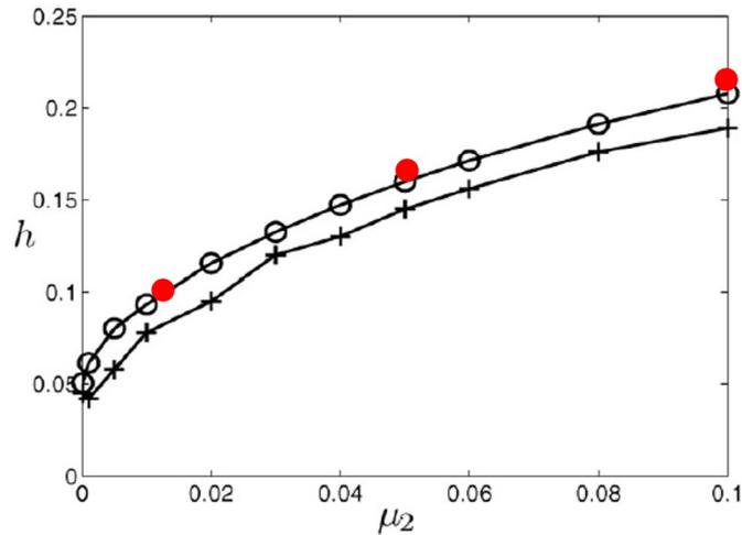
**Figure 6.12** – Thickness of the layer left at the walls during the displacement of two Bingham fluids for varying the viscosity of the displaced fluid  $\mu_2$  and with  $\mu_1 = 0.01$ ,  $\tau_{1,Y} = 0.2$  and  $\tau_{2,Y} = 0.5$ . (open circle) data from [187], (cross) data from [2], (red full circles) our results with Fluent.
