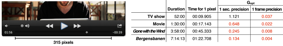
FIGURE 4.4: Optimal CD gain values ( G_{opt} ) for one-second and one-frame resolution navigation in videos of various durations using the slider interface of QuickTime Player. Red G_{opt} values are outside the CD gain range of the typical transfer functions of modern operating systems, and require pointing transfer function adaptation.
